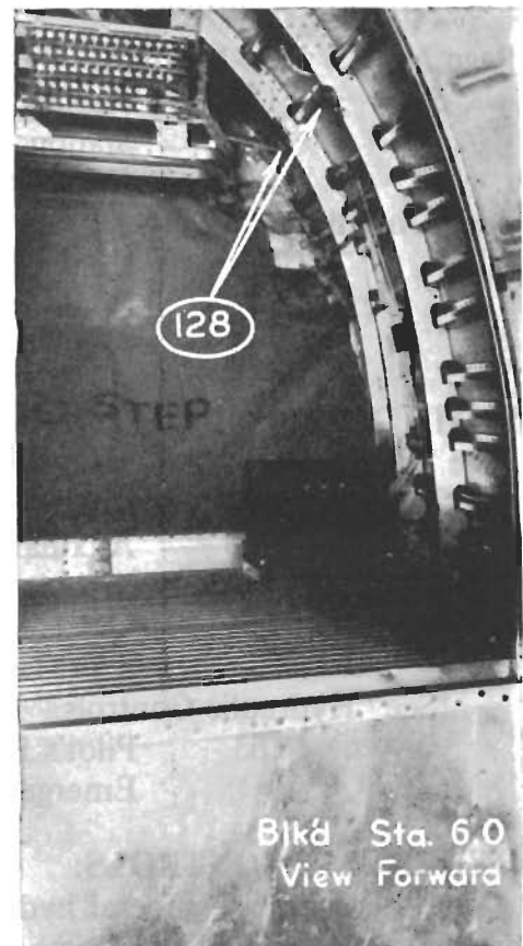
128. Starter Crank Stowage
