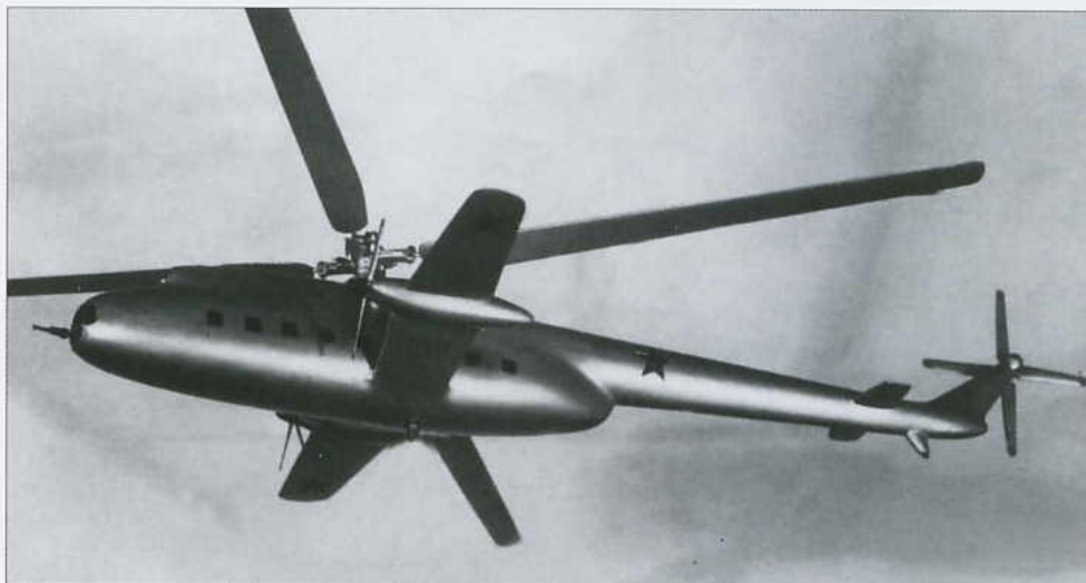
A model of the VM-6 project as originally envisaged, showing the low-set wings carrying turboprops with tractor propellers. Note also the almost hemispherical nose with a machine-gun mount.
