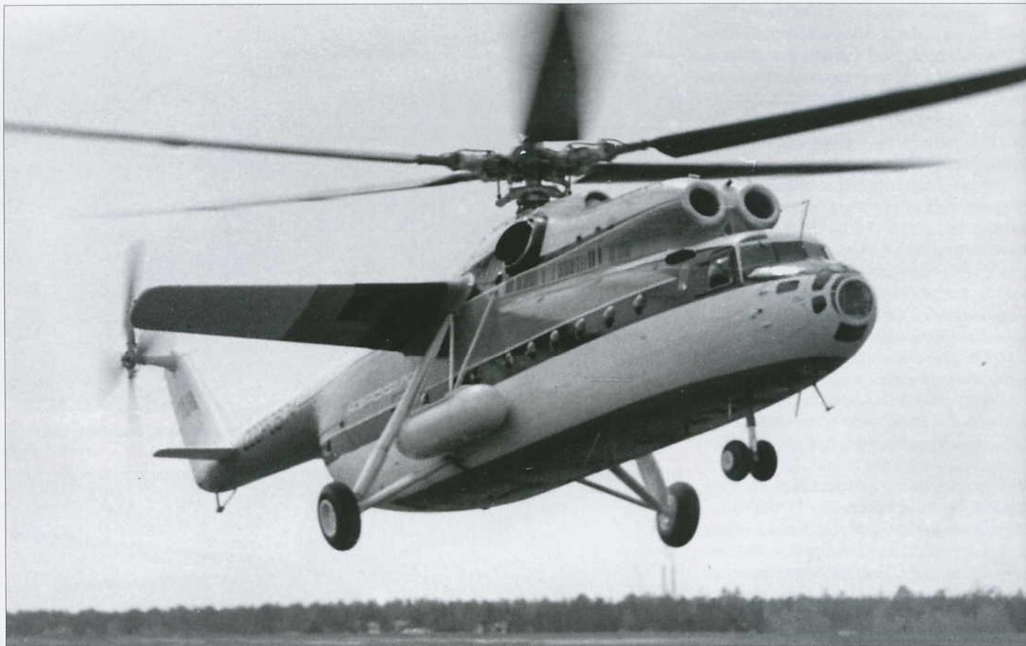
Above: Smartly painted CCCP-06174 (c/n 5682010V) was the prototype of the commercial version of the Mi-6. Note the dark-coloured heat shields on the wing leading edges protecting these from the hot exhaust; the inner wings were painted to disguise the exhaust soot stains as much as possible.
