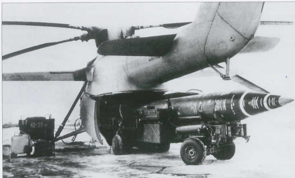
Above: The Mi-6RVK (c/n 2681110V) disgorges a towed mobile launcher with an R-17V intermediate-range ballistic missile.
