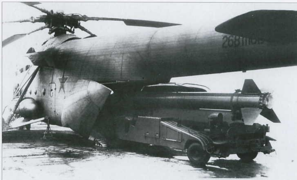
Above: A 9M21 Loona-MV theatre ballistic missile on a launcher is loaded into Mi-6RVK c/n 268110V.
