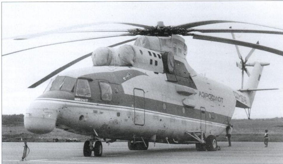
Above: CCCP-06146, the Mi-26NEF-M ASW helicopter, at Pushkin in 1992. The 'droopsnoot' radome housing a search radar is clearly visible, but the cutout for the dunking sonar in the ramp is not. Before...
