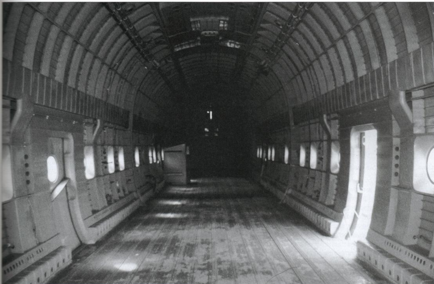
Above: The cargo cabin of the V-12, showing the rear pair of entry doors and the cabin heating air ducts running along the walls above the window level. Note the bottom of the cross-shaft's intermediate gearbox casing at the top of the picture.
