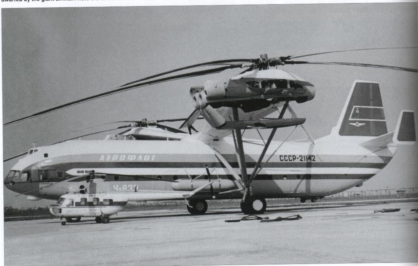
Another view of the Mi-2 and the V-12. The latter's huge engine cowlings give virtually unrestricted access to the engines and the main gearboxes. Note the small twin-wheel tail bumpers and the supports on which the cargo ramp rests.
