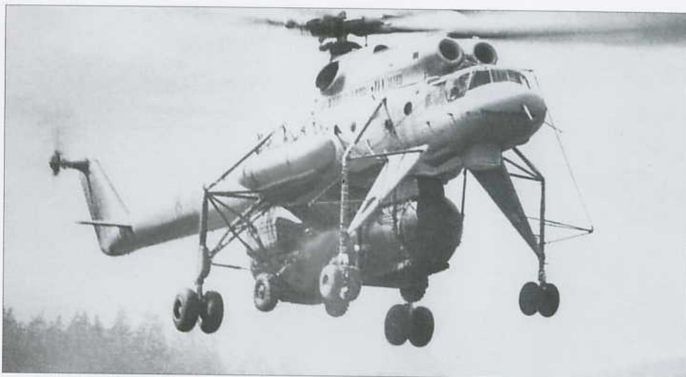
Above: A Mi-10RVK missile carrier with the 9P116 wheeled launcher attached. Note the fat low-pressure tyres on all four landing gear units.
