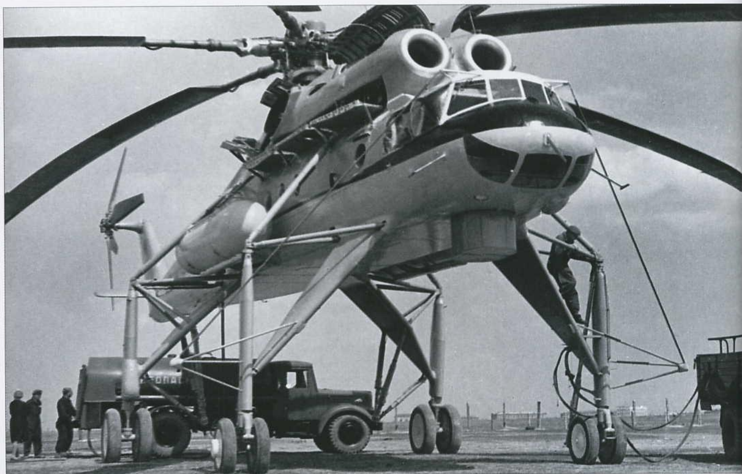
Mi-10 CCCP-04102 undergoes routine maintenance with the engine and main gearbox cowling panels open for inspection. A ground power unit on a ZIS-150 chassis is parked alongside, while a fuel bowser based on a MAZ-200 diesel lorry tops up the helicopter's fuel tanks. The nosewheels are of a new type.
