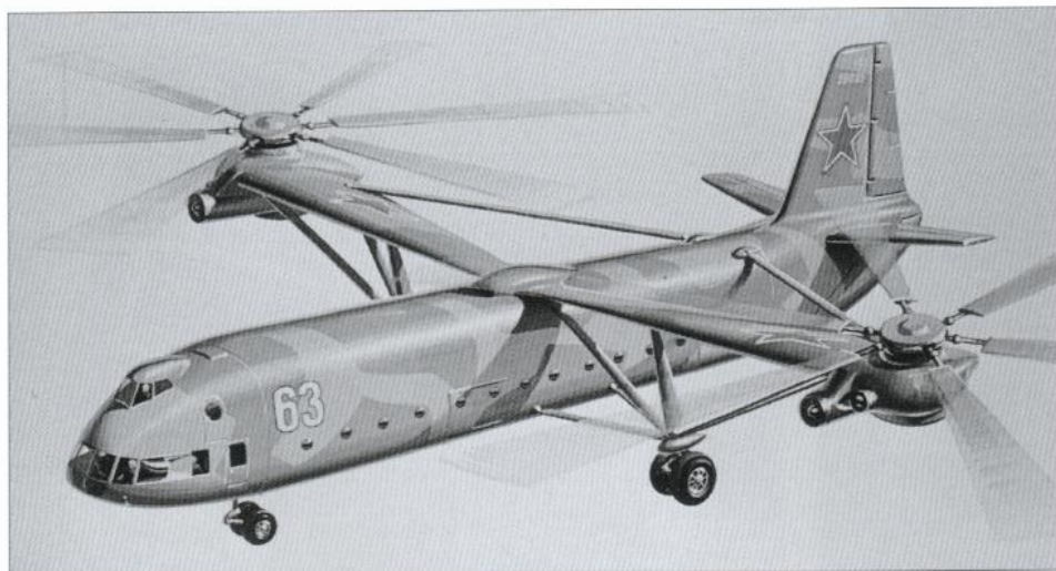
Above: An artist's impression of the V-16 – basically a V-12 with new engines featuring large-diameter low-speed free turbines driving six-blade rotors.
