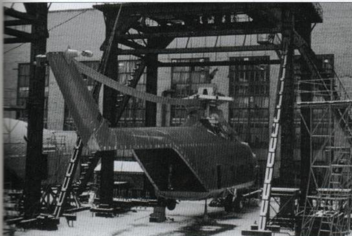
Left and right: The static test airframe of the Mi-26 suspended under a gantry-type test rig which was used for testing the landing gear for crashworthiness.
