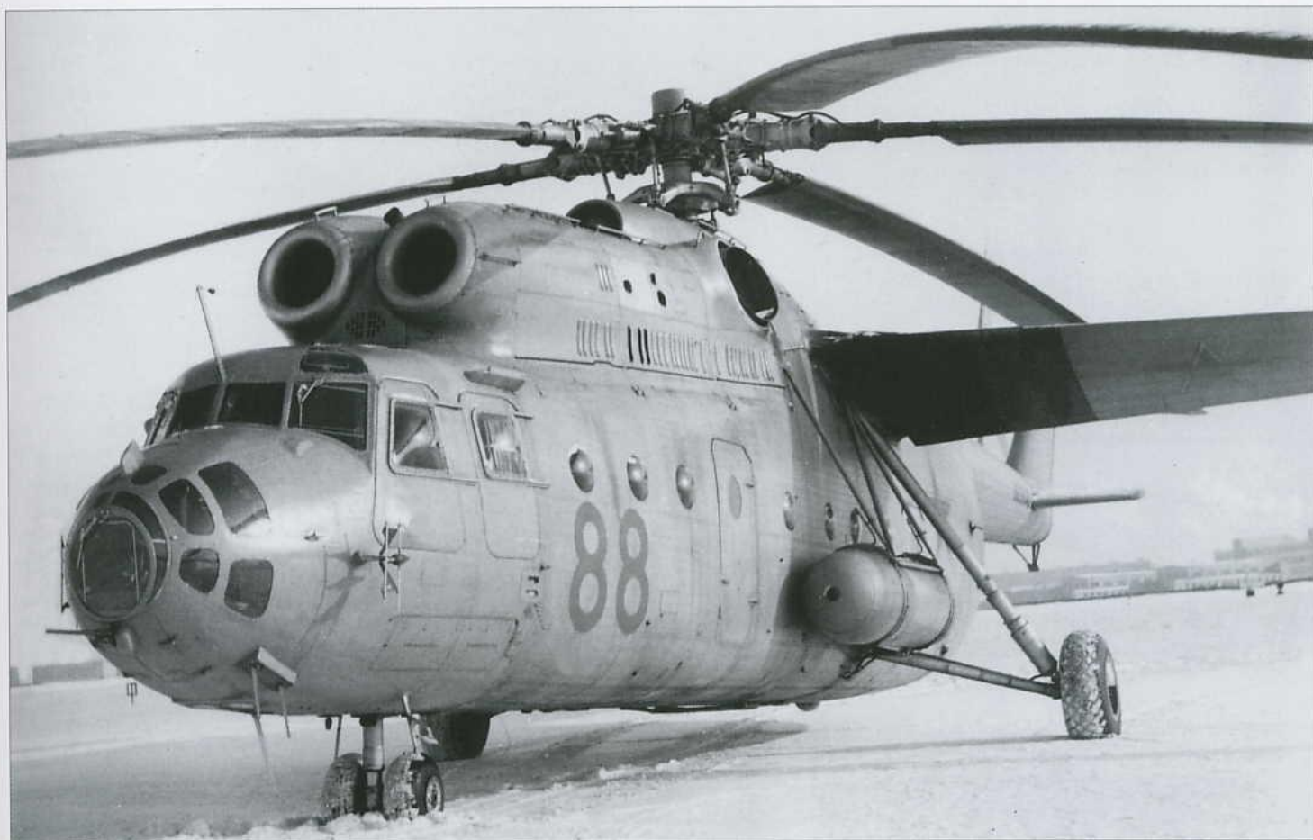
After checkout trials at GK NII VVS this Mi-6 coded '88 Red' was used for development work at LII in Zhukovskiy. Note the black 'anti-soot' bands on the wing roots.
