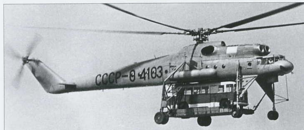
Above and below: Wearing the registration in unusually large digits, the third prototype (CCCP-04103, c/n 04103) carries a ZIL-158 bus. The windows in the latter's four-leaf doors are obscured for some reason.
