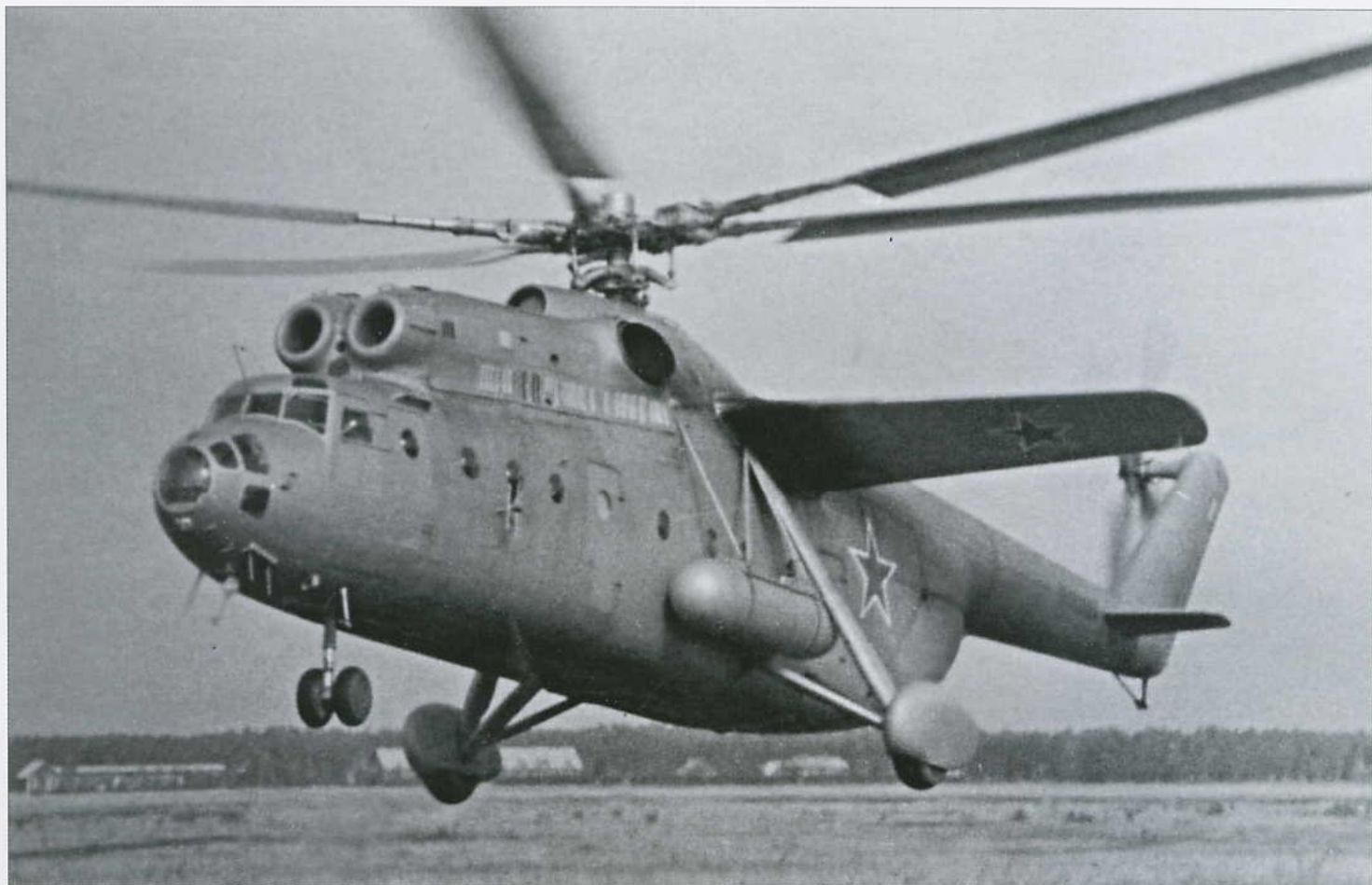
Above: An early-production Mi-6 fitted with external tanks and bristling with aerials (compare with the photo on page 4). Note the soot-blackened wing roots. Below: As this picture testifies, at least the first 120 Rostov-built Mi-6s (such as c/n 2681110V here) were delivered with mainwheel spats.
