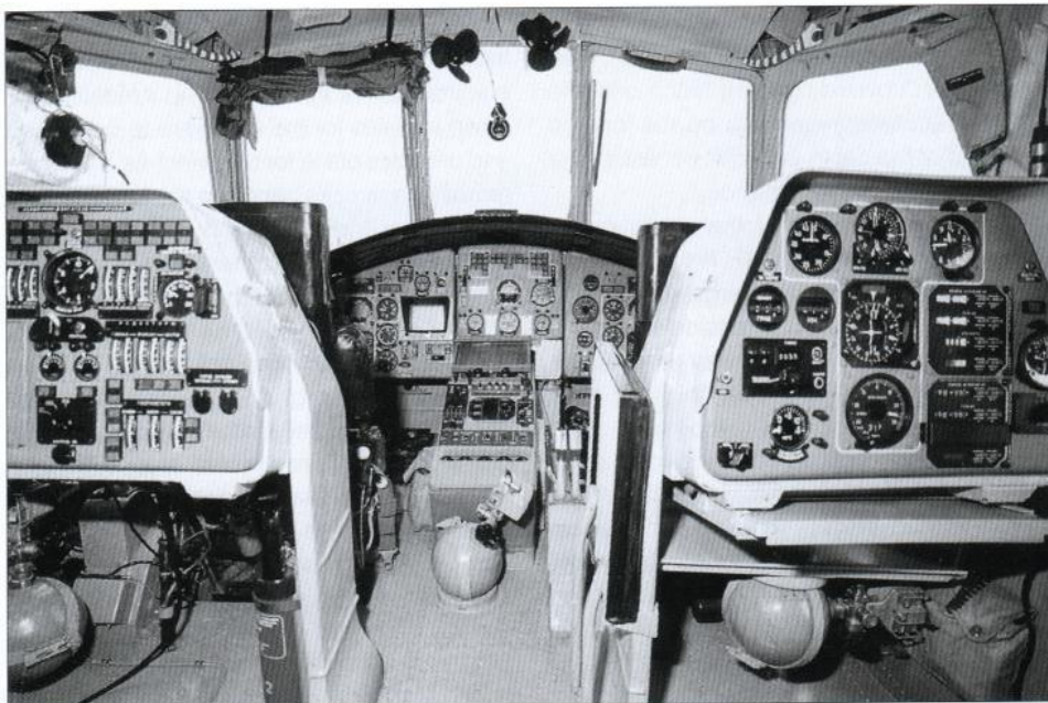
Above: The flightdeck of a standard Mi-26, with the flight engineer's station on the left and the navigator's station on the right behind the captain and the co-pilot respectively.
