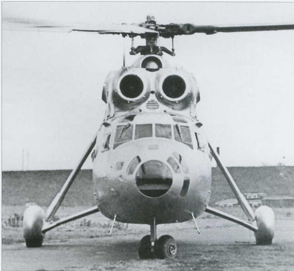
Above: This head-on shot of the prototype taxiing at Zakharkovo shows the asymmetric arrangement of the navigator's station glazing panels.
