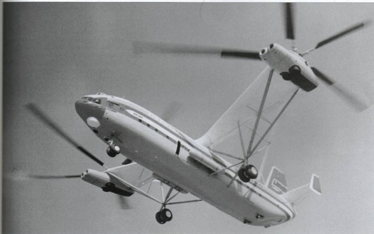
Another in-flight photo of the V-12, showing the complex wing support/undercarriage trusses. Note the partially open entry door.
