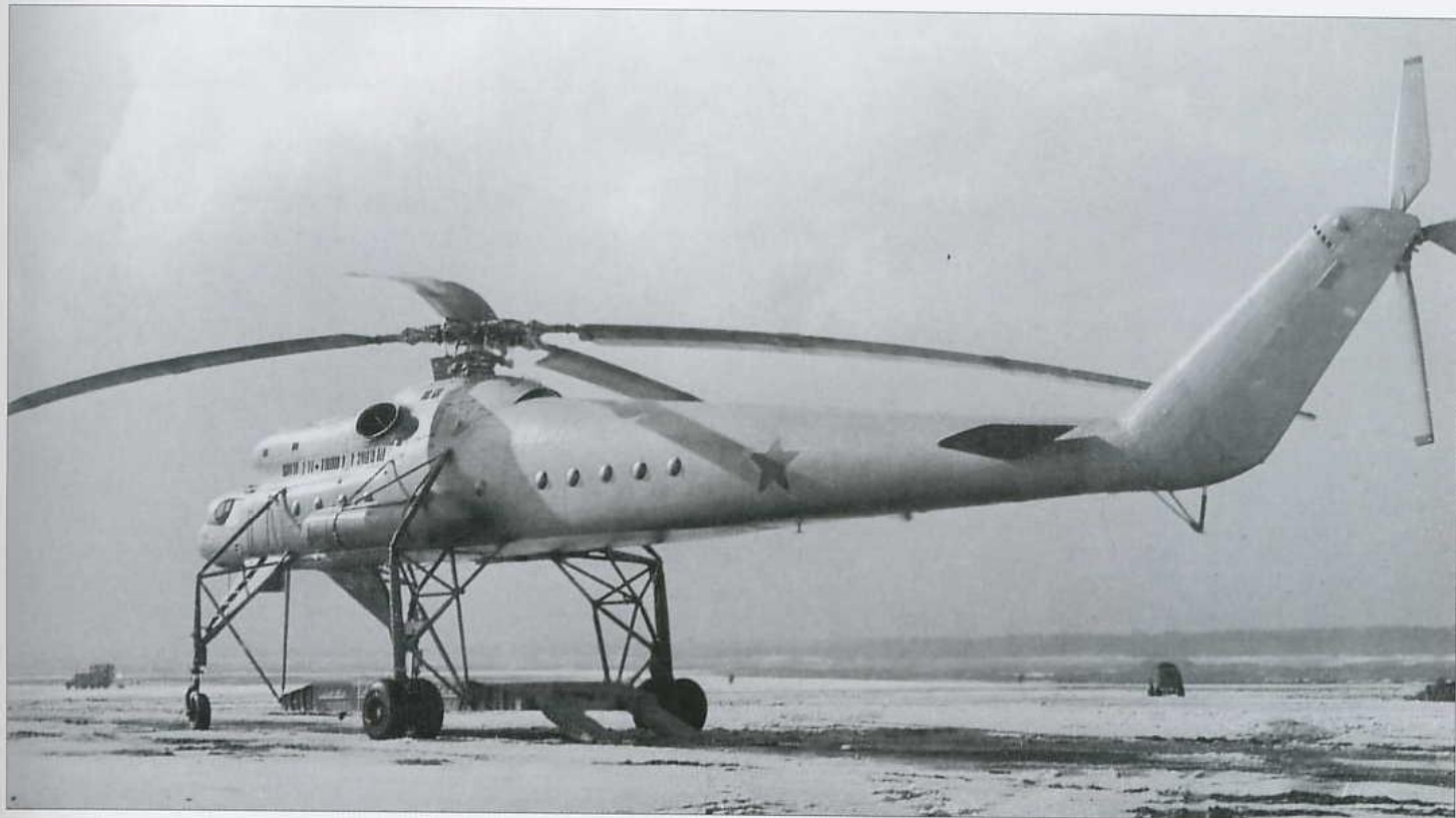
Above: The first prototype in an interim configuration with new main gear units featuring vertical struts and twin wheels. The nose units have been modified to incorporate boarding steps. The ramps used for loading vehicles onto the suspended platform are visible here, as are the bulged flightdeck windows.
