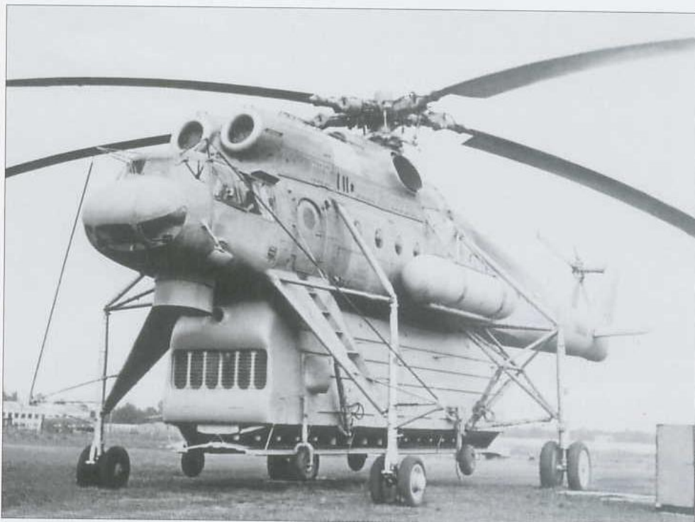
Above: The Mi-10P (alias Mi-10PP; c/n 7680502K?) with the huge ST-9000 Step' ECM pod under the fuselage. Note the forward-mounted radiator and the wheels for towing the pod.
