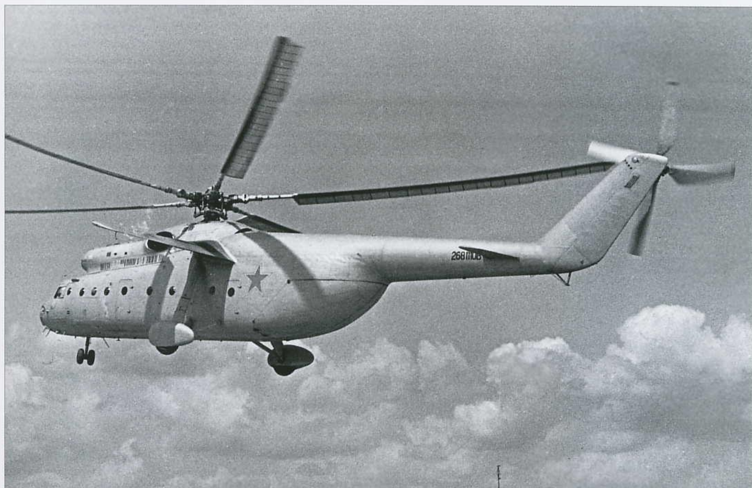
Above: An early-production Mi-6 fitted with external tanks and bristling with aerials (compare with the photo on page 4). Note the soot-blackened wing roots. Below: As this picture testifies, at least the first 120 Rostov-built Mi-6s (such as c/n 2681110V here) were delivered with mainwheel spats.
