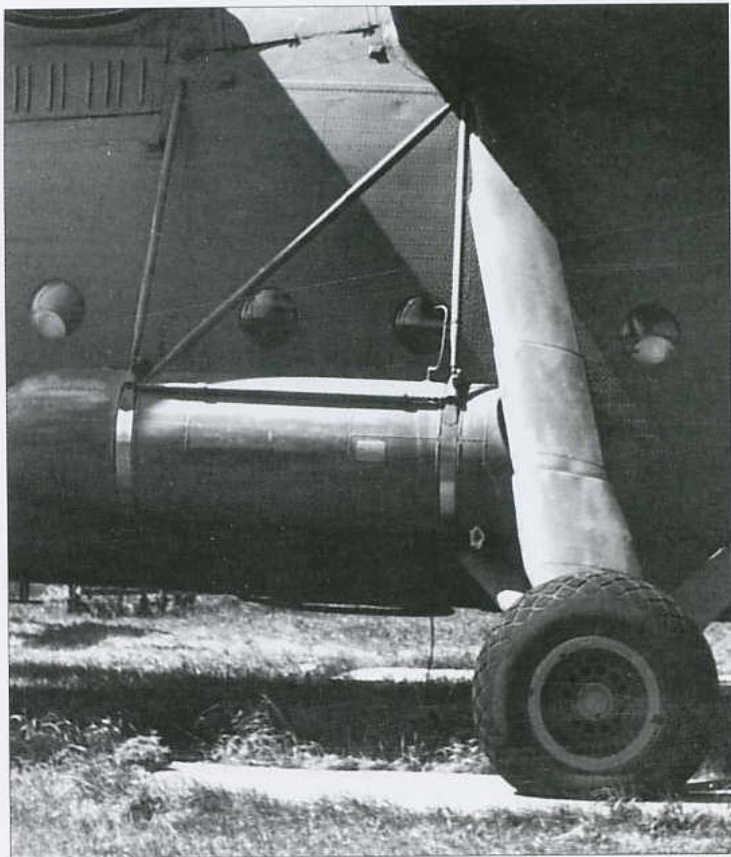
Left: The centre fuselage and the port external tank with its retaining straps and N-strut. Right: The starboard main landing gear unit with a faired shock strut.
