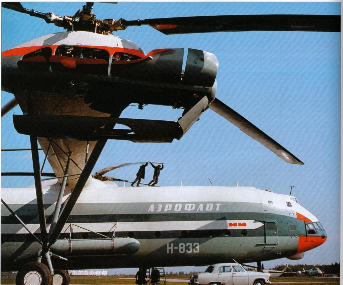
The V-12 sits with every engine cowling panel open for inspection as two technicians seemingly make a futile attempt to turn the rotors! The 1965-model GAZ-21R Volga sedan has probably brought members of the design staff to the hardstand. Note the Mi-6 and the Mi-8 parked beyond.
