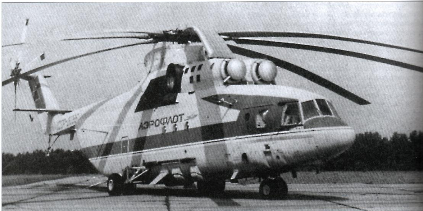
Above: CCCP-06098, one of the two Mi-27 airborne command posts, showing the ventral antenna farm and the closely-spaced raised windows.
