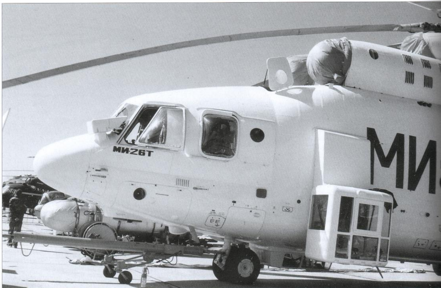
Above: Mi-26T RA-06089, seen here at the MAKS-97 airshow, featured two extra control cockpits (aft of the nose gear and in place of the port forward door) and an external TV display for 'flying crane' work.
