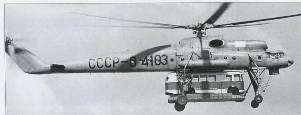
Above and below: Wearing the registration in unusually large digits, the third prototype (CCCP-04103, c/n 04103) carries a ZIL-158 bus. The windows in the latter's four-leaf doors are obscured for some reason.
