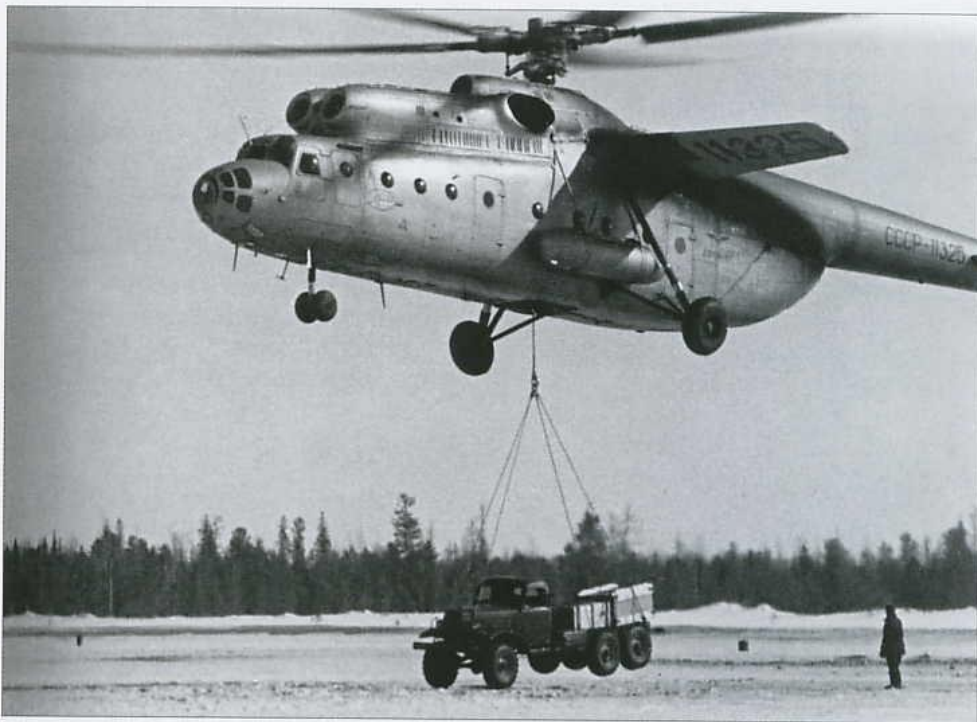
Mi-6 CCCP-11325 (c/n 3681406V) of the Moscow Agricultural Work & Commuter Air Traffic Directorate lifts a ZiL-157K 6 x 6 lorry on a sling.
