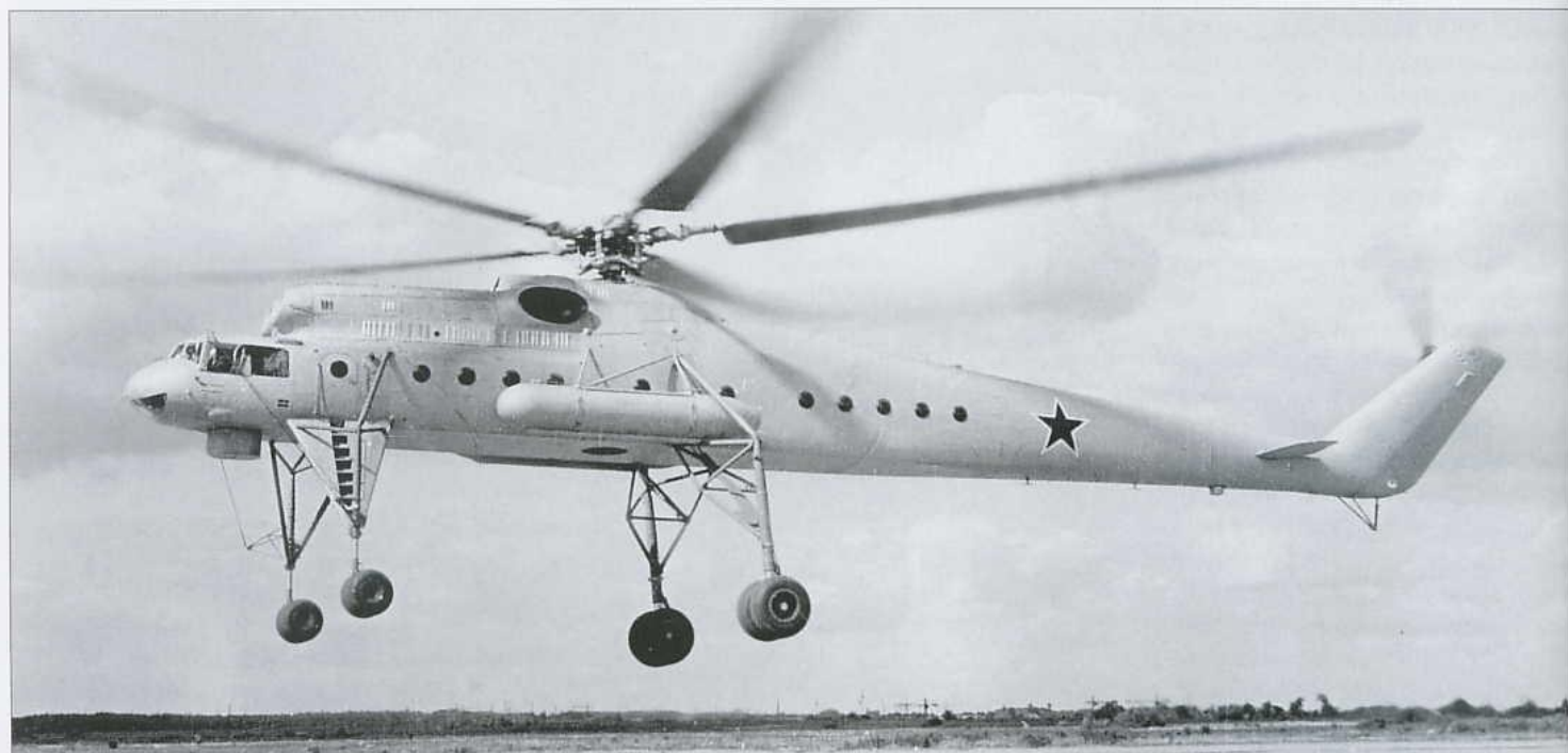
The first prototype Mi-10 lifts off in unloaded condition during trials, showing the ventral hatch for the cargo sling. The escape chute is retracted and its bottom closed by a jettisonable cover. Note how the rear ends of the external tanks fit in between the rods of the main gear trusses.
