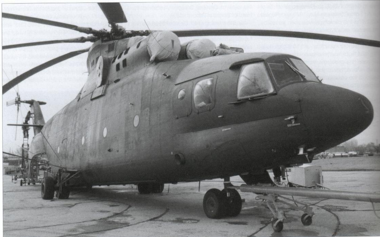
This Mi-26 wearing a dark camouflage scheme is probably intended for the Indian Air Force. It is seen here undergoing pre-delivery checks at the factory airfield in Rostov. Note the folding work platforms underneath the engine jetpipes; these are usually obscured by the 'anti-soot' panels.
