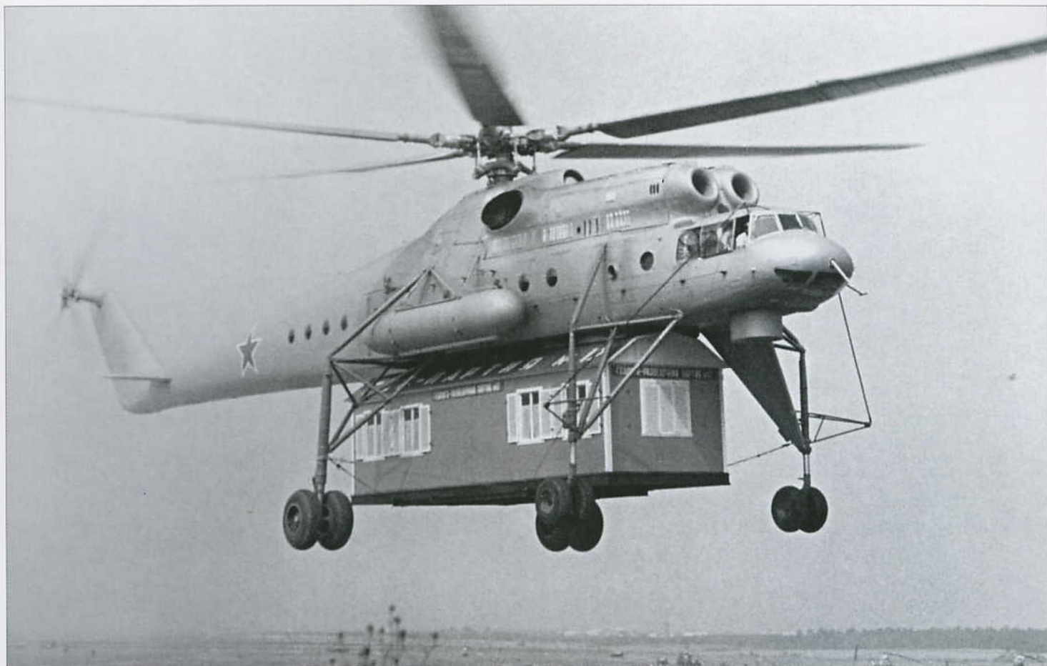
Above: Mi-10 c/n 04102 a few moments before touching down at Tushino with the prefabricated hut firmly pressed to the flat fuselage underside. The shape of the landing gear trusses obviously accounts for the shape of the hut's roof! Note the APU air intake and exhaust just aft of the flightdeck.
