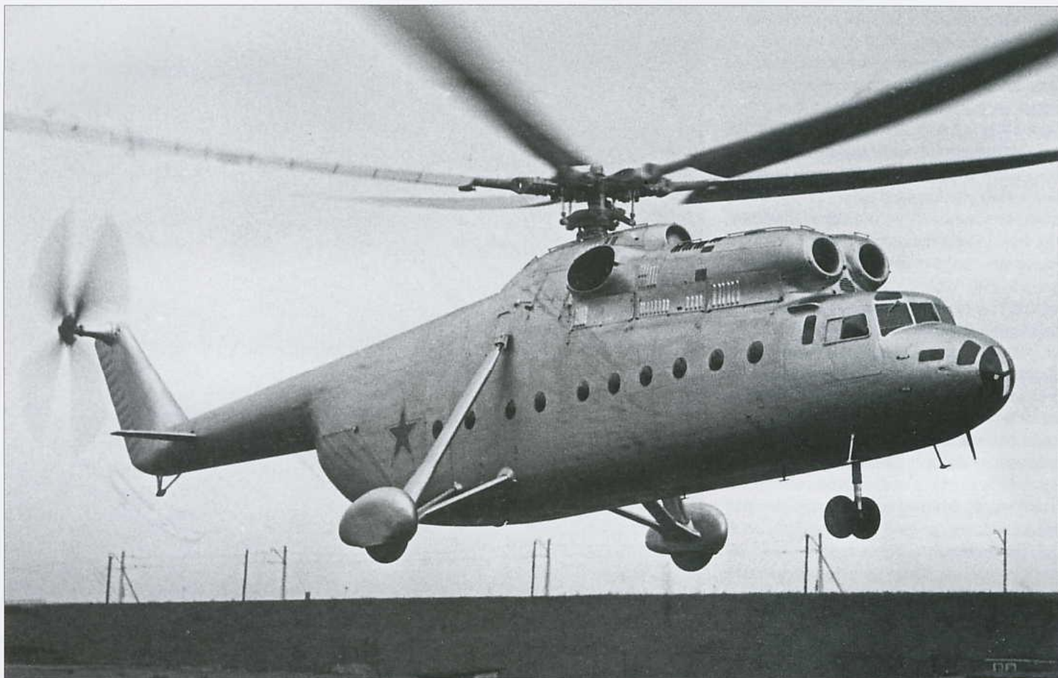
Above: This view shows the unbroken window arrangement on the starboard side. The narrow horizontal window on the nose is in the navigator's entry door. Below: The second prototype built at Moscow-Fili was the first Mi-6 to feature the characteristic wings.
