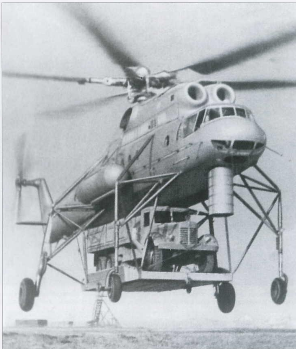
This view shows clearly how the cargo platform is secured to the landing gear struts by a set of struts. Note also the small wheels used for towing the empty platform around the apron.
