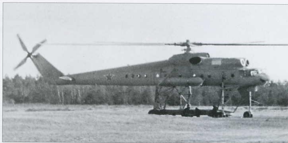
Above: An operational Soviet Air Force Mi-10 with the cargo platform attached. Most of the Mi-10s were later converted for ECM duties.
