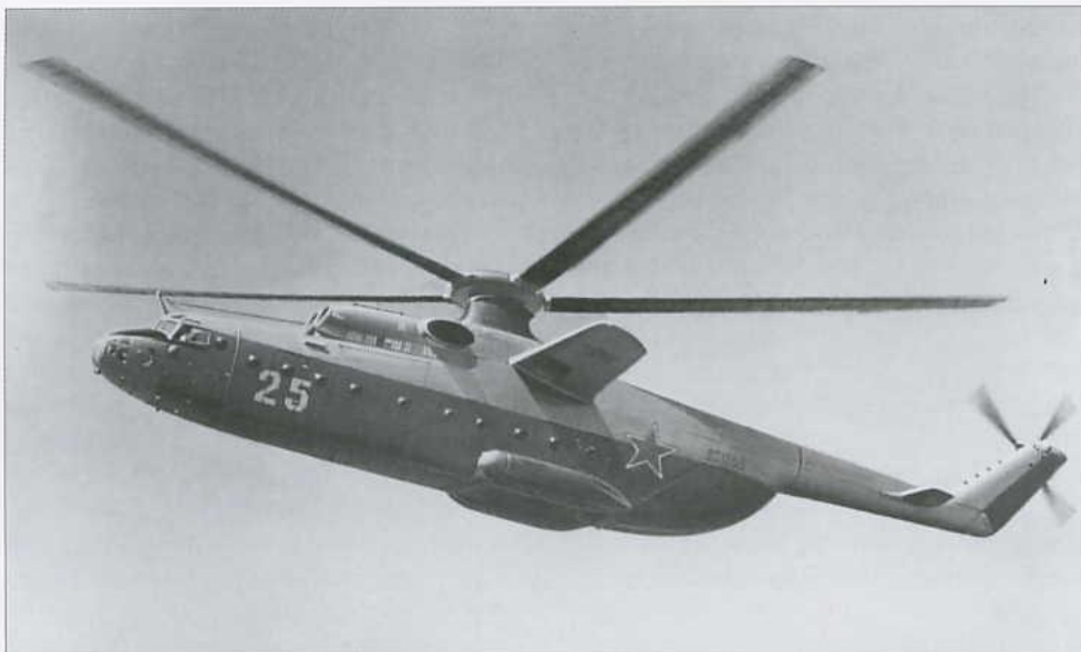
Above: This artist's impression of the modernised Mi-6M (the second helicopter to bear this designation) shows the retractable landing gear and the faired main rotor head. This was an early step towards the Mi-26.
