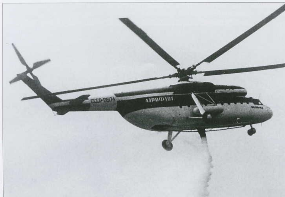
Another view of Mi-6PZh CCCP-06174 dropping water, this time with the water replenishment pipes stowed.
