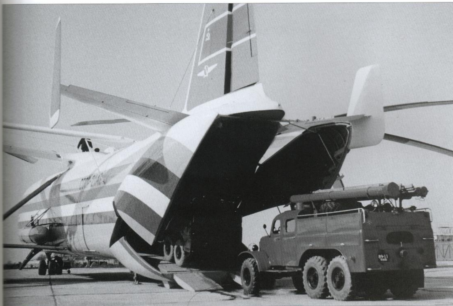
Above: In a demonstration of the V-12's capacities, two PMZ-13 fire engines based on the ZIL-157 are wheeled into the first prototype. The letters on the pre-1983 black number plate of the rear vehicle (89-11 YuASh) indicate it is registered in the Moscow Region. The cargo ramp/door design is clearly visible.
