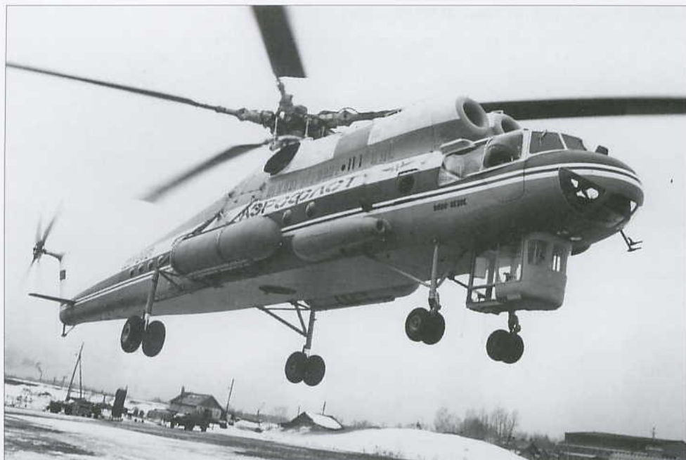
Above: Mi-10K CCCP-04121 (c/n 2163) of the Tyumen' CAD in 1973-standard Aeroflot livery. Note the KO-50 cabin heater ahead of the external fuel tank.
