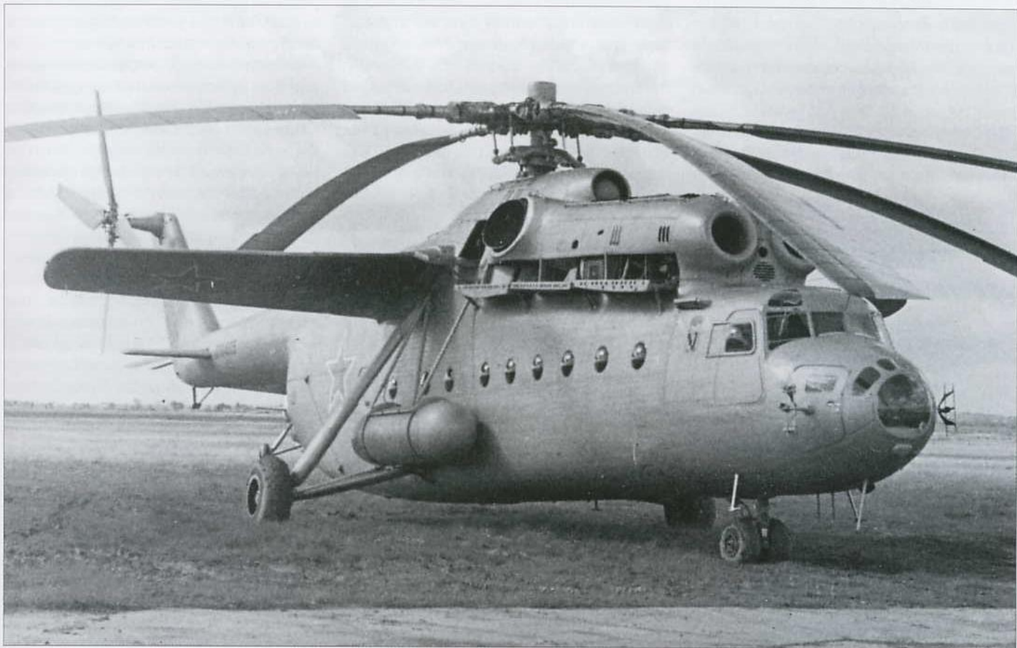
Mi-6 with the lower portions of the engine cowlings open. Moscow/Fili-built examples sometimes had the c/n stencilled on both sides. Note the different position of the engine cooling louvres; also, the starboard TACAN aerial is mounted directly on the navigator's station door on this example.
