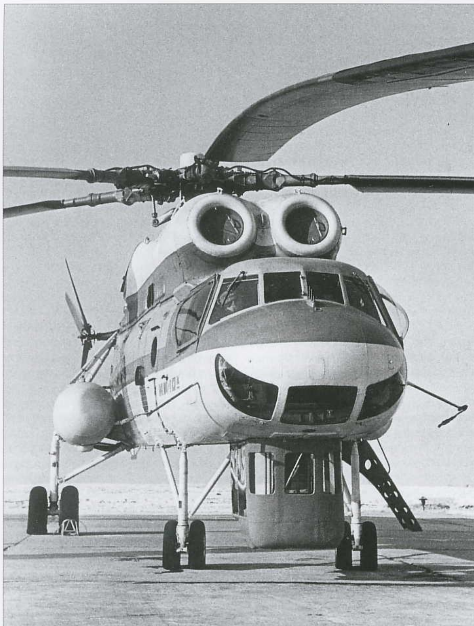
Another view of CCCP-29115. Note the rain gutter above the APU air intake window.
