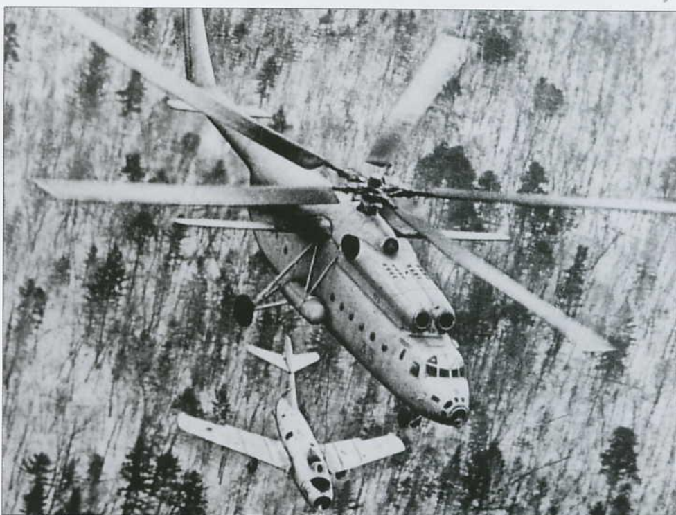
Top and above: Mi-6s were often used for transporting aircraft (not necessarily disabled) on a sling. Here, the 'victims' are two UTI-MiG-15 trainers and a single-seat MiG-15. Note the open machine-gun bay doors.
