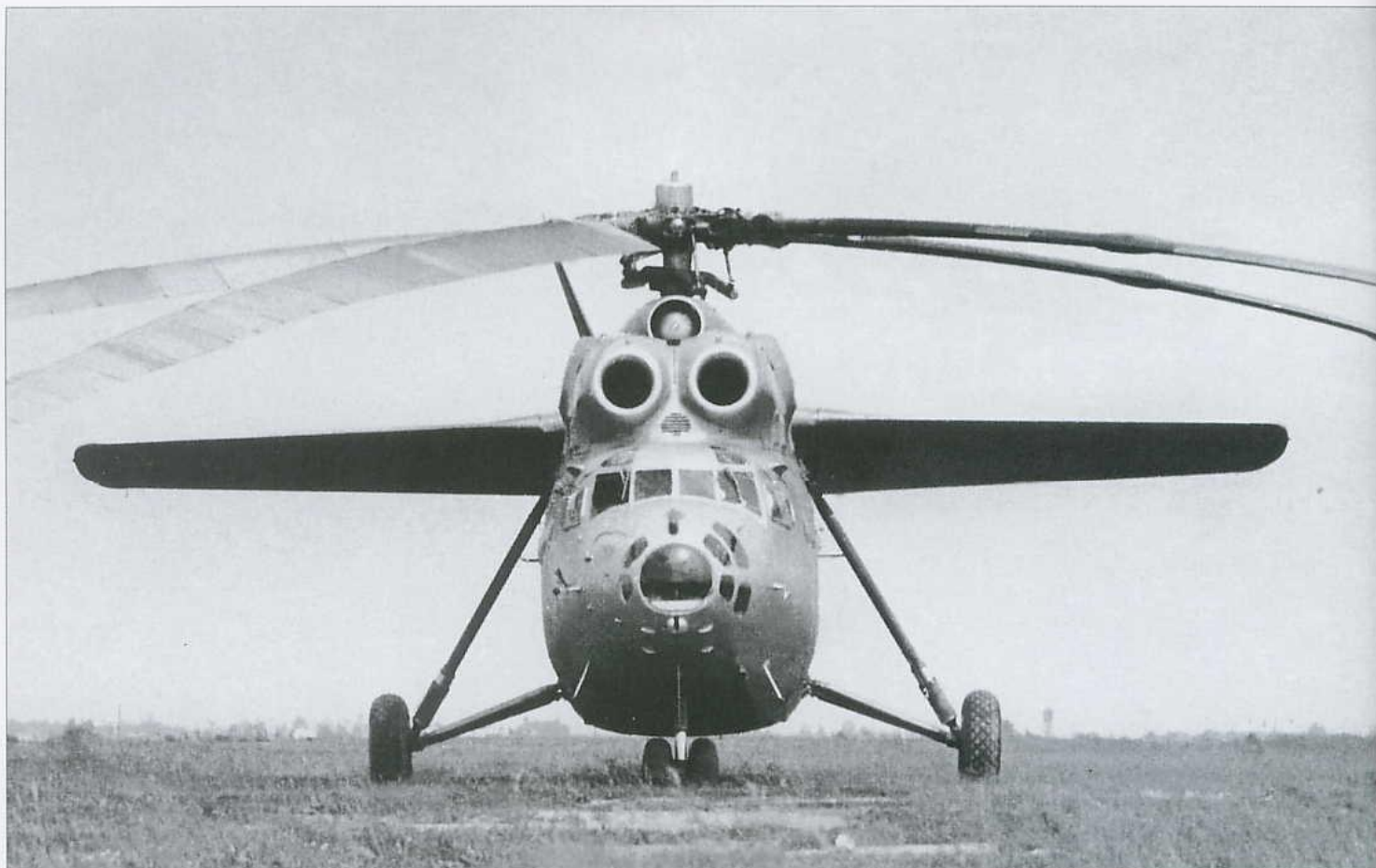
Above: Head-on view of an early-production Mi-6. Note the doors under the nose (with a bulge at the front) concealing the NUV-1M gimballed mount for an A-12.7 machine-gun.
