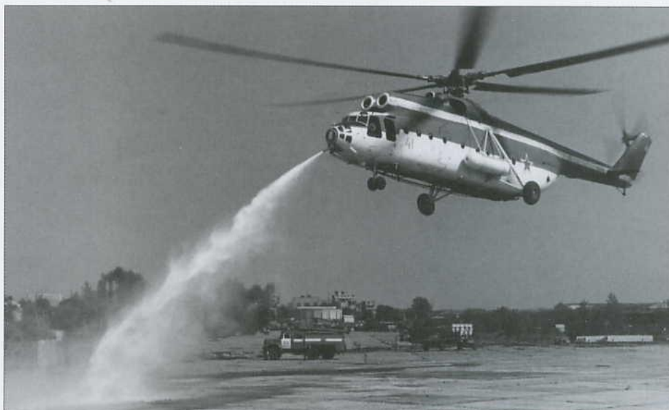
Mi-6PZh2 '41 Yellow' (c/n 9683901V) 'fires' the water cannon in a test flight. The emergency exit doors are removed – just in case. Note the water replenishment pipes and the ATs-40-131 fire engine in the background.
