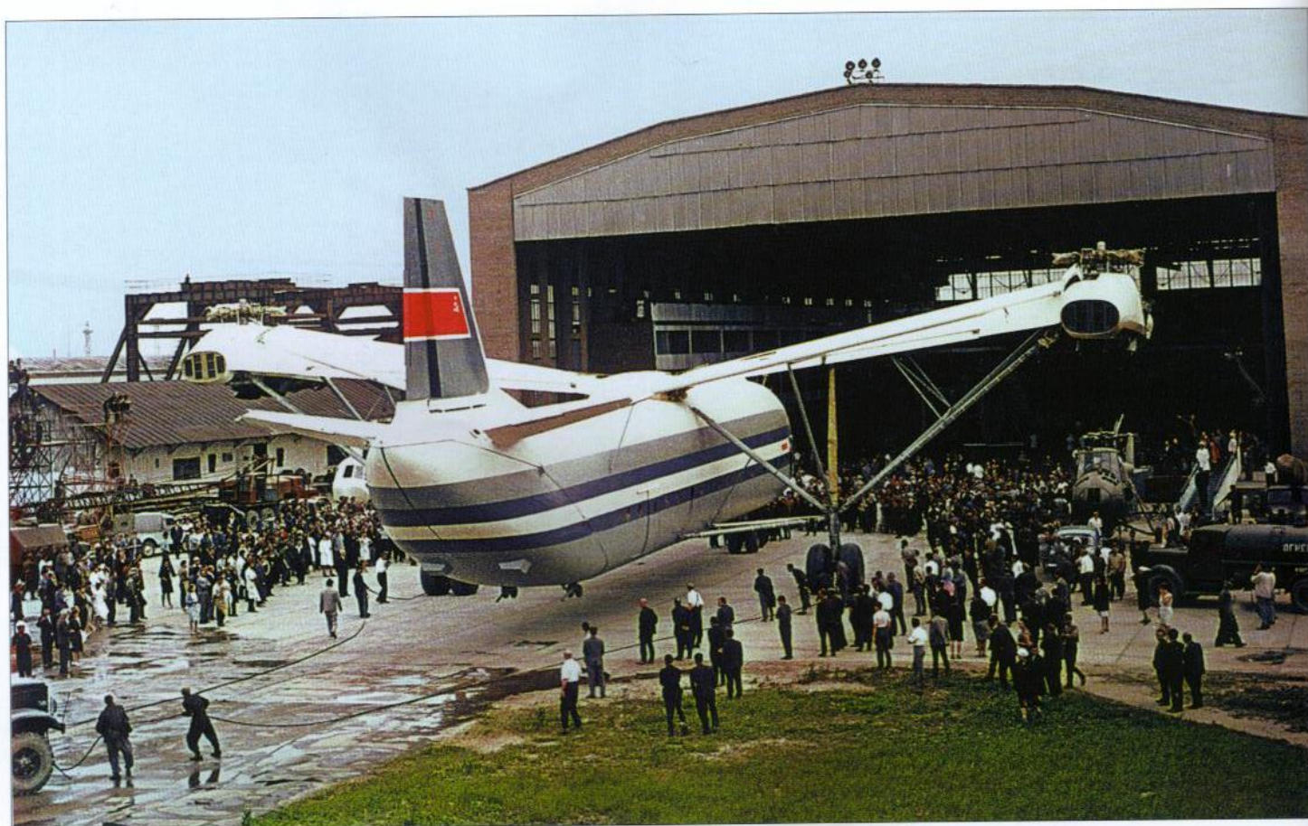
The ceremonial rollout of the first prototype V-12. The nose gear unit was inaccessible for tugs, so the helicopter was extracted by a KrAZ-255B, using strong cables hooked up to the main gear struts. Note the rotorless Mi-4 parked under the V-12's starboard wing and the MAZ-200 fuel bowser further to the right.
