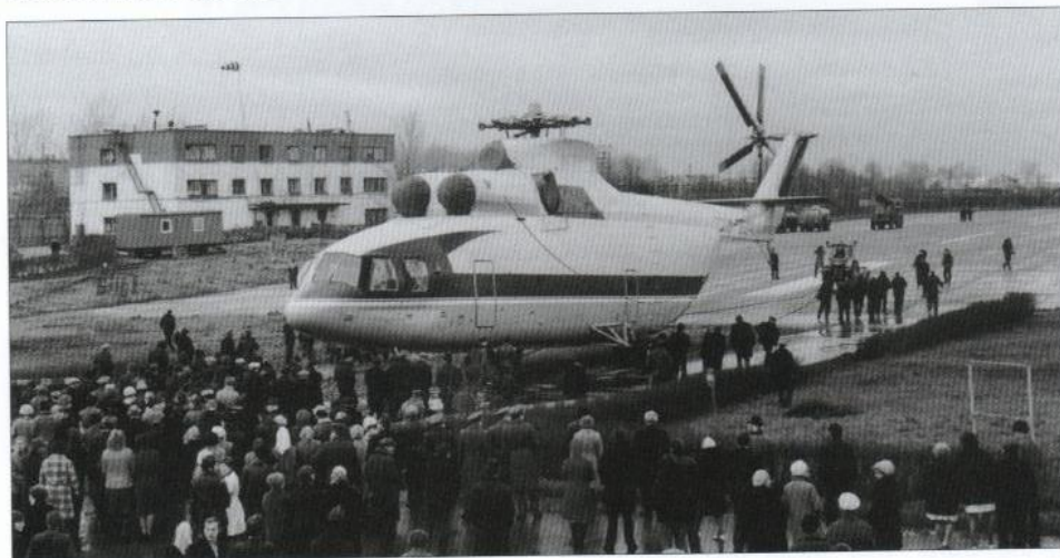
Above: The rollout of the Mi-26 prototype, CCCP-06141 in October 1977. Cloth covers are fitted over the engine air intake filters, cooling fan intake and jetpipes. Note that the helicopter lacks Aeroflot titles.
