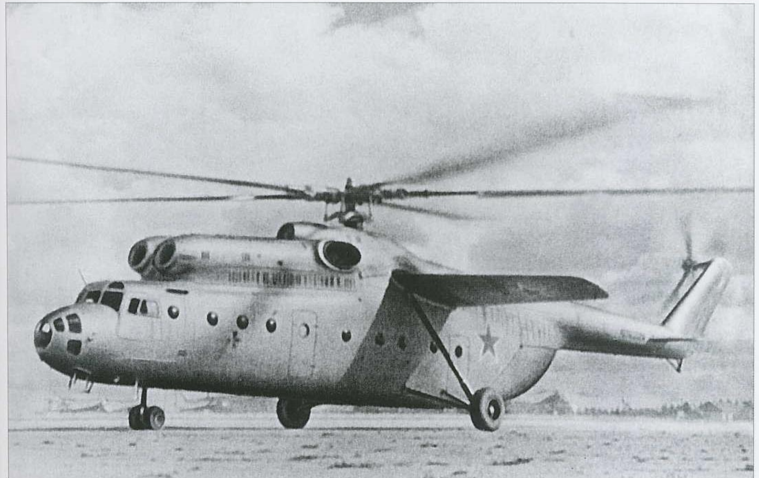
This production Mi-6 has the lateral TACAN aerials positioned well aft (compare with the example at the top).
