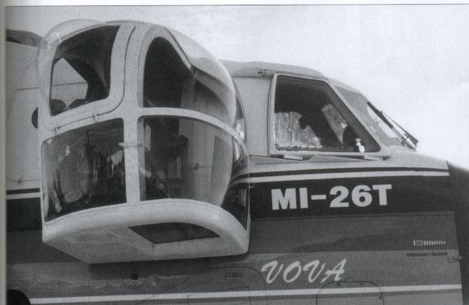
...and after. Mi-26T RA-06146 operated by Aerinn/Heli Harvest and named Vova was fitted with a custom-made external cab with extra controls attached to a flightdeck escape window for 'flying crane' work.
