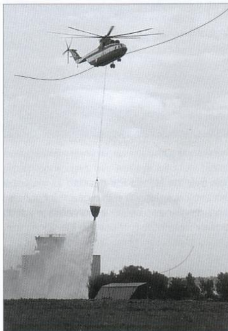
Above: Mi-26TS (c/n 34001212511) with a VSU-15 'Bambi Bucket' shows its firefighting capabilities.
