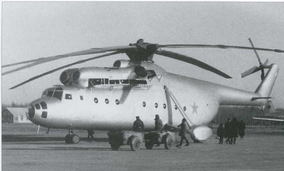
Above: The first prototype of the V-6 (Mi-6); the real thing was quite different from the original project. The main rotor head is wrapped in tarpaulins; note the ground power carts alongside.
