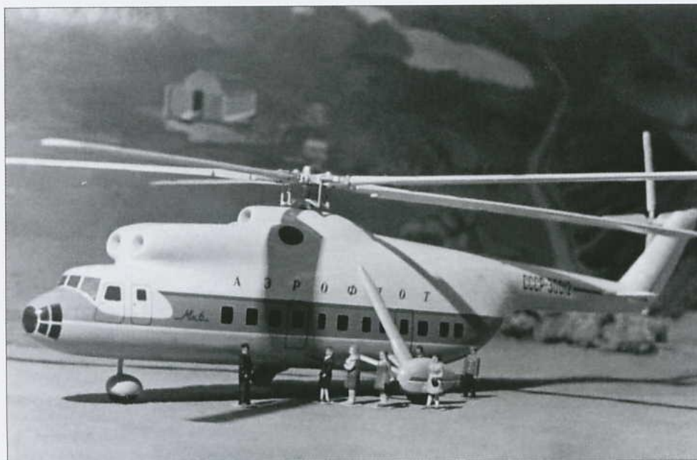
A model of the future Mi-6P passenger helicopter marked CCCP-30012. Note the wheel spats on all three landing gear units, the lack of wings and the window arrangement which did not match the real thing.
