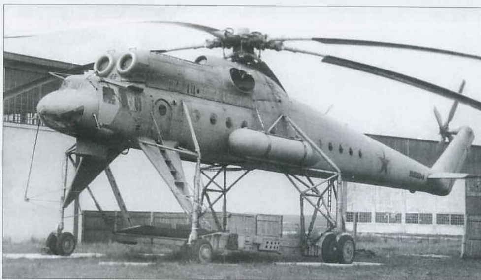
This production Mi-10 (c/n 8680604K) built in 1968 was donated to the Soviet Air Force Museum in Monino. Note the flightdeck escape door replacing the earlier sliding blister window.
