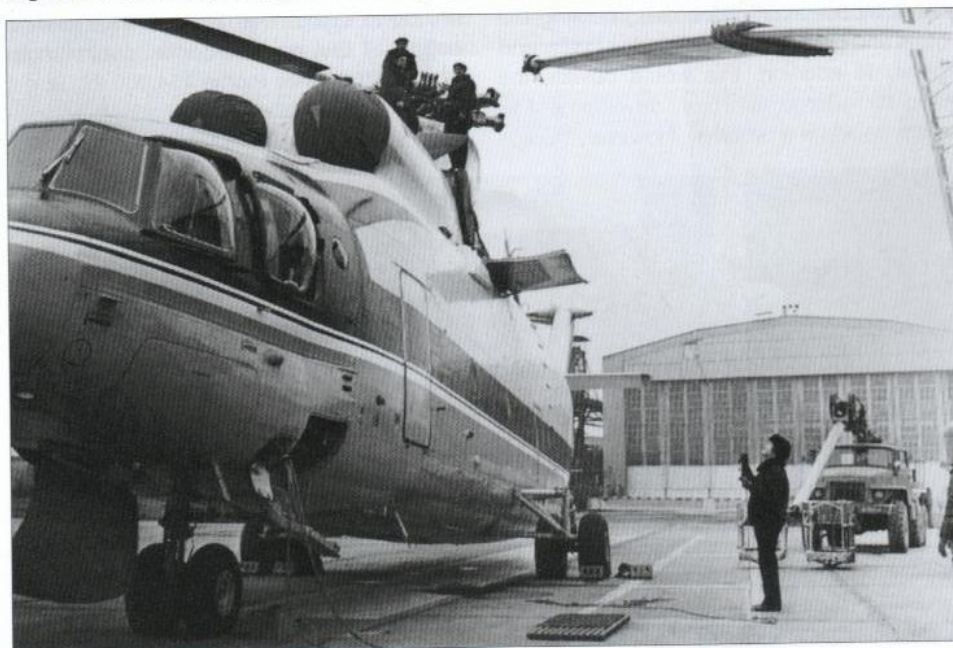
A crane is used to install the Mi-26 prototype's main rotor blades. The vehicle in the background is an AGP series 'cherry picker' servicing platform based on a petrol-engined Ural-375D 6 x 6 army lorry.
