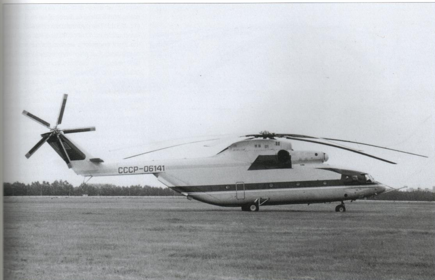
Above and below: The first prototype Mi-26 during initial flight tests. Note the asymmetrical door/window arrangement, the port side maintenance access steps, the air data boom attached to the nose radome and the strakes on the clamshell cargo doors. These strakes were later deleted as unnecessary.
