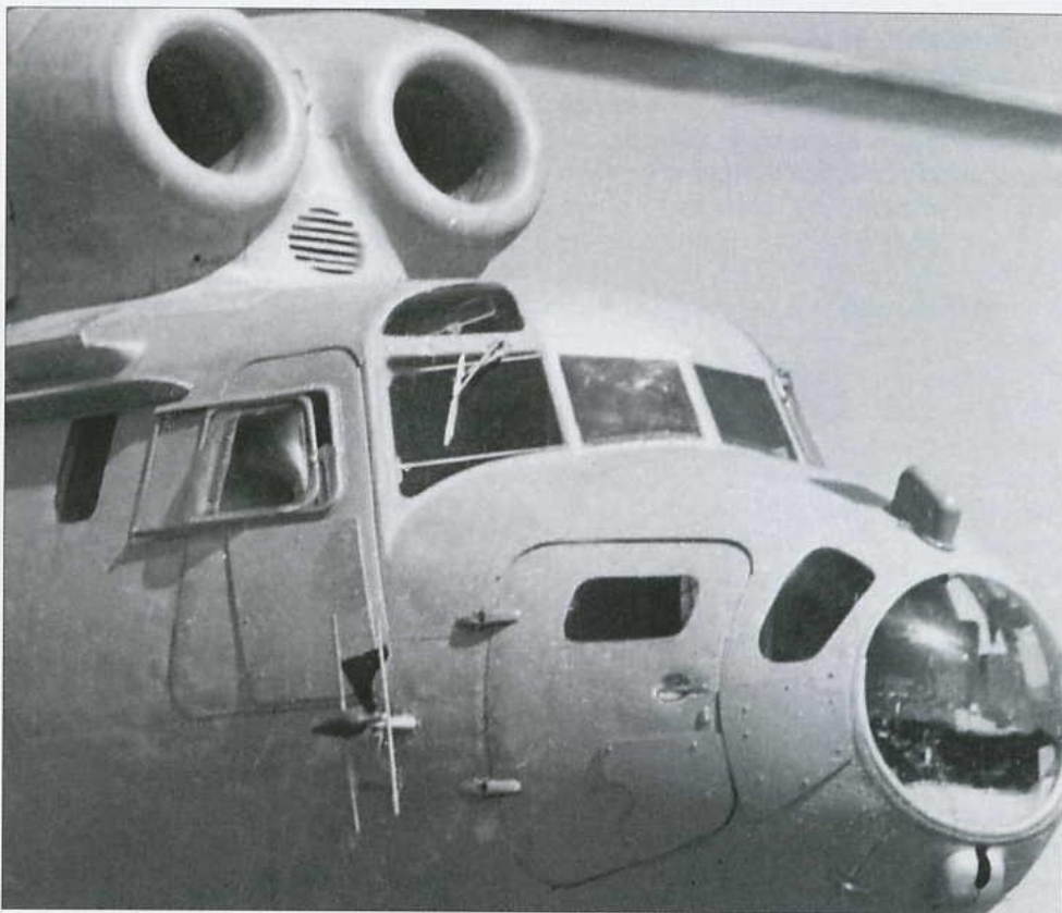
The forward fuselage (crew section) of an early Mi-6 modified by riveting additional armour plates to the sides of the navigator's station and the flightdeck escape doors. Note the open direct vision window.
