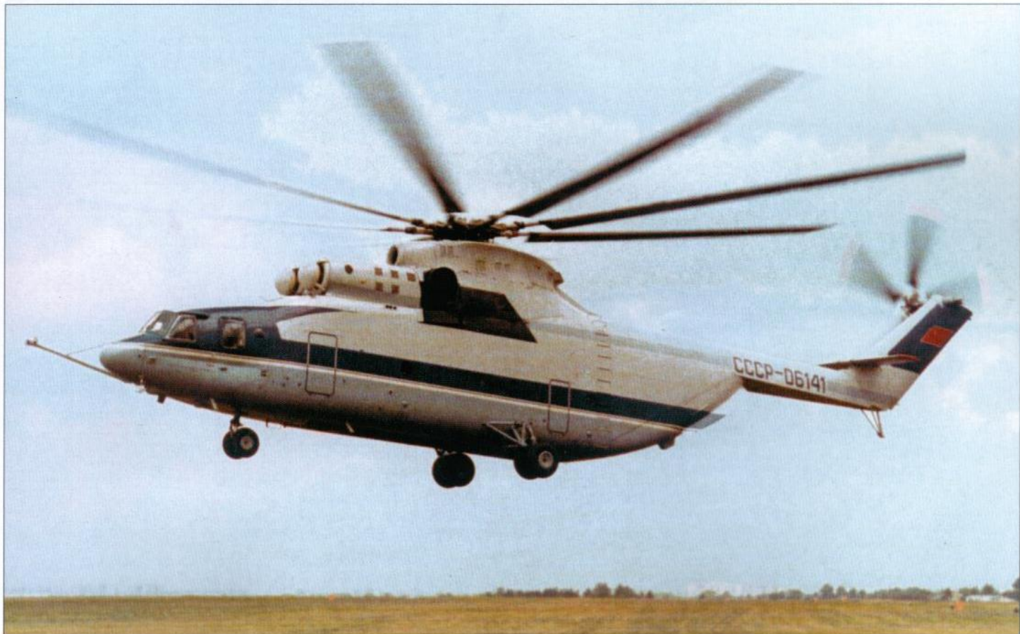
CCCP-06141 takes to the air with an instrumented air data boom fitted. It was the only Mi-26 to feature strakes on the rear clamshell doors.
