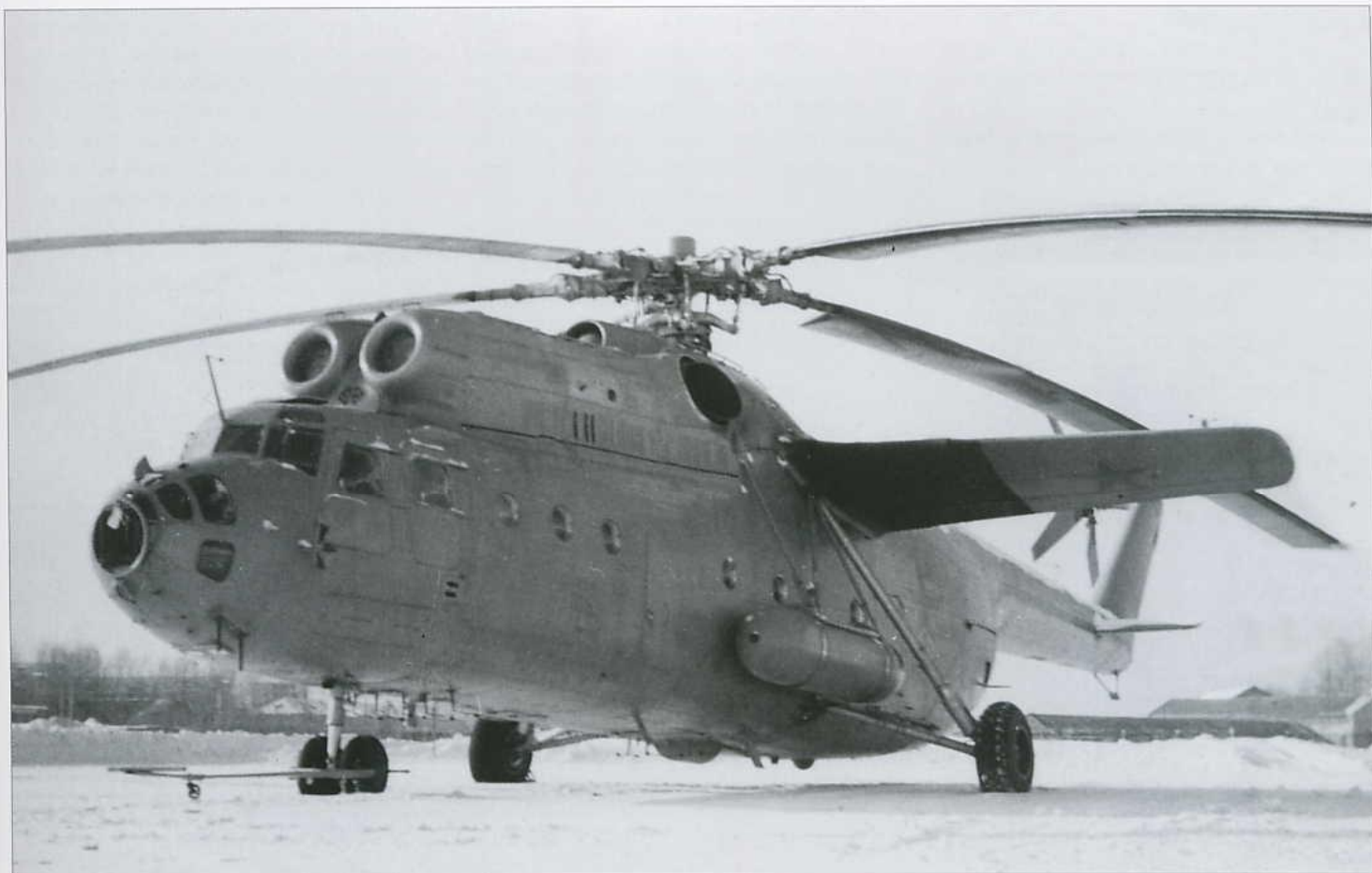
Above: A fine winter study of an uncoded Soviet Air Force Mi-6AYa (Mi-22) airborne command post in standard overall grey camouflage. Note the modified nose glazing, the windowless doors and the ventral bulge over mission equipment replacing the cargo suspension system hatch.
