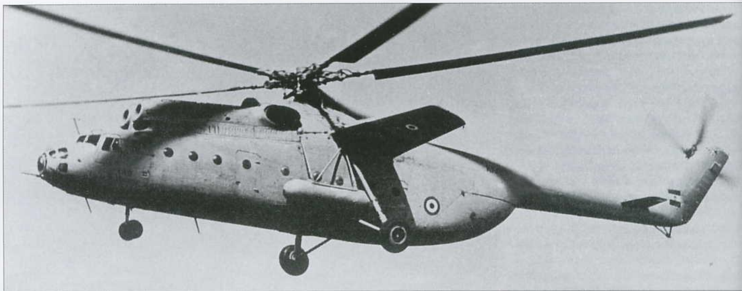
Above: The Egyptian Air Force took delivery of a number of Mi-6s, including this example with the late-standard nose glazing design.
