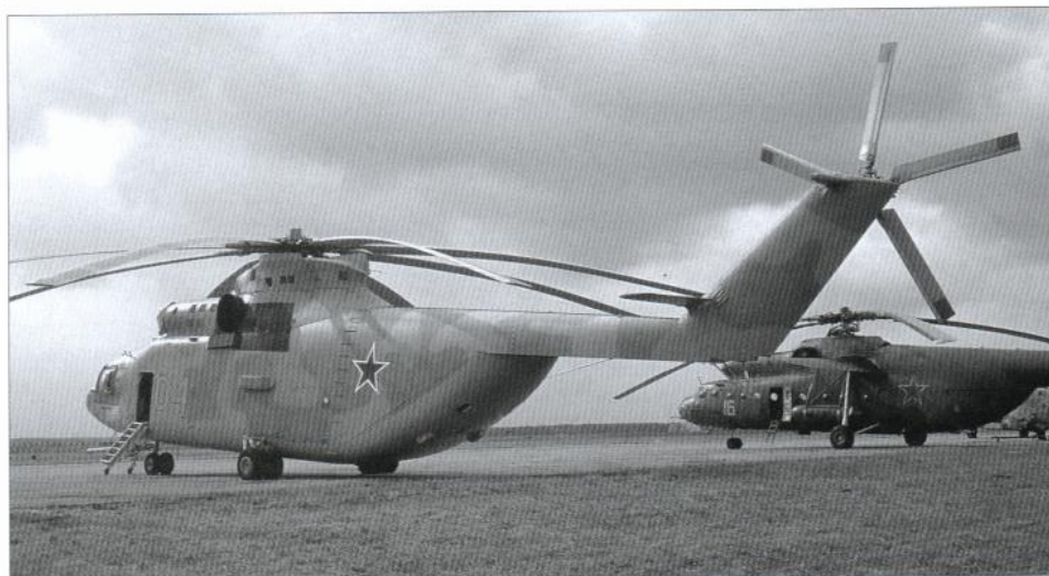
Above: Mi-26 '04 Yellow' in company with Mi-6A '16 Yellow' and a Mi-24P at Kubinka AB. Note the characteristic chaff/flare dispensers above the main gear units fitted to most Soviet/CIS military examples.
