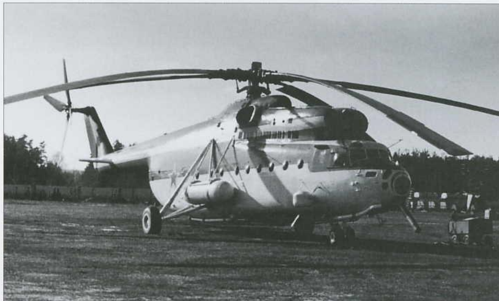
Above: An uncoded Mi-6PZh2 fire-fighting helicopter seen during trials. Note the chin-mounted water cannon and the small cylindrical tank on the starboard side of the nose characteristic of this version.
