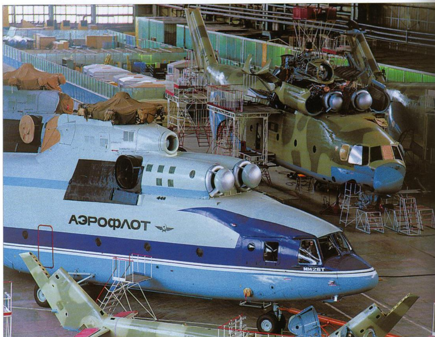
A quasi-Aeroflot Mi-26T owned by the Russian Ministry of Interior shares the assembly shop at the Rostvertol plant with two sister ships in Russian Air Force camouflage and a pair of Mi-24 attack helicopters. Note how the radome swings open to starboard.
