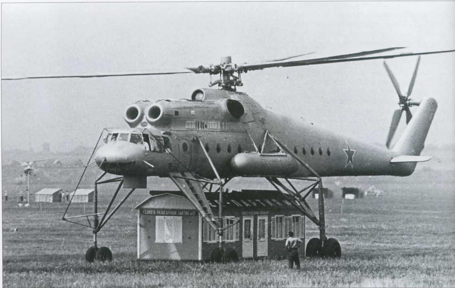
Above: The second prototype Mi-10 (c/n 04102) in its original military guise during the air event at Moscow-Tushino on 9th July 1967. The helicopter has just delivered a prefabricated hut marked 'Geological prospecting party No.17' to the airfield and lowered it to the ground, using the internal winch.
