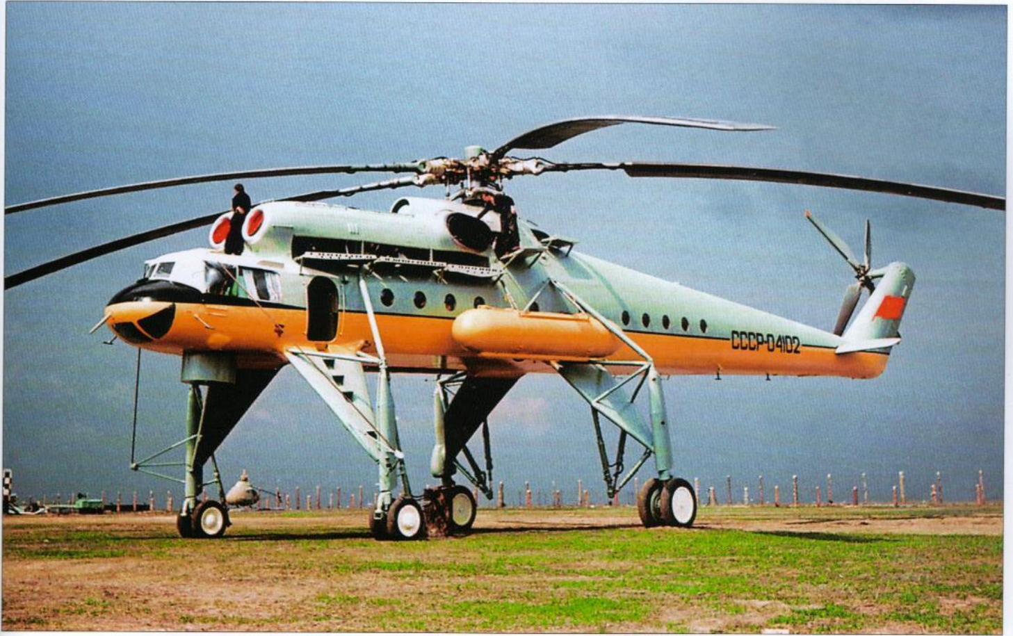
Above: The second prototype in civilian guise as CCCP-04102 with new nosewheels and faired-over trusses on all four landing gear struts. It was in this guise that the machine was displayed at the 1965 Paris Air Show.
