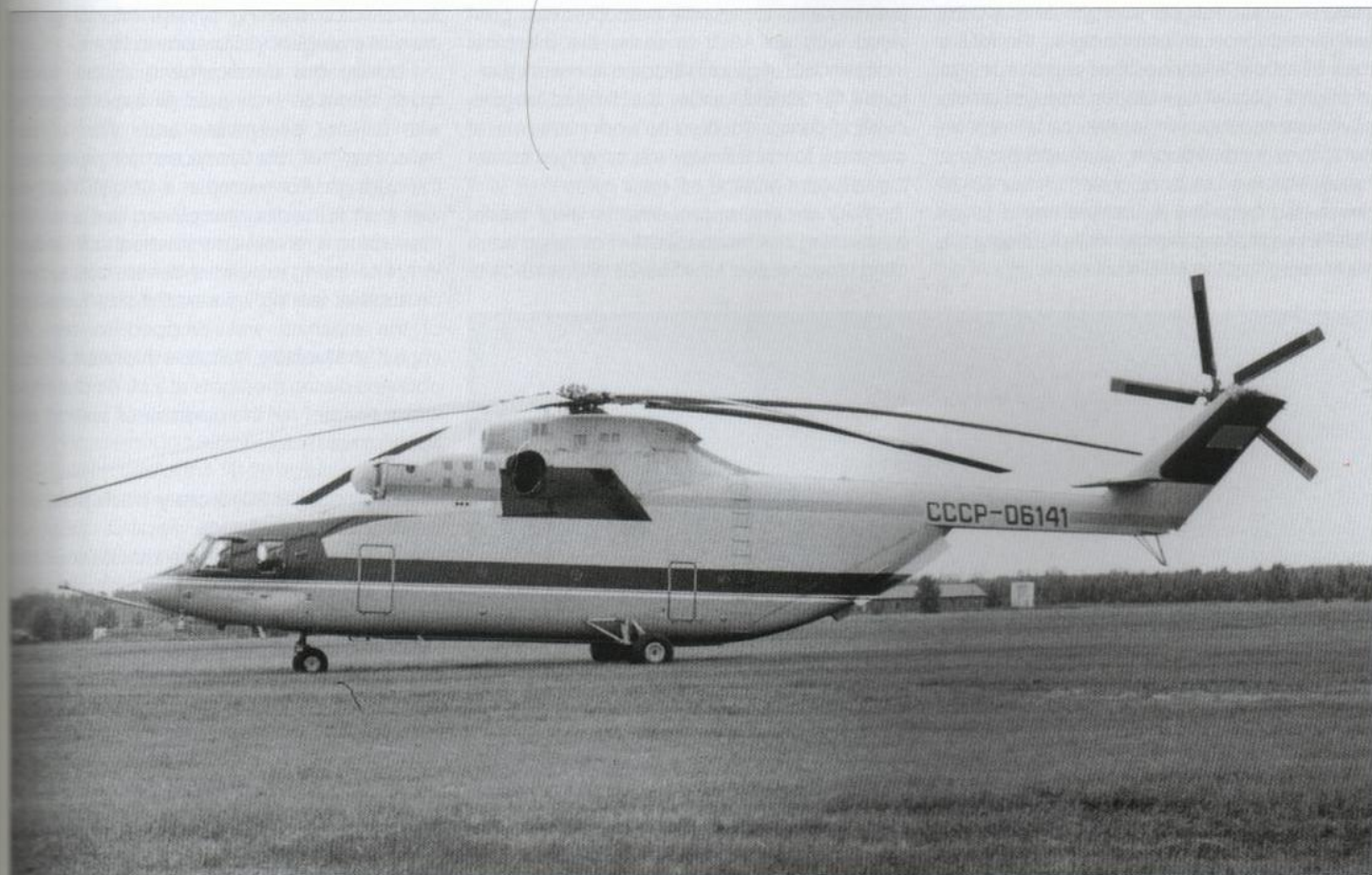
Above and below: The first prototype Mi-26 during initial flight tests. Note the asymmetrical door/window arrangement, the port side maintenance access steps, the air data boom attached to the nose radome and the strakes on the clamshell cargo doors. These strakes were later deleted as unnecessary.
