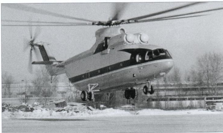
Mi-26 CCCP-06141 hovers for the first time on 14th December 1977. No air data boom is fitted yet. Note that the black anti-soot panels near the engine jetpipes were considerably enlarged later.
