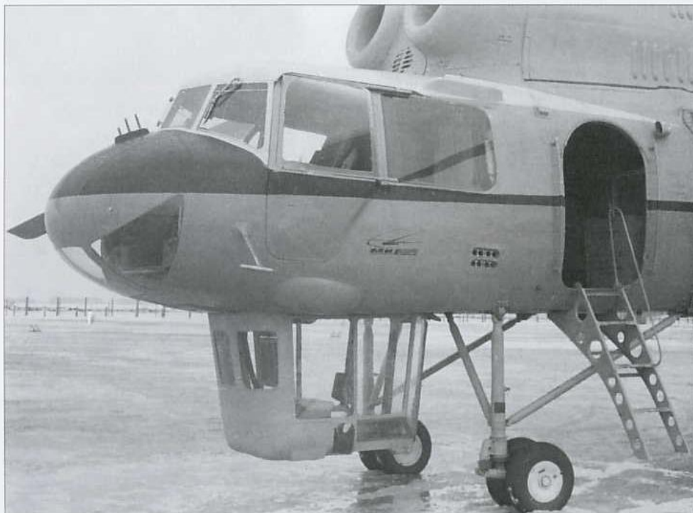
Close-up of the Mi-10K prototype's forward fuselage, showing the nose gear units, the ventral cockpit and the entry door with a boarding ladder.
