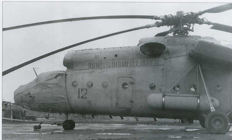
Above: Another aspect of Mi-22 '12 Red', showing the ventral antenna farm. Note that this example has windows in the port side doors; the absence of star insignia on the wings is also noteworthy.
