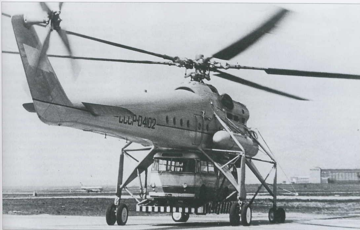
Above: Mi-10 CCCP-04102 makes a tight taxiing turn, carrying a L'vov-built LAZ-695 sans suffixe bus. Note the extreme negative incidence of the stabilisers, the cargo hoist arm above the starboard-side cargo door and the Tupolev Tu-124 airliner taxiing in the background.
