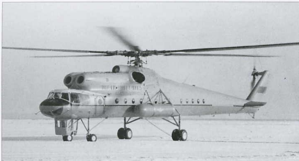
Above: The prototype of the Mi-10K 'flying crane' helicopter during initial flight tests. An external sling cable is attached to the helicopter
