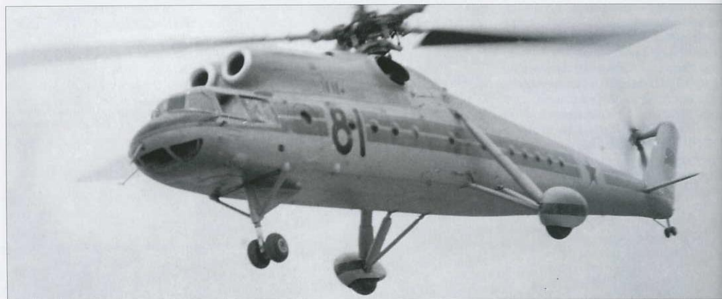
The photos on this page show the one-off, record-breaking tricycle-gear Mi-10R; note the design of the nose gear unit, the flat side windows of the flightdeck and the lack of the APU. The helicopter wore dayglo orange stripes along the fuselage and a Soviet flag on the fin to complement the Air Force star insignia.
