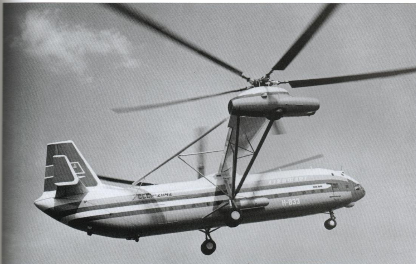
Above: The V-12 was impressive enough on the ground, but in flight it was a truly awesome sight. Note the oil cooler air outlets at the rear ends of the engine nacelles; the oil cooler air intake scoops are located on the outer faces of the nacelles in line with the rotor heads.
