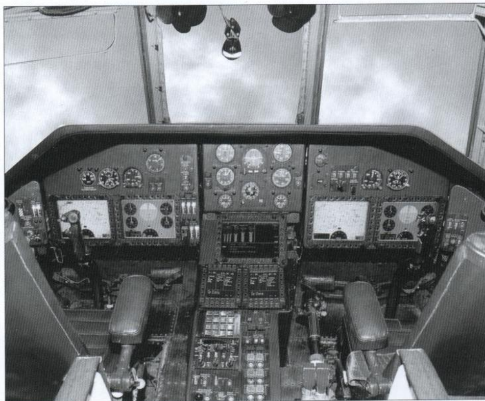
The flightdeck of the proposed Mi-26T2 configured for a crew of two, with five large liquid-crystal displays.
