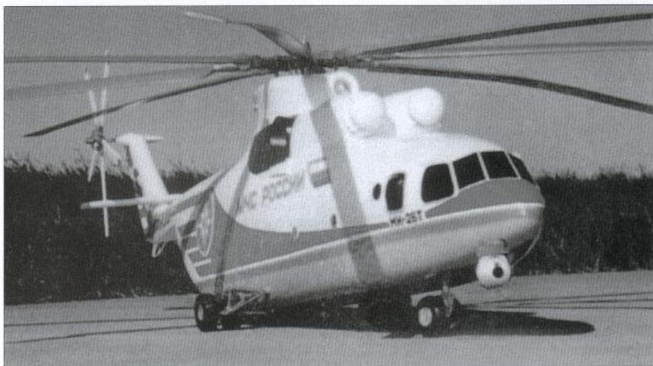
This model depicts another configuration proposed for EMERCOM of Russia with a Urals Optomechanical Plant (UOMZ) GOES-320 gyro-stabilised opto-electronic system under the nose.
