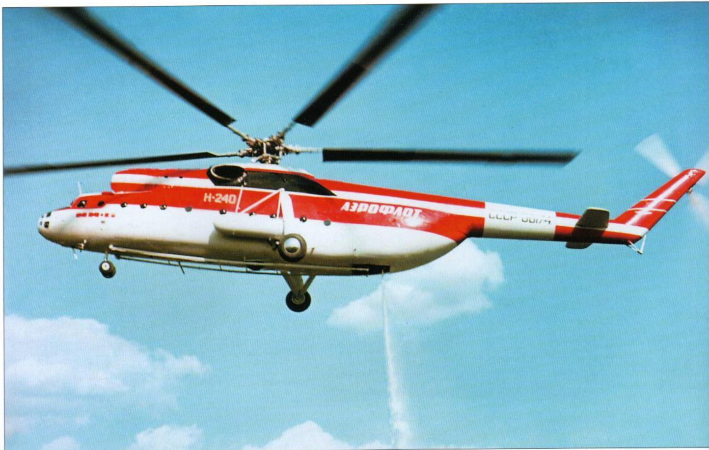
Above: CCCP-06174 in its new 'fire engine' livery following conversion into the Mi-6PZh prototype. Excess water is spilling from the mouthpiece of the twin water replenishment pipes.
