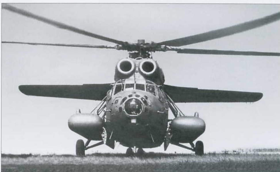
This head-on view of the Mi-6M shows the open doors in the large lateral weapons panniers.
