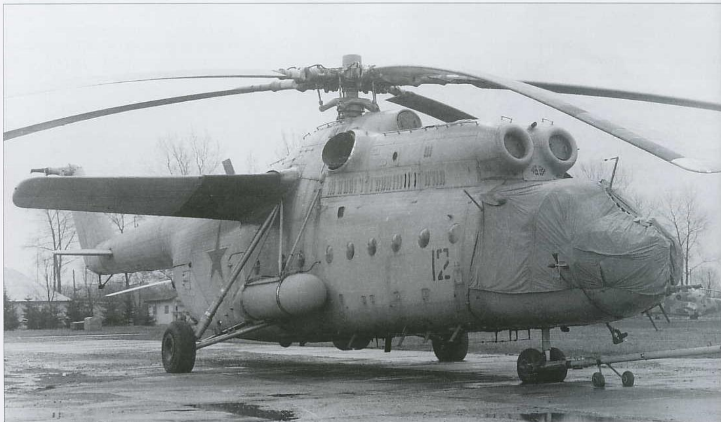
'12 Red', a Mi-6AYa (Mi-22) airborne command post, awaits repairs, hence the lack of the tail rotor. Note the large blade aerial atop the root of the tailboom which is the Mi-22's main identification feature.
