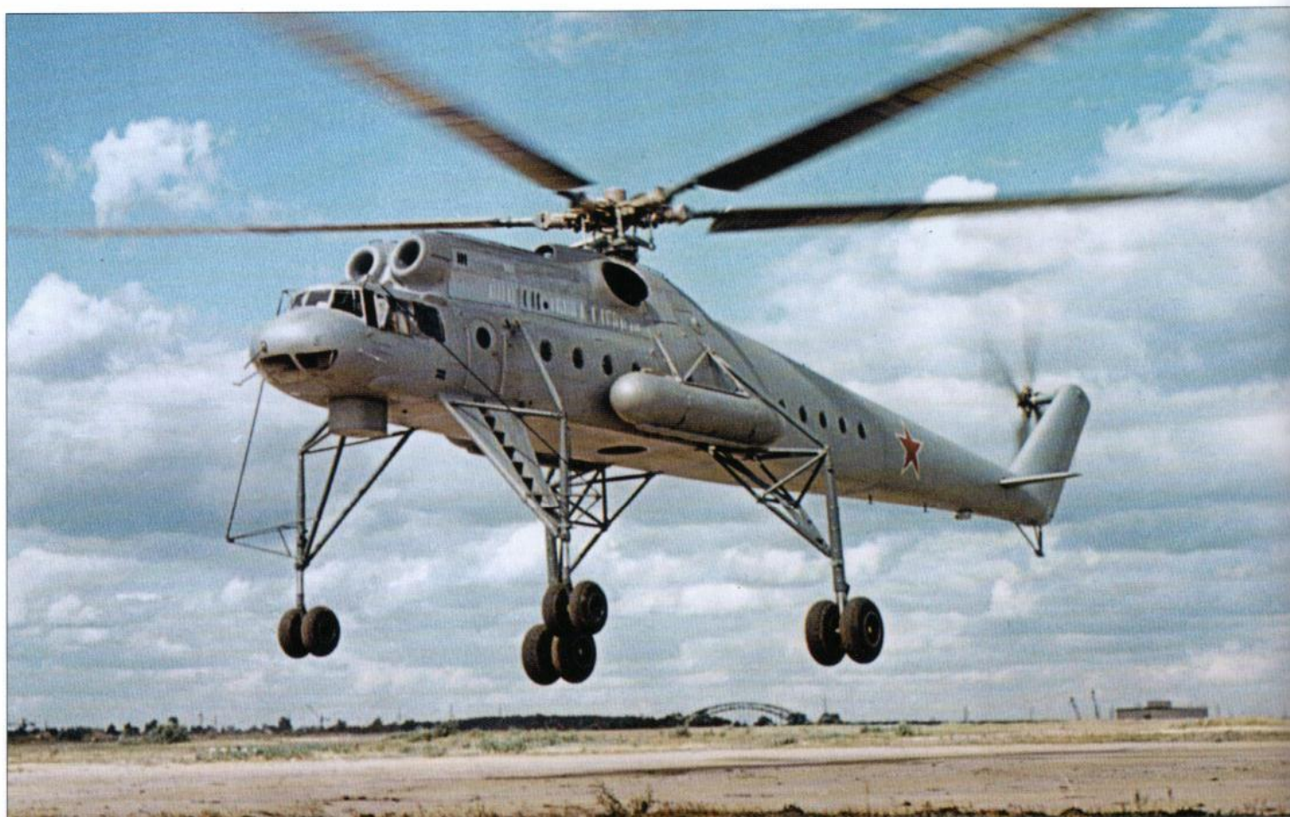
Above: A Mi-10 seen seconds after lifting off. Note the ventral hatch for the external sling system amidships.
