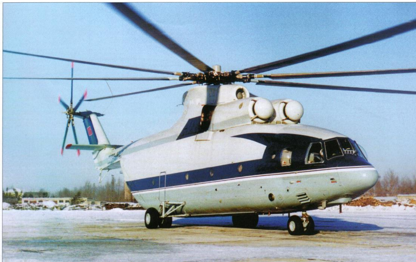
Above: The first prototype Mi-26, CCCP-06141, during ground engine runs shortly before the first hover. Note the open 'gills' of the APU air intake under the co-pilot's sliding window and the lack of Aeroflot titles.
