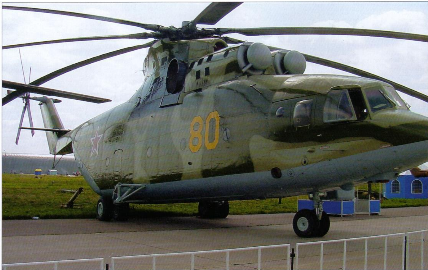
Above: Mi-26PK '80 Yellow' (c/n 34001212081) operated by Vzlyot in the static park at the MAKS-2001 airshow. The port side cockpit for 'flying crane' operations is not visible here. Note the lack of chaff/flare dispensers.
