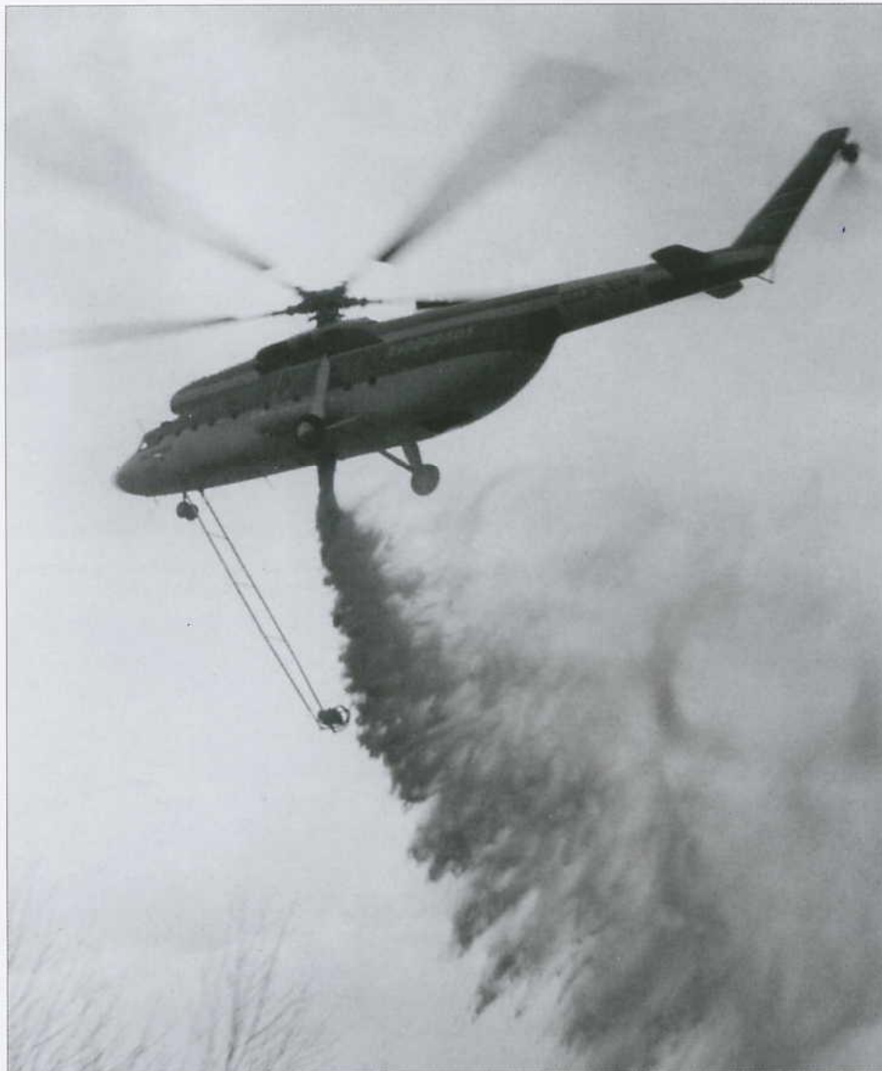
Above: The ill-starred cannonless Mi-6PZh (CCCP-06174) dumps its load of water through the ventral nozzle. The hinged water replenishment pipes are lowered into position; note the pump unit at the end.
