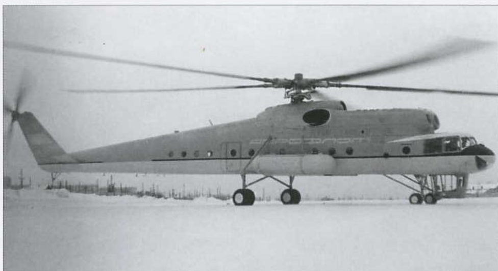
Above: This view shows the Mi-10K's shorter external fuel tanks. As originally flown the prototype wore a grey/yellow colour scheme similar to that of Mi-10 CCCP-04102 and no registration.
