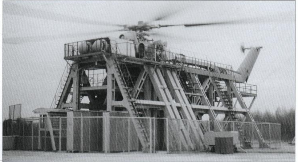
Above: 'The Partially Invisible Helicopter' – the Mi-26's full-scale powerplant/dynamic components test rig.
