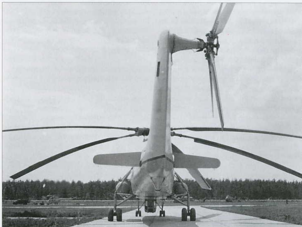
Above and below: Front and rear views of the Mi-10K prototype (c/n 5680202K). Note the bulged blister windows of unequal size (the captain's blister is bigger).
