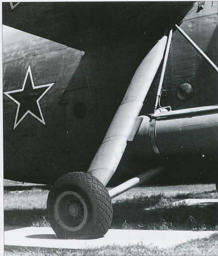
Left: The centre fuselage and the port external tank with its retaining straps and N-strut. Right: The starboard main landing gear unit with a faired shock strut.
