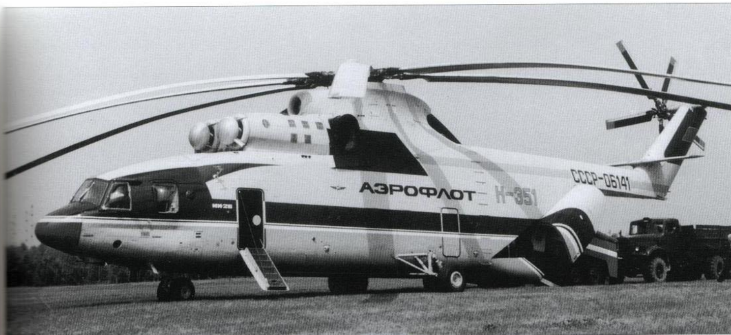
Above: Mi-26 СССР-06141, now with Aeroflot titles, a red radome and the Le Bourget exhibit code H-351, swallows an ATs-40-131 fire engine, with a KrAZ-255B1 heavy-duty 6 x 6 lorry waiting its turn. Note the entry door design.
