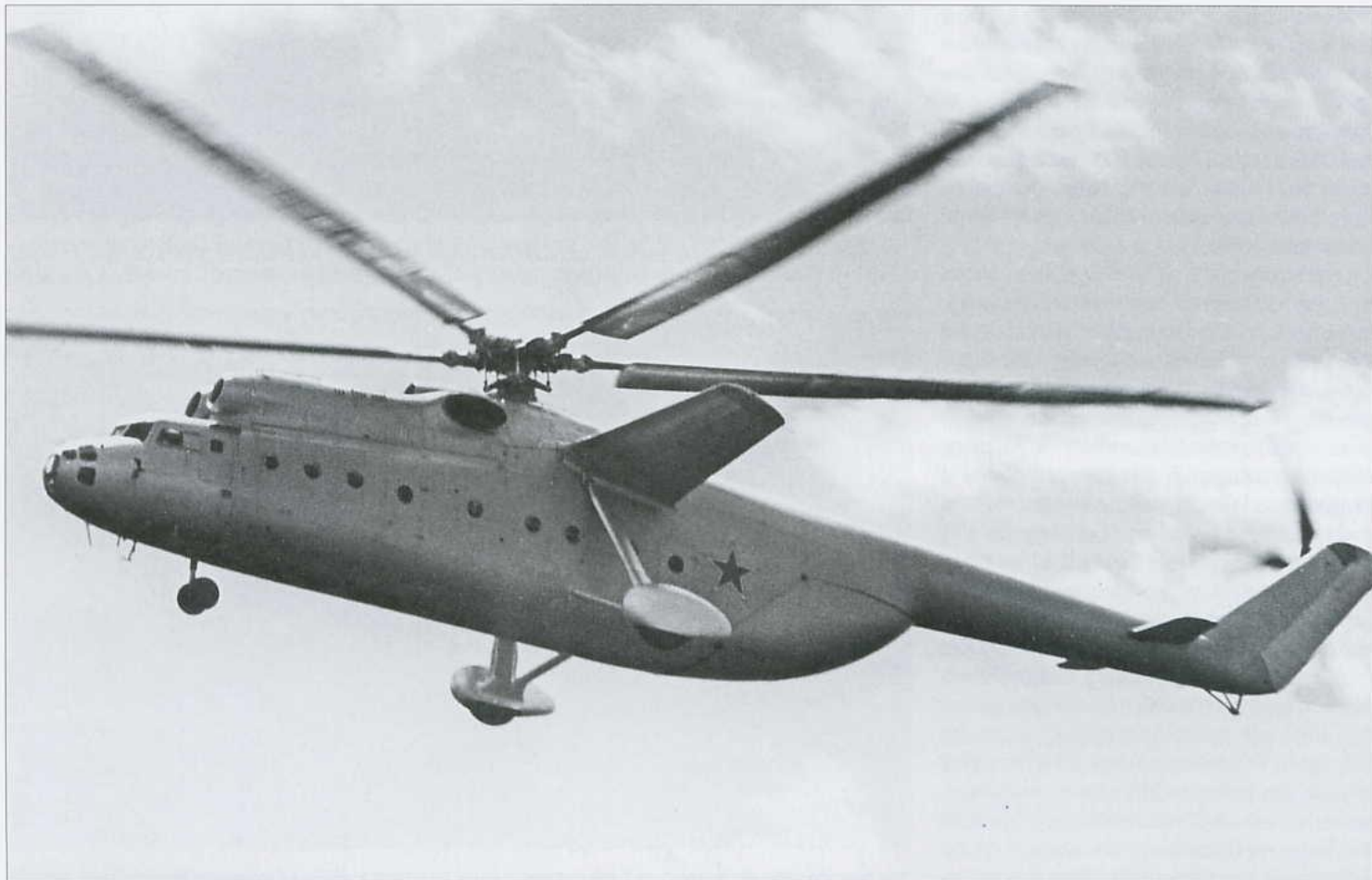
Above: This view shows the unbroken window arrangement on the starboard side. The narrow horizontal window on the nose is in the navigator's entry door. Below: The second prototype built at Moscow-Fili was the first Mi-6 to feature the characteristic wings.
