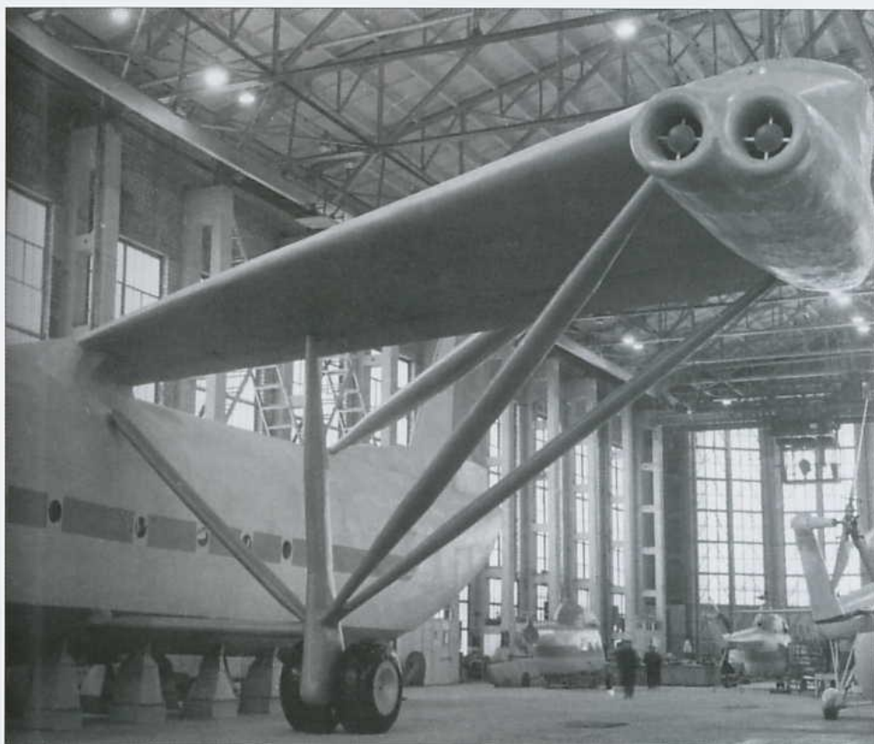
Above and below: The full-scale mock-up of the V-12 in the assembly shop of plant No.329 in Panki. Note the stepped nose and the T-tail; both features changed before the real thing was built. The engine nacelles were also reshaped later on.
