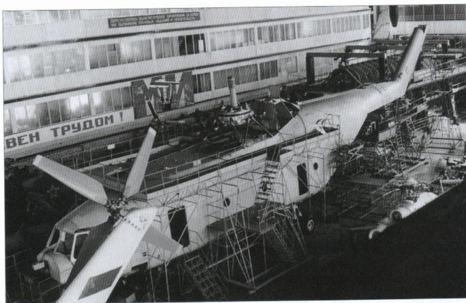
Above: The full-scale mock-up of the Mi-26 nearing completion at Plant No.329 in Panki, with the tail rotor of a Mi-6 in the foreground.
