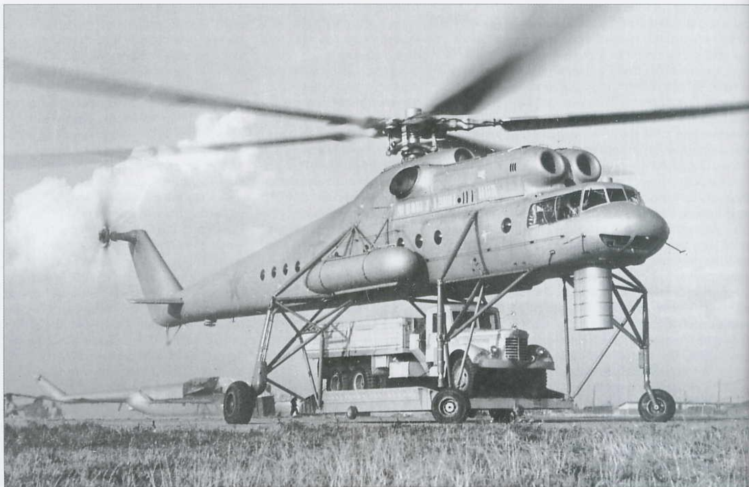
Above and below: The first prototype V-10 (Mi-10), c/n 04101, as originally built with single wheels on all four landing gear units and outward-canted main gear struts. Note the deployed escape chute and the suspended cargo platform; it is loaded with a Yaroslavl'-built YaAZ-210 6 x 4 dropside lorry.
