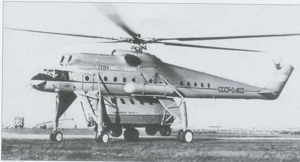
Mi-10 CCCP-04102 after outfitting as a Mi-10UPL. The automotive trailer suspended under the fuselage is a mobile ore analysis laboratory.
