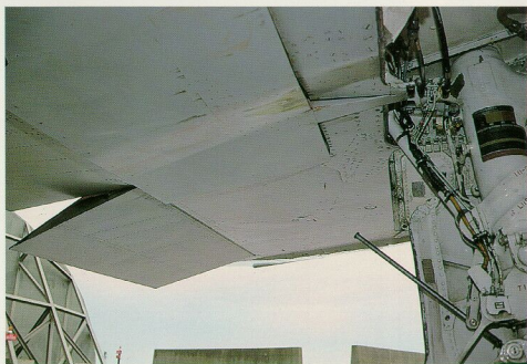
The bottom speed brake just aft of the main gear well. Part of the latter can be seen at far right.
