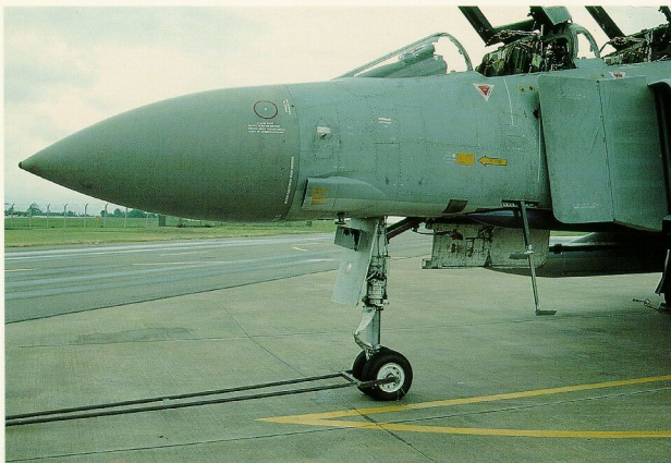
(Top) The aft end of the left inboard pylon with part of the Sidewinder launching rail in detail. (Left) The nose section of FGR.2 XT891 viewed from the left. Note the different color of the nose radome. A sensor probe is located just below the large ram air coolant intake on the lower side of the fuselage. Also note the typical FGR.2 nose landing gear door with a different antenna blade and the lack of the three landing lights featured on the FGR1 (see previous page). The retractable boarding ladder can be seen in front of the intake splitter plate.
