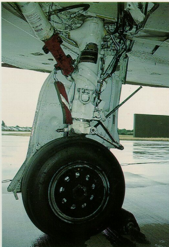
(Left & far left) Outboard view of the right main landing gear strut. Another "retraction preventor" is installed on the main gear actuator. Note the full compression of the gear strut which features another tie-down ring and the scissor linkage bar.
