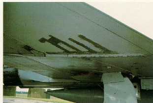
(Top) A view on the outer wingtip folding mechanism of the right wing.
