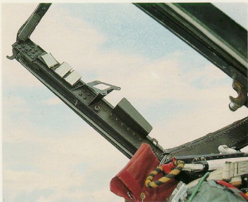
(Above) Radio call signs and checklists can be seen mounted on the canopy framing.
