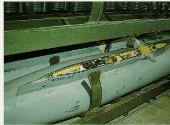
(Above) A detail seldom shown in books such as this. The fuel connecting lines and electrical wiring can clearly be seen. Note the pylon is an integral part of the fuel tank. (Left) A 308 gallon(US) tank and a travel pod are mounted on the outer wing and inboard pylon respectively on this Leuchars based FGR.2 Phantom. Note the very pointed inboard pylon with an unusual bomb rack holding the travel pod and the way the pylon is mounted to the lower wing surface.
