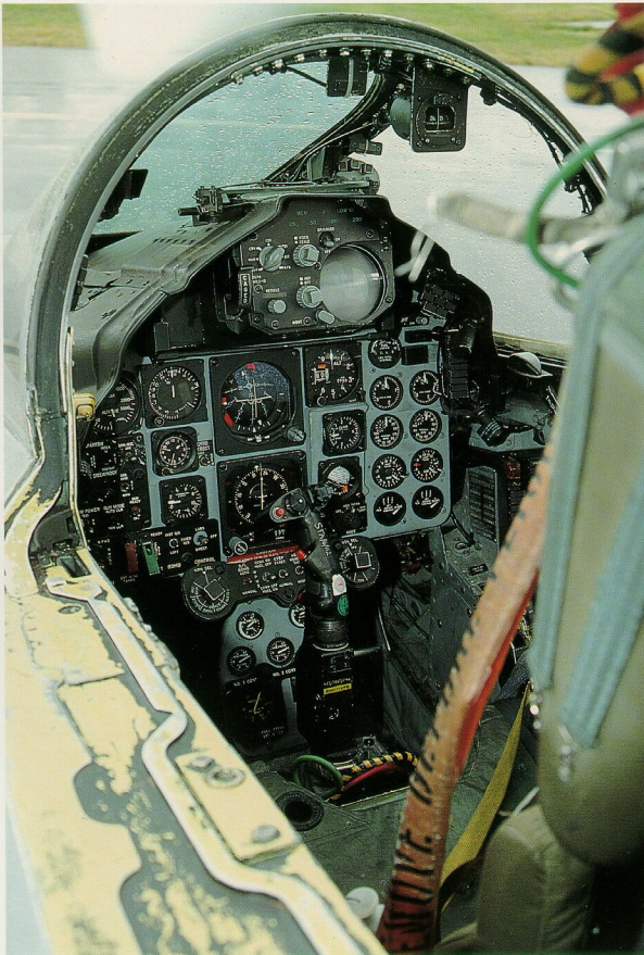
(Above) Radio call signs and checklists can be seen mounted on the canopy framing.
