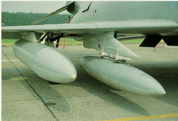
(Above) A detail seldom shown in books such as this. The fuel connecting lines and electrical wiring can clearly be seen. Note the pylon is an integral part of the fuel tank. (Left) A 308 gallon(US) tank and a travel pod are mounted on the outer wing and inboard pylon respectively on this Leuchars based FGR.2 Phantom. Note the very pointed inboard pylon with an unusual bomb rack holding the travel pod and the way the pylon is mounted to the lower wing surface.
