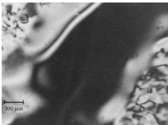
FIG. 1.23. Typical texture of an N_D phase in a 200 \mu\text{m} thick sample of a freshly prepared mixture of potassium laurate, 1-decanol, and water, in a polarizing light microscope, between crossed polarizers.
