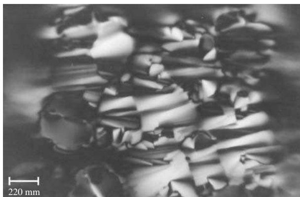
FIG. 1.35. Typical fan-like texture of a hexagonal phase for a 100 \mu\text{m} thick sample of a potassium laurate/decanol/water mixture, in a polarizing light microscope, between crossed polarizers.
