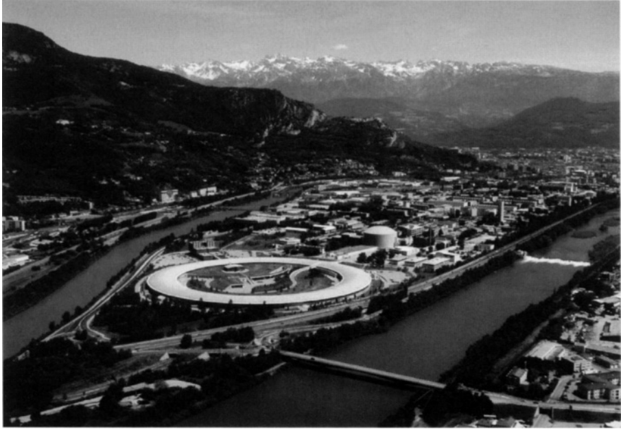
FIGURE 2.2. An aerial photograph of the European Synchrotron Radiation Facility (ESRF) in Grenoble, France. A synchrotron source consists of a ring-shaped vacuum pipe in which high-energy electrons are circulating. Radiation is produced at each location where the electron path is curved. The ESRF is one of the three hard X-ray synchrotron radiation sources of the third generation that are currently in operation. The other two are located in the USA (APS, in Argonne) and in Japan (SPring-8, in Nishi Harima). (Source: ESRF).
