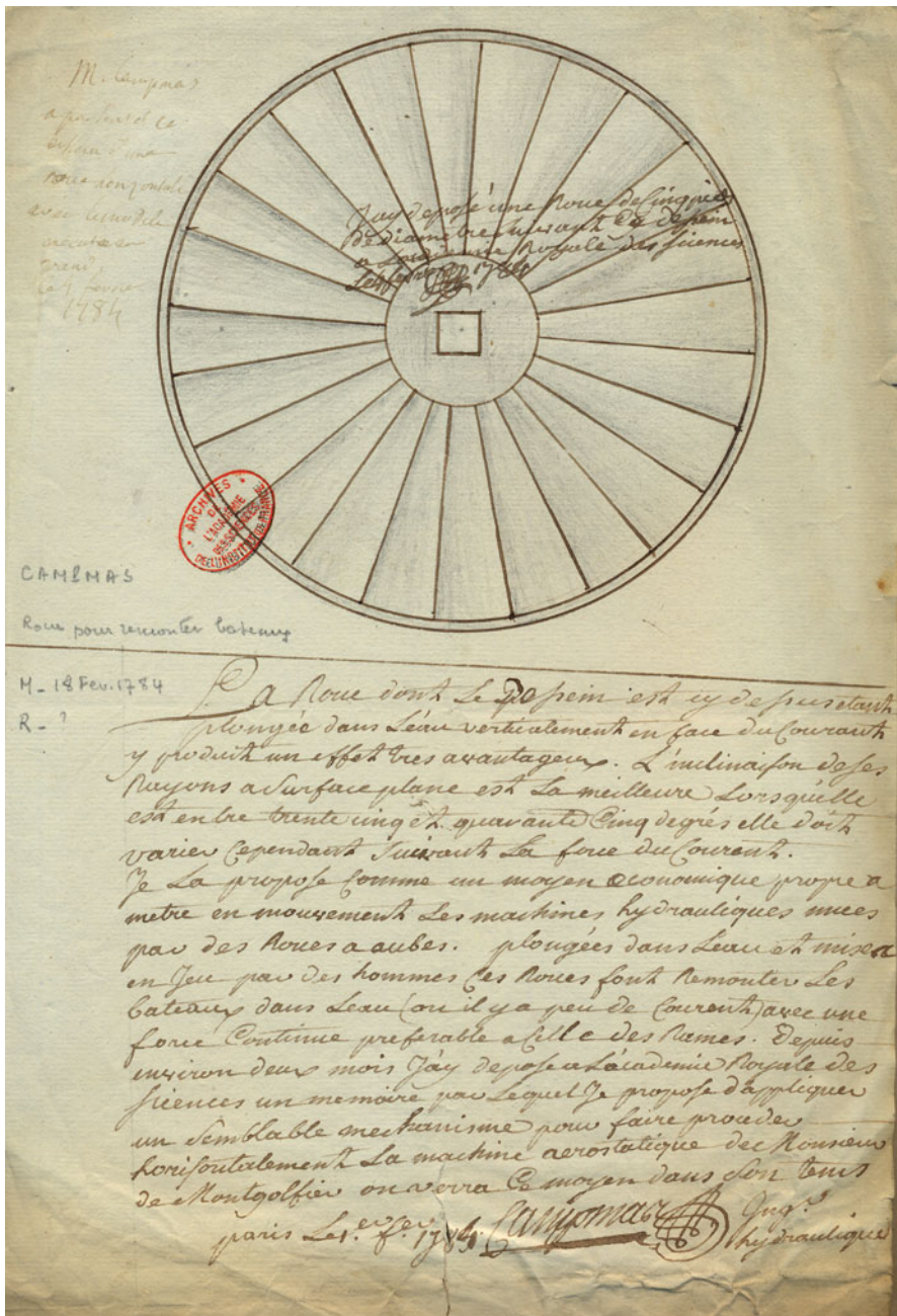
Fig. 21.5 Naval and aerial towing wheel, Feb. 4, 1784 (AAdS, pochette, Feb. 18, 1784). Top left: registration by Condorcet, same day, when Campmas presented a 5-foot model of the wheel at the Academy. Courtesy of the Academy of Sciences, Paris
