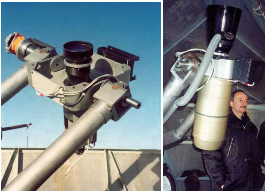
Fig. 11.47 FAVOR (FAst Variability Optical Registrator) camera - SAO RAS, operating since 2003. Built in collaboration with IPI and IKI (Moscow), from [91]
