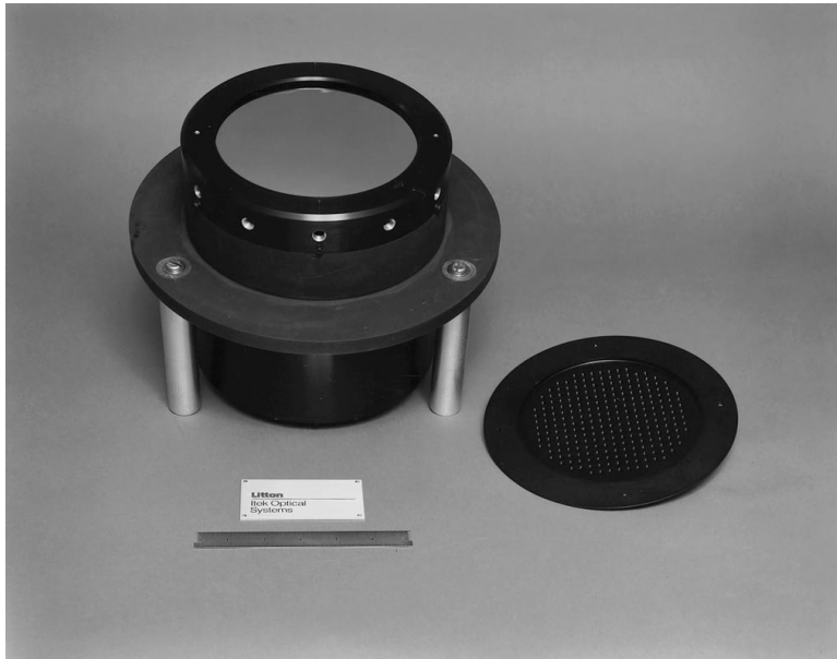
Fig. 4.6. A 341-actuator deformable mirror (SELECT) from LITTON-ITEK (Courtesy M. Ealey).
