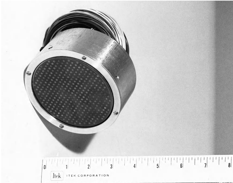
Fig. 4.5. A 345-actuator monolithic piezoelectric mirror (MPM) from ITEK (Courtesy M. Ealey).
