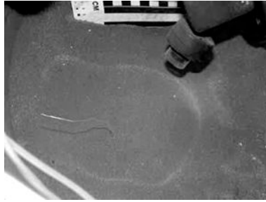
Figure 15.5 Inside a bucket in the chamber of the Andromeda planetary environmental chamber. After escape of subsurface volatiles, craters containing ponds of fine-grained material were produced.
