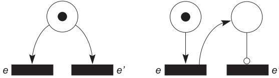
Figure 2.19. Two scenarios in which the firing of deterministic transition e causes transition e' to become disabled.
