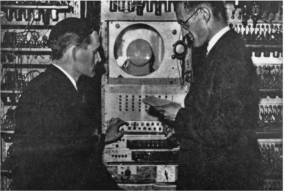
Figure 8.7. Freddie Williams (right) and Tom Kilburn in front of their tiny pioneering computer at the University of Manchester. The push-button switches were for entering the program digit by digit. The instructions were stored in the computer as patterns of dots on the surface of a cathode ray tube; this was similar in appearance to the small monitor tube in the center of the photo. School of Computer Science, University of Manchester. Reproduced with permission.
