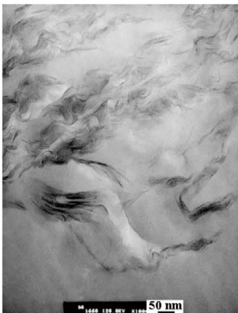
Figure 3.13 TEM image of SbC16 PS nanocomposite (scale bar 50 nm). Reproduced from [57] with permission.
