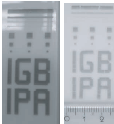
Fig. 15. Cobalt blue pigment before (left) and after the baking step at 1100°C (right).
