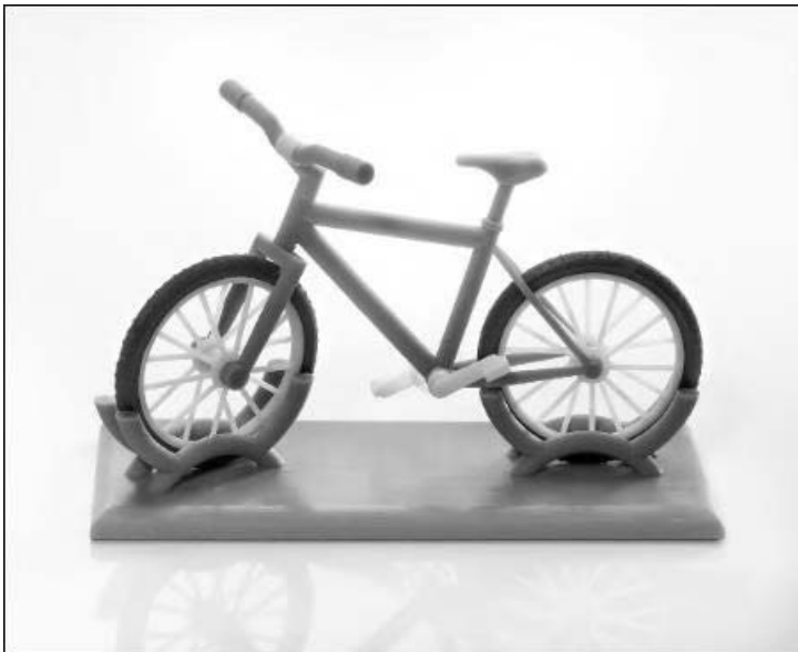
Fig. 3. Inkjet 3D model of a bicycle. The model was built by PolyJet Matrix technology, in a single printing process by the simultaneous use of several Digital Materials .
