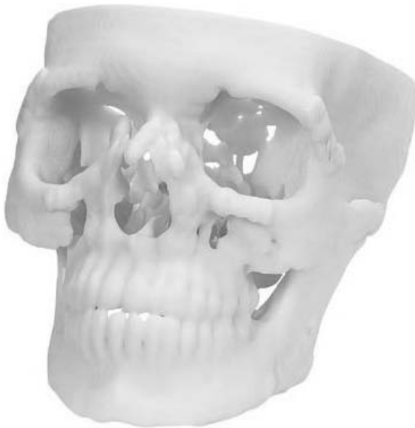
Fig. 1. Human skull as an example of an anatomic model built by PolyJet 3D Printing.
