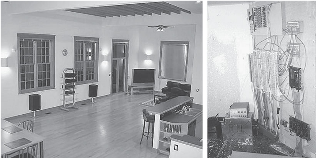
Figure 16.3. Michael Mozer's adaptive house. An interior photo of the great room is shown on the left. On the right is a photo of the data collection room where sensor information terminates in a telephone punch panel and is routed to a PC. A speaker control board and a microcontroller for the lights, electric outlets, and fans are also shown here. (Photos courtesy of Michael Mozer).
