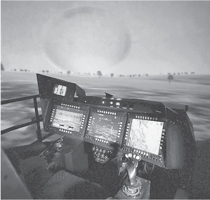
Figure 16.1. The Rotorcraft Pilot's Associate cockpit in a simulated environment. Reprinted from Knowledge-Based Systems , 12, Miller, C. A., and Hansen, M. D., The Rotorcraft Pilot's Associate: Design and evaluation of an intelligent user interface for cockpit information management , pp. 443–456, copyright 1999, with permission from Elsevier.
