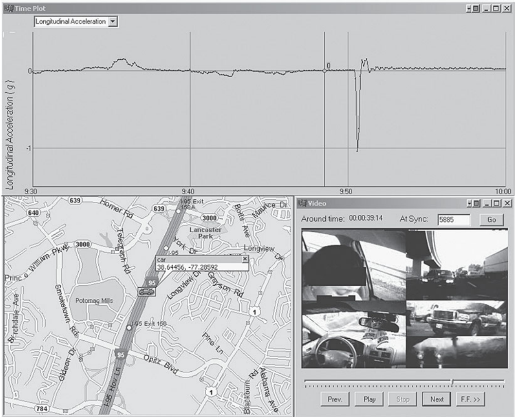
Figure 8.5. A real-life crash produces an abrupt longitudinal deceleration in the electronic record from the IV. GPS data show the exact location of the crash on the map. Corresponding video data (the quad view) show the driver was looking down (to eat a sandwich) and reacted too late to a braking lead vehicle.
