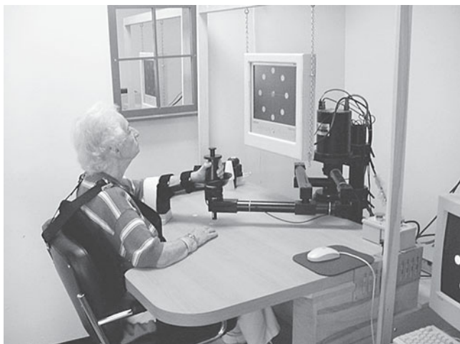
Figure 22.3. Patient using the MIT-Manus (Hogan et al., 1995; Krebs et al., 1998).
