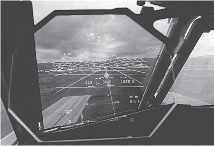
Figure 17.4. Augmented cognition. The Rockwell Collins Synthetic Vision System overlays wire-frame terrain imagery rendered from an onboard database onto a heads-up display along with guidance symbology. This improves the pilot's awareness of terrain under poor visibility conditions without obstructing the real-world view as visibility improves (courtesy of Rockwell Collins, Inc.).
