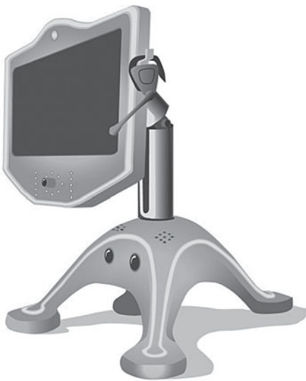
Figure 18.1. Concept drawing of the physically animated computer (left), and a mechanical prototype (right). RoCo can move its monitor “head” and its mechanical “neck” using 5 degrees of freedom. There are two axes of rotation at the head, an elbow joint, and a swivel and a lean degree of freedom at the base. It does not have explicit facial features, but this does not preclude the ability to display these graphically on the LCD screen.
