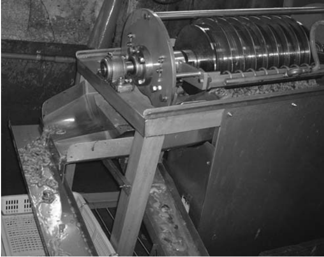
Figure 23.2. Scallop mantle separating machine (Takahashi, 2005).
