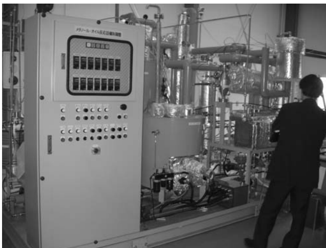
Figure 5.4 Pilot-scale reactor, which can produce 40 L of fatty acid methyl ester based on the superheated methanol vapor bubble method.
