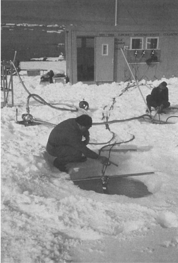
Figure 7.1. Micrometeorite “factory” used at Cap-Prudhomme during the Antarctic summer of 1993–94. The caravan hosts three steam generators that deliver jets of reheated melt ice water at \approx 70 °C that are injected into three drill holes with an initial diameter and depth of about 30 cm and 1.5 m, respectively (the water quickly reaches an equilibrium temperature of a few °C). After 8 hours of functioning, each hole has generated a pocket of melt ice water with a volume of about 3–5 m 3 . The chimney of the factory was equipped with a smoke filter that stopped all fly ashes with a size \geq 36 \mu\text{m} .
