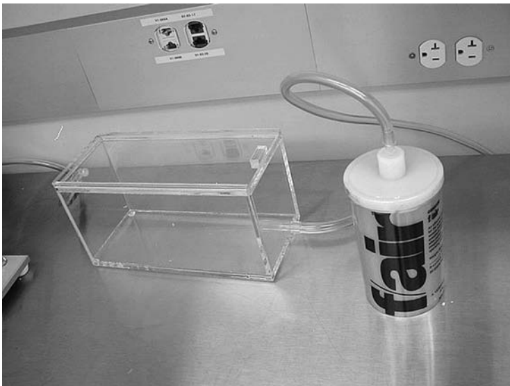
Figure 5.4. Anesthetic induction chamber in a non-rebreathing system consisting of a transparent container and equipped with two tubing connectors for introducing and exhausting the gas. (The devices are supplied from Harvard Apparatus, Cambridge, MA.)
