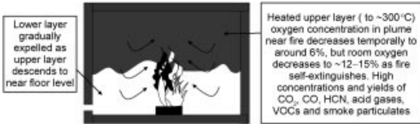
2.7 Under-ventilated (vitiating) fire in enclosed compartment.
