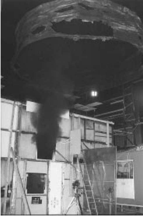
13.33 The larger storage configuration enclosure in TOXFIRE.
