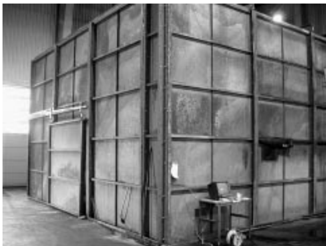
13.9 The exterior of the IMO test enclosure.
