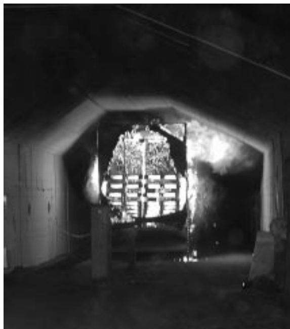
13.26 Burning load on HGV mock-up in one of the Runehamar tests.
