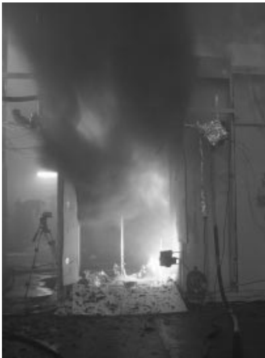
13.29 Opening of corridor instrumented with sampling probe for FTIR during full-scale cabin fire.
