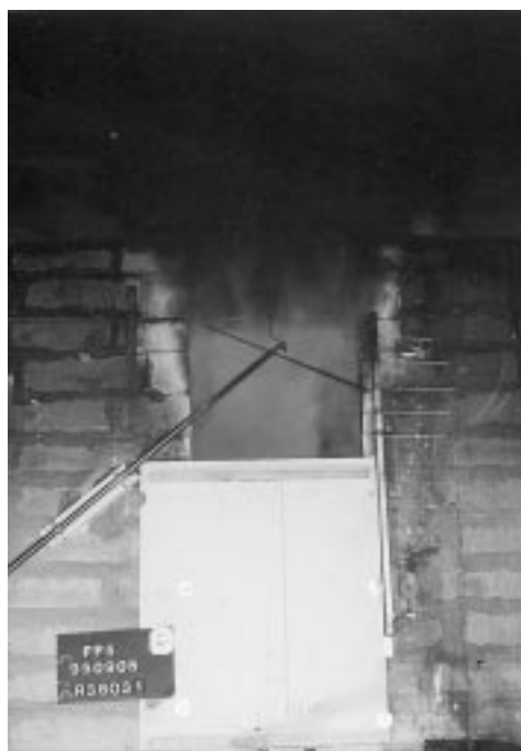
13.32 Restricted door opening of the ISO 9705 room in TOXFIRE.
