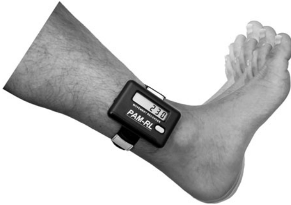
Figure 20.4 PAM-RL can record leg movements continuously for 72 hours. It can also differentiate between standing and lying using an integrated position sensor. Somnomedics®.
