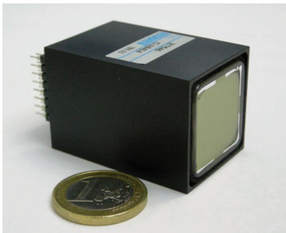
Fig. 10.1 Position-sensitive photomultiplier tube (PSPMT) Hamamatsu H7546 with 64 channels
