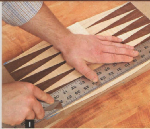
I Position a steel rule from point to point on the outermost maple triangles to cut the game-board veneer to size.
