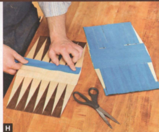
H Tape the entire surface of each game-board veneer, avoiding excessive overlaps that might cause uneven pressure during glue-up.
