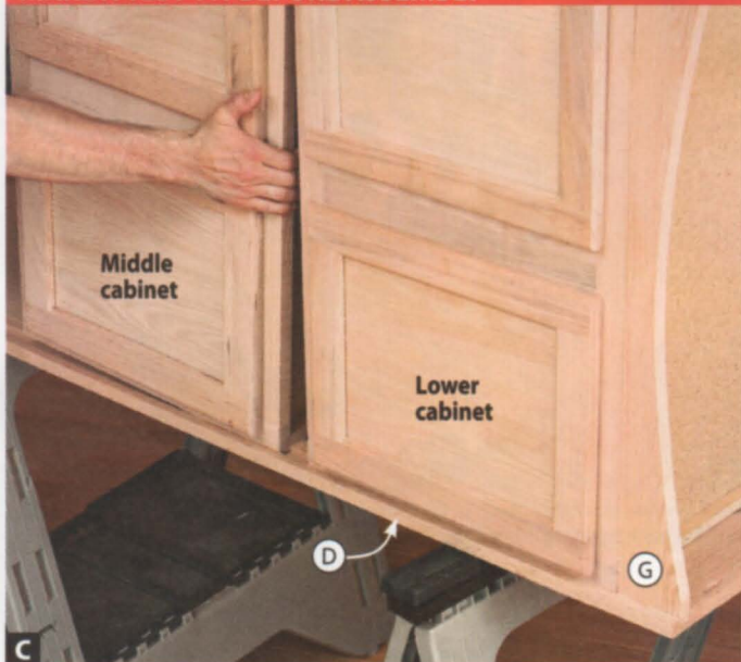
Position the front lower rail (G) and lower cabinet, then add the remaining cabinets to check their spacing along the stiles (D).
