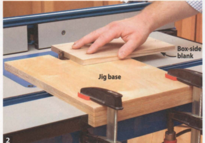
2 Clamp the jig base to your router table with the bit centered in its slot. With the box-side blank on the base, set the bit height just proud of the blank thickness.
