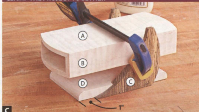
C Position the front point of the legs 1" from the front end of the base, with the drawer box centered over the base.
