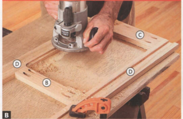
B Clamp a side assembly (A–D) to your worksurface and rout \frac{3}{8} " rabbets \frac{1}{4} " deep around each opening. Repeat for the other side assembly.
