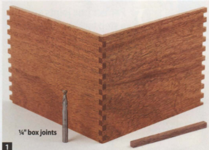
1 Choose a bit to match your box thickness to create an even joint like these \frac{1}{4} " fingers in \frac{1}{4} " stock. But don't be afraid of different bit sizes for larger joint fingers.
