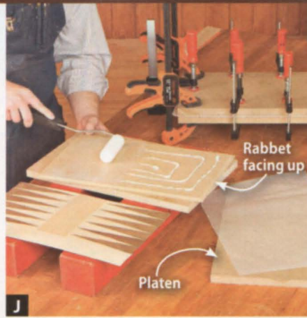
J Thin but thorough glue coverage is all that's needed for a veneer glue-up. Use plenty of clamps for even platen pressure.
