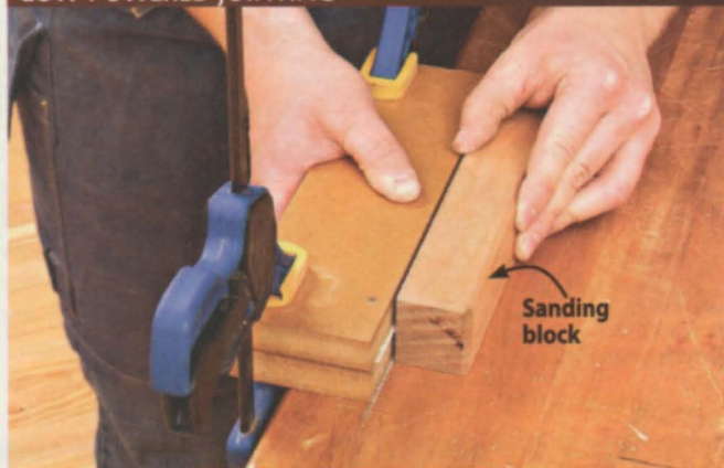
The sanding block sizes the bar to its final width, parallels the edges and joints the edge for an airtight glue line.
