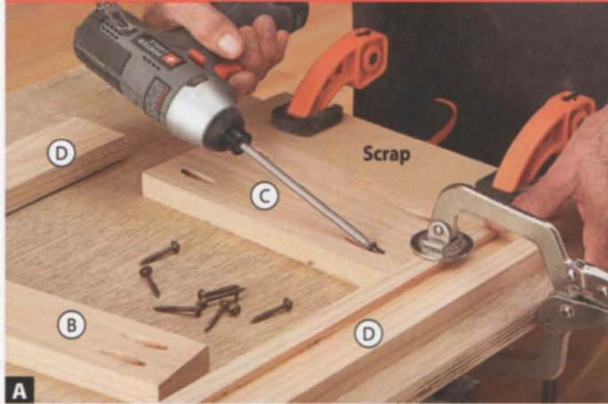
A Butt the stile (D) and lower rail (C) against a scrap to align them, then clamp the parts to your worksurface. Drive pocket screws.
