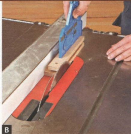
B With the wide platen against the fence, make nibbling passes on the tablesaw until the edge of the veneer stack is smooth.
