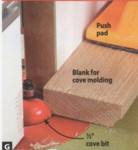
G Taking shallow passes, rout a cove profile on each edge of a wider blank. Use a push pad to keep your hands safely away from the bit.
