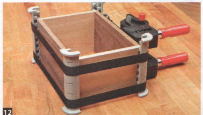
12 Rockler's box-joint-jig clamping cauls (item no. 42784, $30, rockler.com) allow you to clamp proud box joints while placing pressure squarely on the joint.
