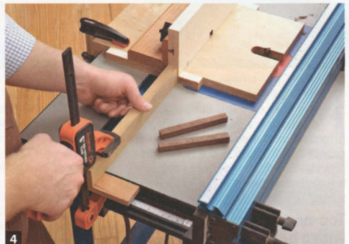
4 Create a scrapwood T-square to fix the distance from the table edge to the guide. The T-square should be tall enough to clamp in place against the guide.
