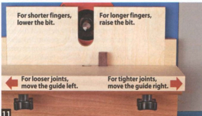
11 Test-fit the joint. It should be easily hand-assembled, but snug enough that it doesn't fall apart under its own weight. Adjust the jig if necessary, as shown.
