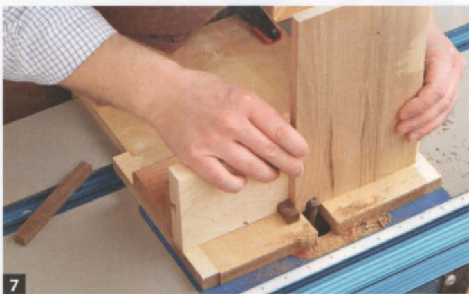
7 Test the setup by standing one test blank against the indexing pin. Slide the fence assembly forward to rout a socket through the blank.
