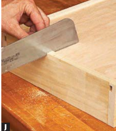
J Cut the notch for the slide at least \frac{1}{8} " wider on each side, to the depth of the drawer bottom. Then chisel out the waste.
