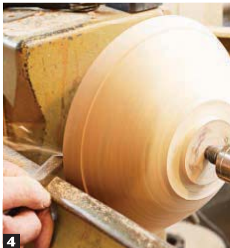
4 As you did with the green bowl, use the parting tool to define the rim. Continue cutting until you have a rim that's true around the entire bowl.
