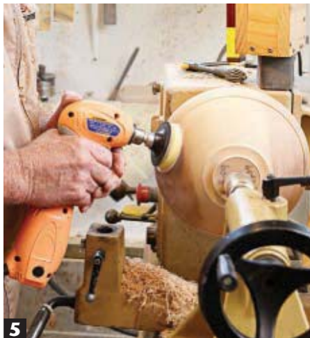
5 With the bowl's outer shape to your satisfaction, sand it smooth, beginning with 120-grit sandpaper and continuing through 320 or 400. Apply finish to the bowl's outside.
