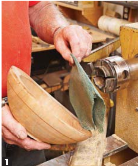
1 Mount the dried bowl by trapping it between the live center and the four-jaw chuck. Use a folded sanding pad as a buffer to add grip. Center the bowl as best you can.
