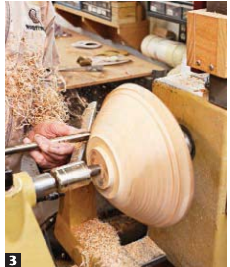
3 Turn the outer surface of the bowl to make it round again. Place the gouge's bevel against the wood near the foot and push-cut toward the rim. Use ultralight cuts to finish the shape.
