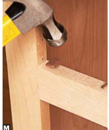
M Glide pads not only prevent the drawer from rocking on a single slide, but they also make for smoother operation.
