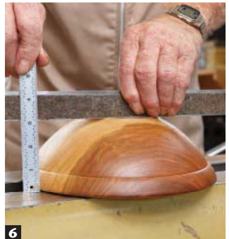
6 Before tackling the inner shape, measure the bowl's depth from rim to foot. This lets you know how much material to remove without cutting through the bottom.
