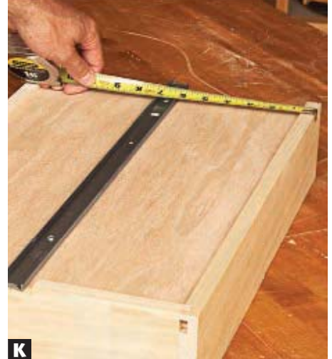
K With one screw holding the front of the slide in place, measure from the drawer side to make sure the slide sits centered and parallel.
