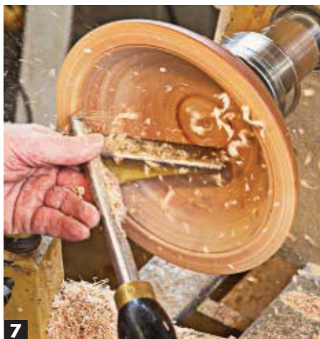
4 As you did with the green bowl, use the parting tool to define the rim. Continue cutting until you have a rim that's true around the entire bowl.
