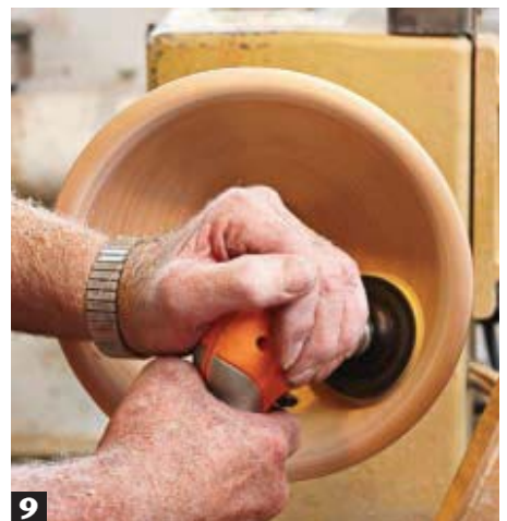
6 Before tackling the inner shape, measure the bowl's depth from rim to foot. This lets you know how much material to remove without cutting through the bottom.
