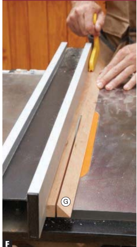
F Cut a shelf support (G) for the other case from the same blank by setting the blade back to 90° and ripping the piece to size.
