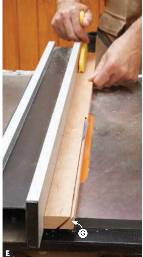
E Tilt your tablesaw blade to 45° and bevel-rip a shelf support (G) from one edge of an oversize blank.
