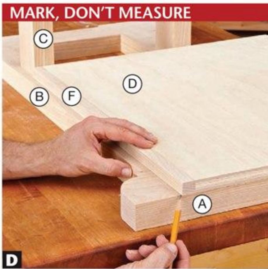
D Rest the edged side panels (D/F) against the stretchers (C) and mark their final length at the tops of the rails (A).
