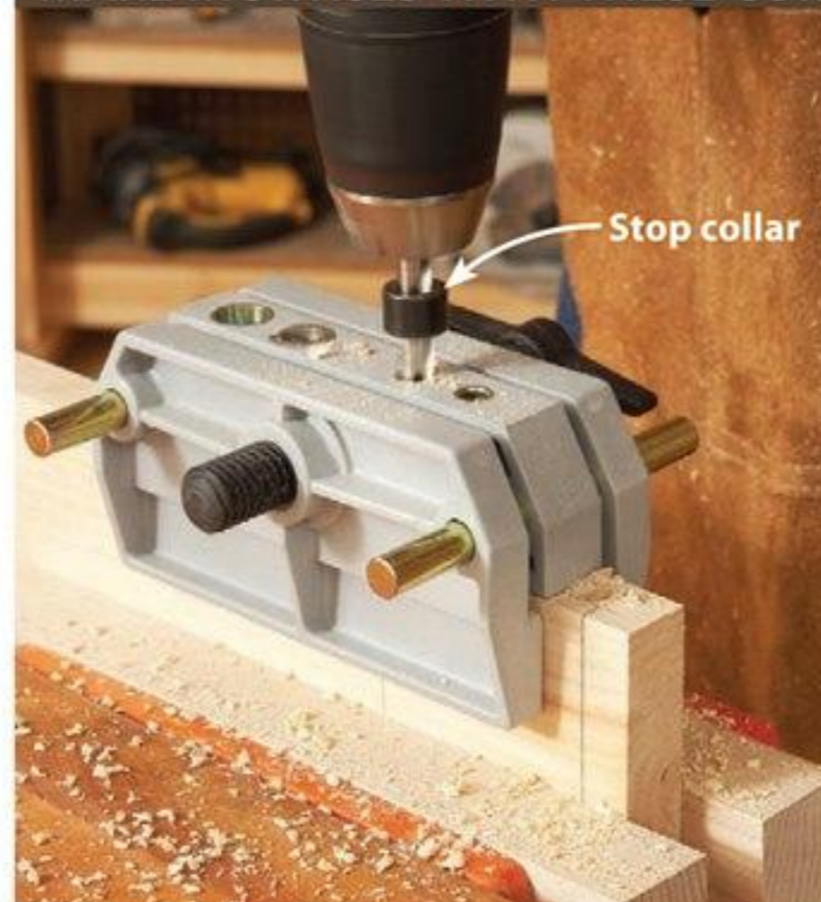
Install a stop collar on the drill bit to limit the hole depth. If you don't have a stop collar, use a masking-tape flag.
