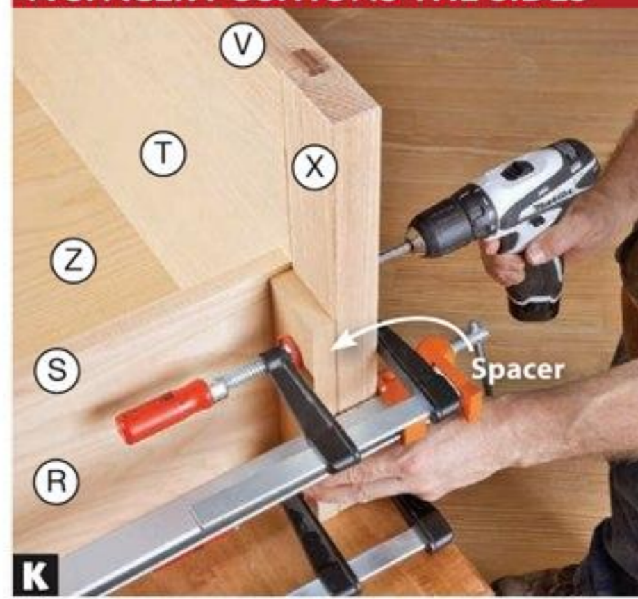
K A spacer as wide as the side trim (X) provides a solid registration surface for aligning the sides (R/S) while driving the screws.
