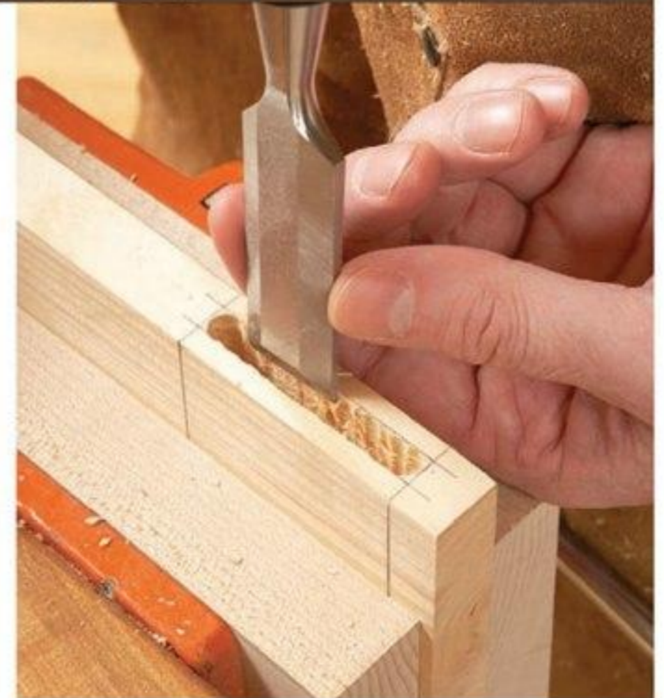
Hold the chisel 90° to the board edge and make light cuts down the mortise walls. A sharp chisel won't need a mallet.
