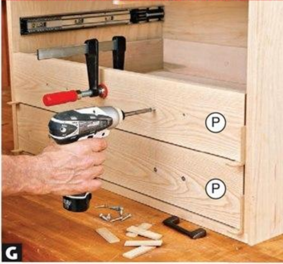
G Drive #8×1" screws through the drawer-pull holes to temporarily hold the false fronts (P, Q) to the drawer boxes.
