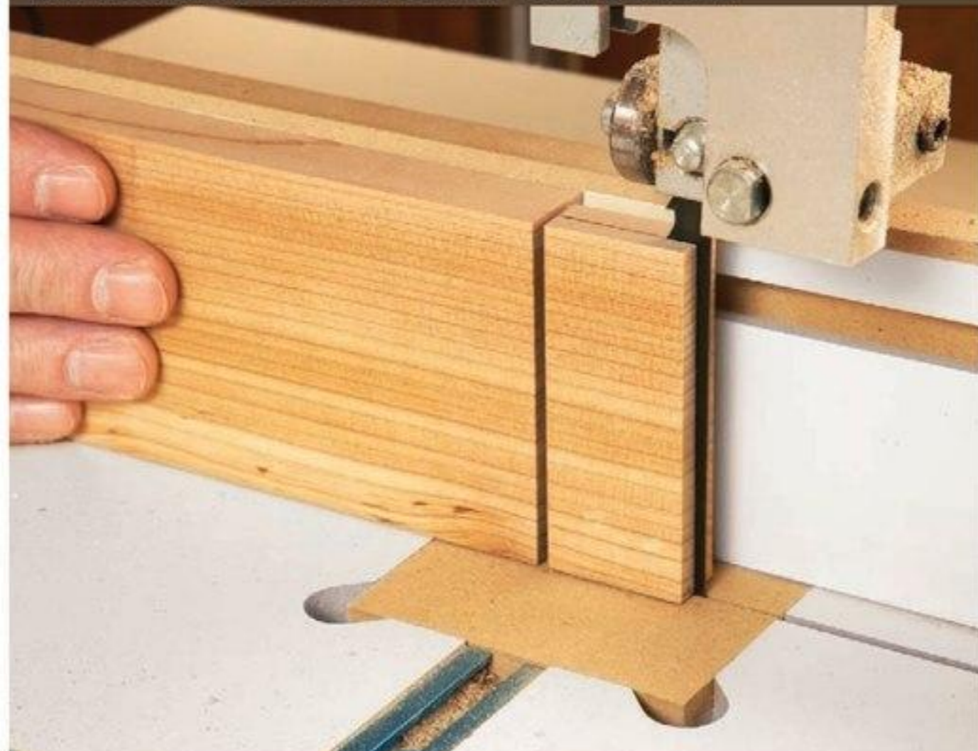
Feed stock slowly and use a 3-teeth-per-inch \frac{1}{2} " blade when cutting tenon cheeks on a bandsaw to get the best cut quality.
