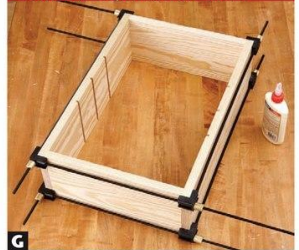
G Normally used for frame glue-ups, these four-way clamps can also be used in pairs for boxes. The corners help square the assembly.
