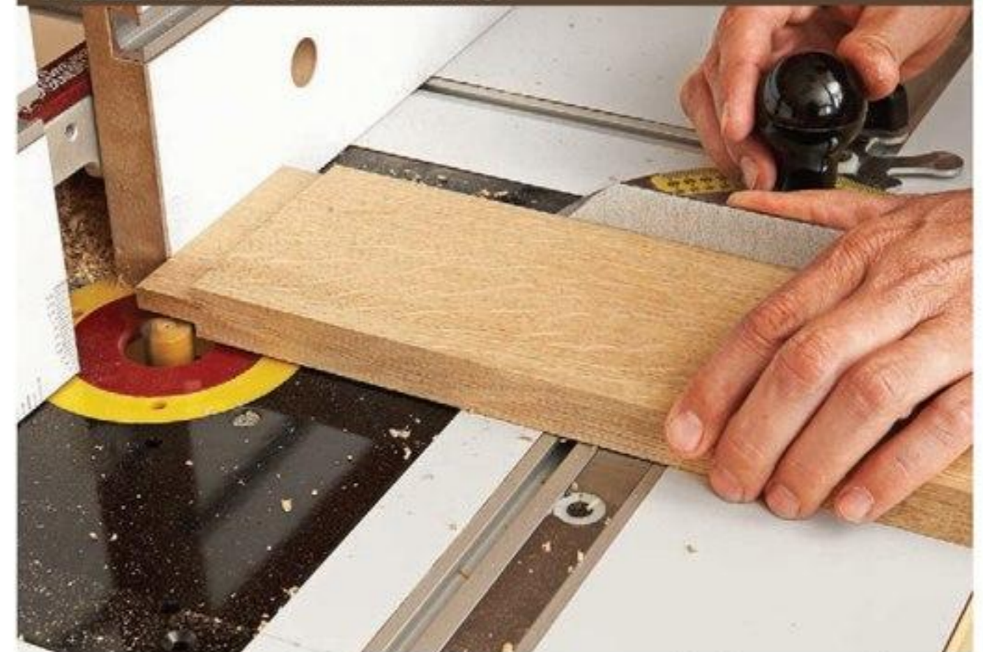
Leave a slight opening between your router-table fence panels so your shop vacuum can suck away the chips.
