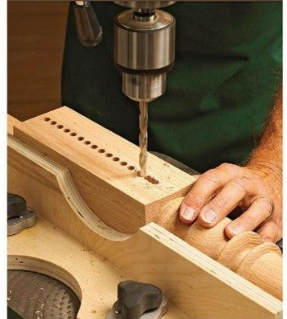
The space left between holes provides a firm starting point for the drill bit as you bore out the remaining waste.
