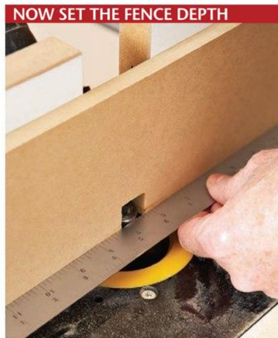
Align the auxiliary fence and the bit's bearing using a steel rule or other reliable straightedge to set the full depth of cut.
