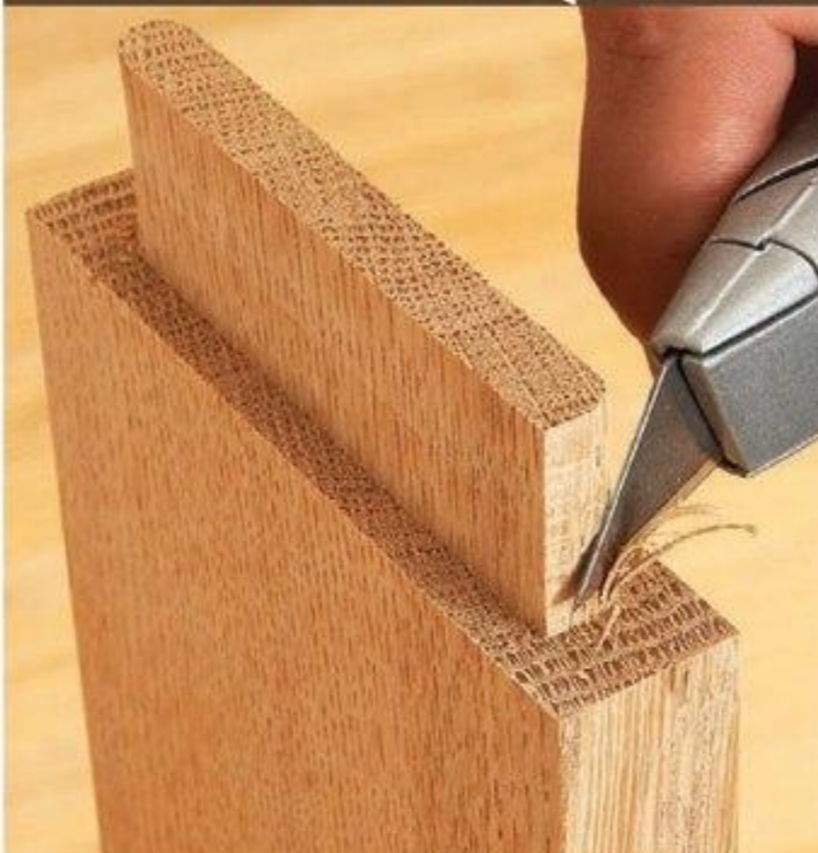
Fitting an integral tenon to a rounded mortise is easier than squaring the mortise. Use a utility knife or rasp to round corners.
