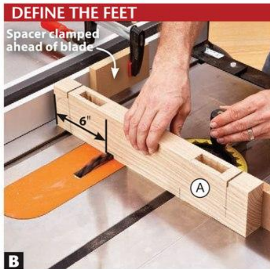
B To prevent the foot (A) from chattering along the rip fence, a spacer clamped to the fence creates space, allowing the foot to slide freely.
