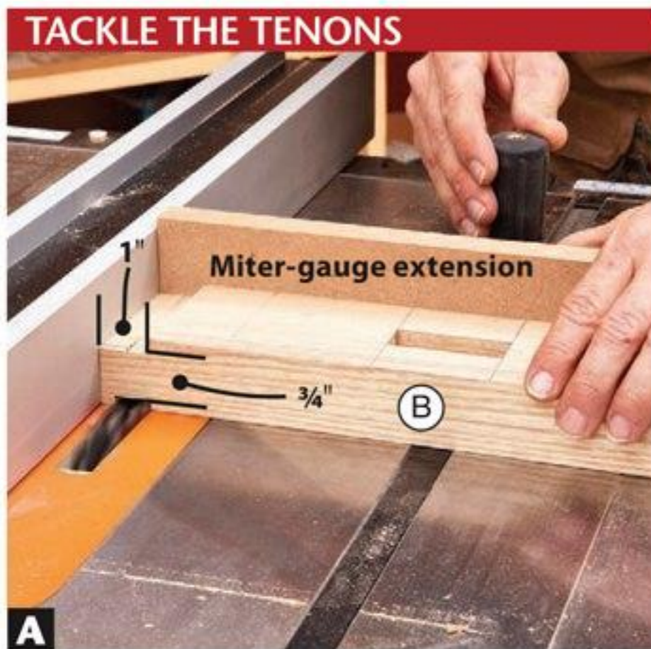
A With a \frac{3}{4} " dado blade set \frac{3}{8} " above the table, cut a test tenon on scrap. Then cut tenons on the uprights (B) and stretchers (C).
