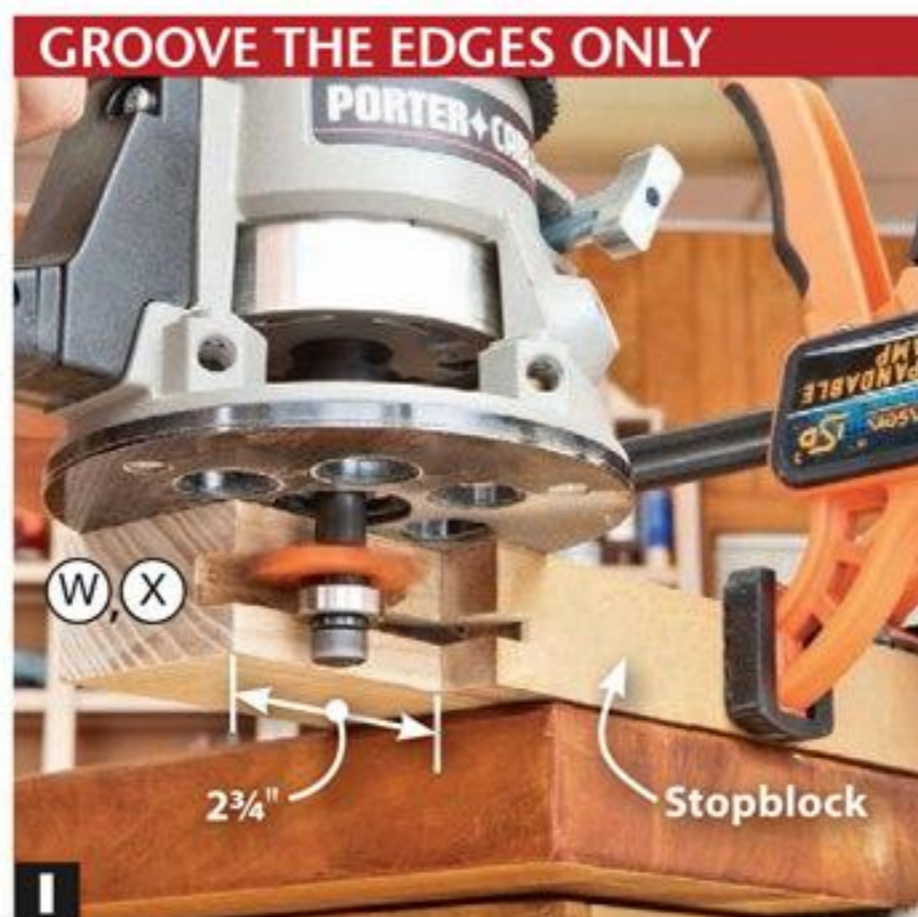
I When routing the side trim (W, X), rout only the edge, not around the end. The curved end of the groove is covered after assembly.
