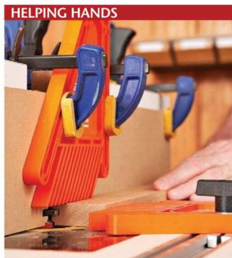
Clamp on a feather board to hold the workpiece tightly against the table and another to keep it pressed against the fence.
