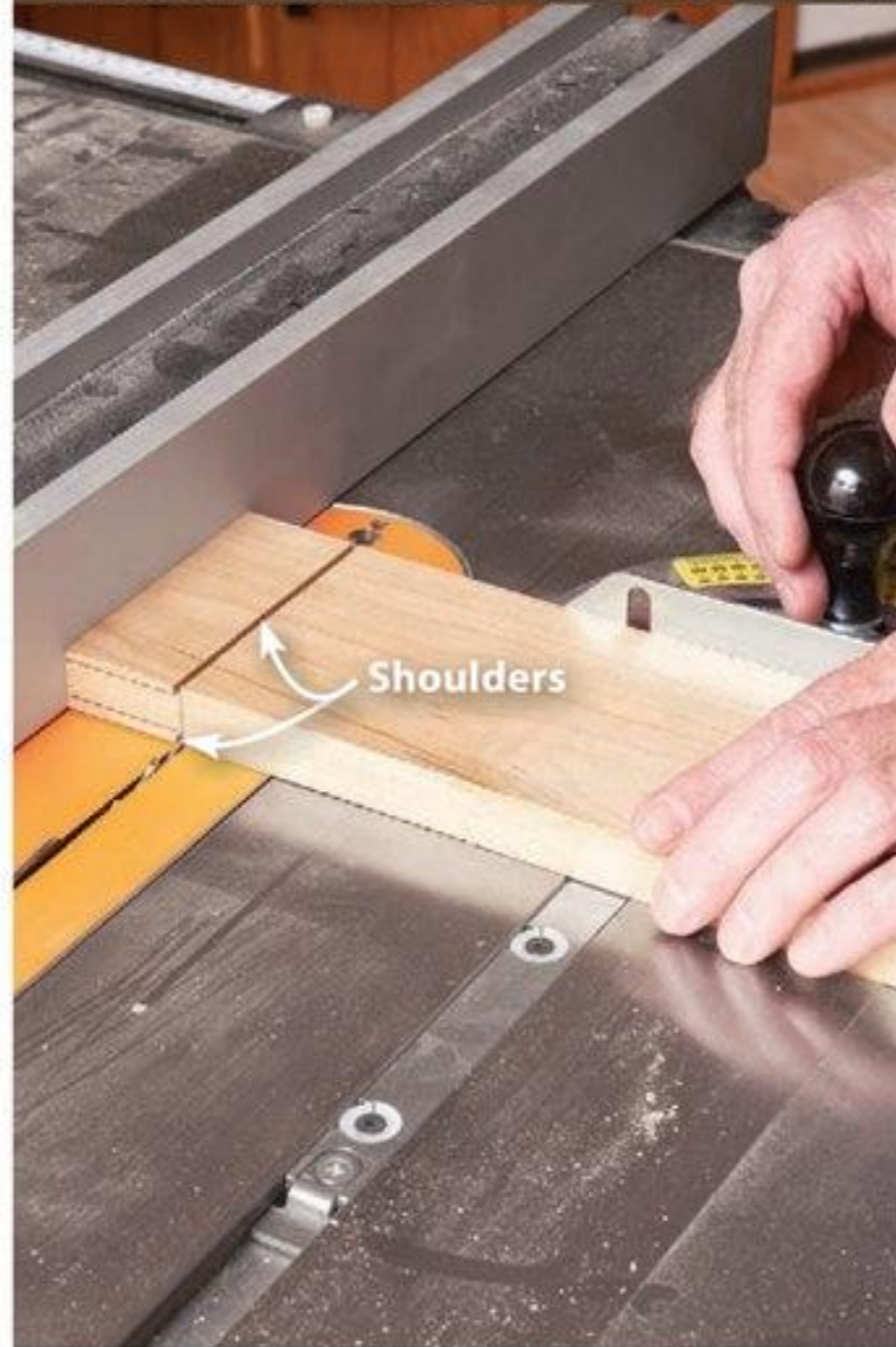
Make the tenon-shoulder cuts first, holding the workpiece square with your miter gauge and using the fence as a stopblock.
