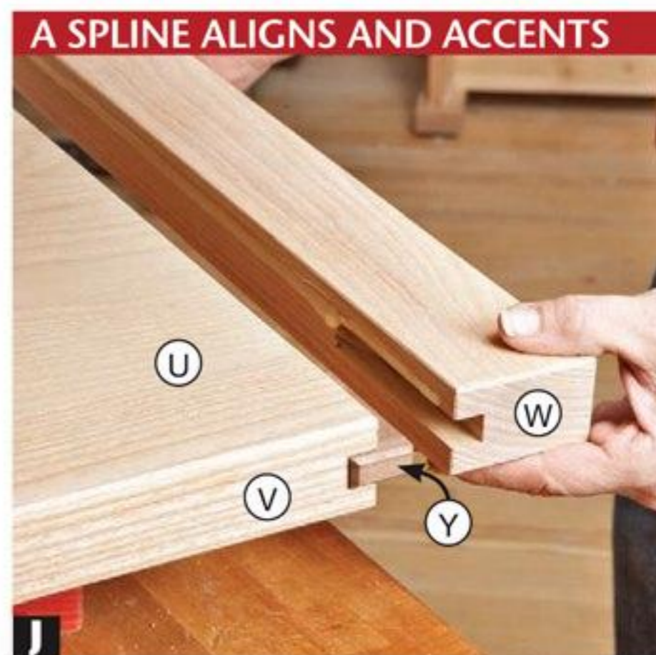
J Glue and clamp splines (Y) into the slots of the front trim (V), then glue and clamp the side trims (W or X) to this assembly.
