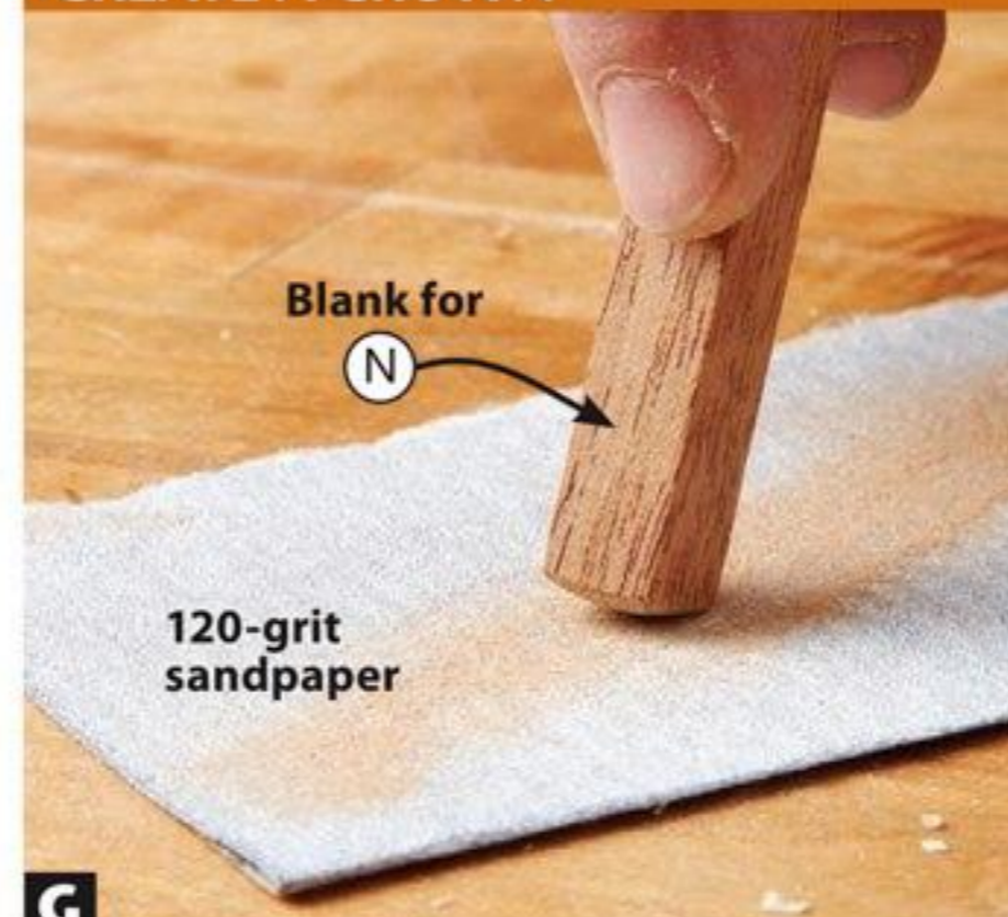
G Slightly round the end of the plug (N) blank on 120-grit sandpaper. Sand all four faces to create an even crown.
