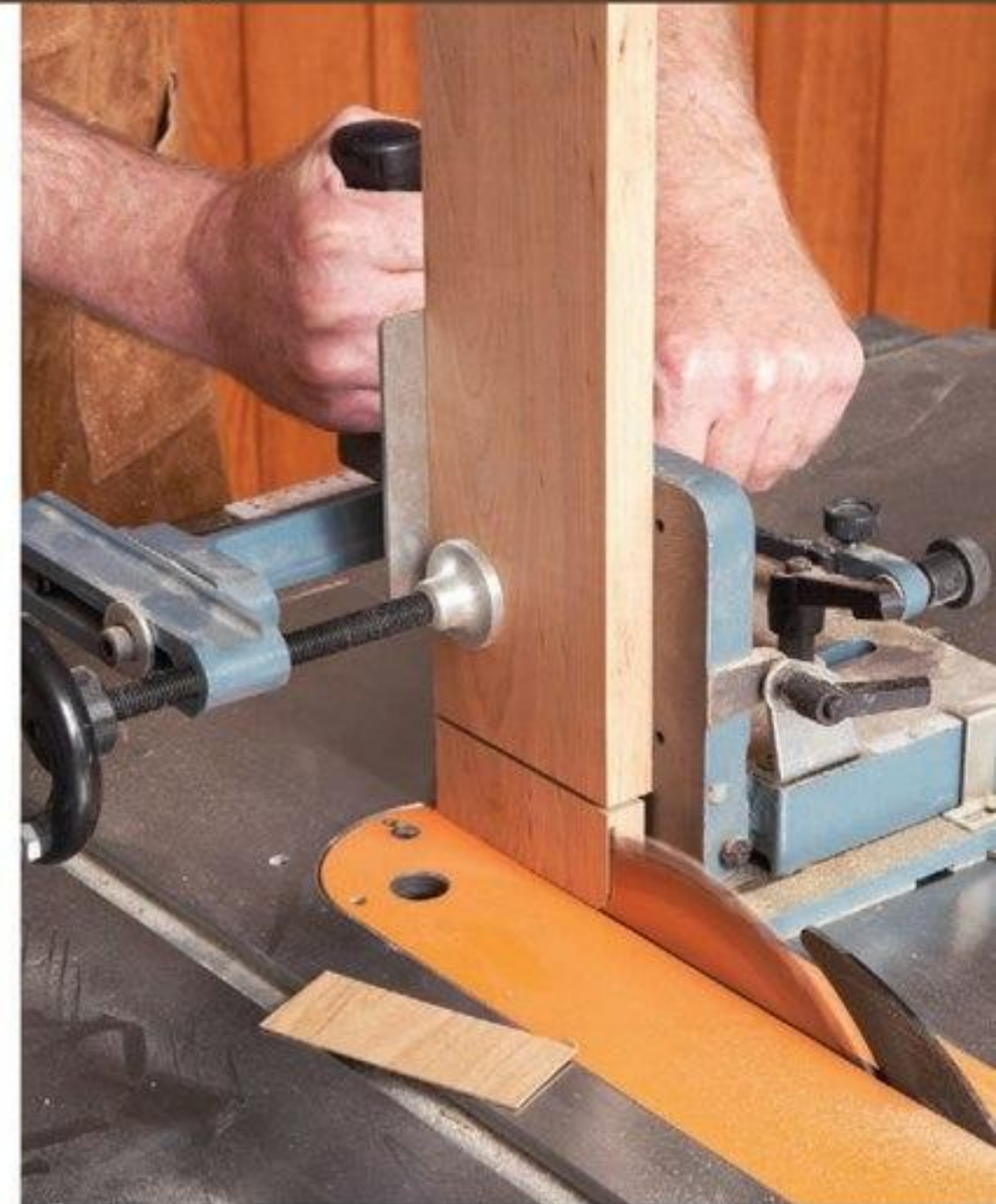
Set your tenoning jig so the tenon-cheek offcut falls away from the blade, not trapped between the blade and jig.
