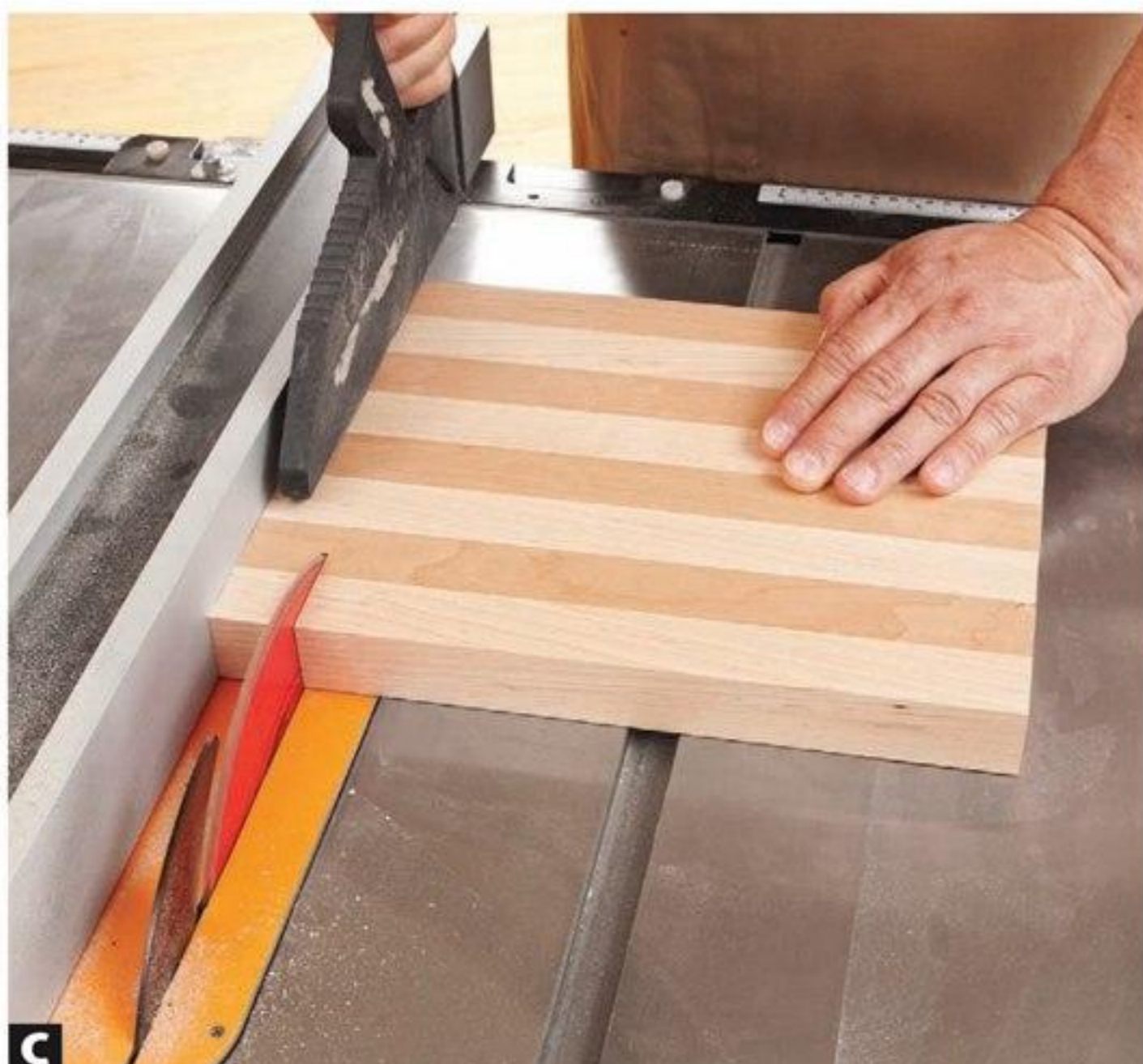
A START SQUARE TO FINISH SQUARE Use a jointer to ensure a dead-on 90-degree angle on each strip. Even a minute angular error multiplies in a butcher block.
