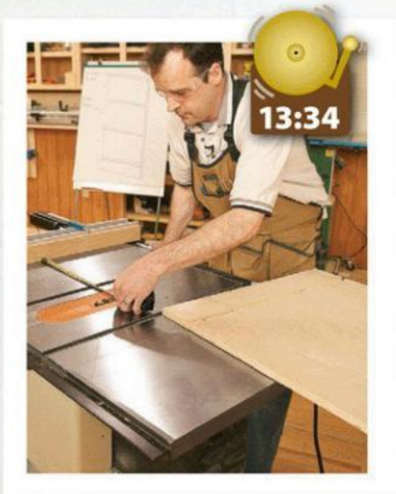
Because the stacked dado set and auxiliary fence nullify the fence scale, Kevin uses a measuring tape to set the rip fence to the correct position for the third dado.
