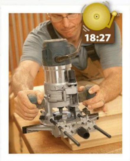
Jeff routs the first of the two \frac{1}{4} " back rabbets. Job completed at 19:44.
