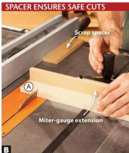
B Because of the open area between the blade and fence created by the spacer, the blocks (A) fall away from the blade after being cut.
