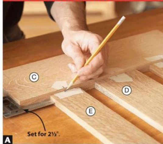
A Set a square to check the outside slat (E) offsets from the rail (B, C) ends. Align inner-slat (D) center marks with the rail centers.
