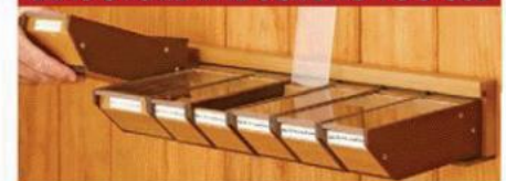
Put this on your to-do list: Removable shop-made bins keep your most popular fasteners organized, dust-free, and accessible.
