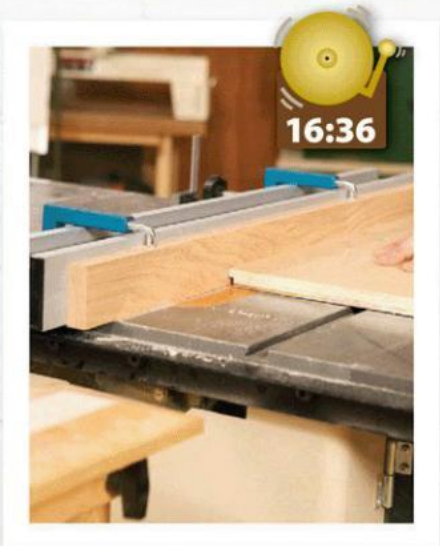
After setting the auxiliary fence over the blade and making a relief cut—something he did not do for the first rabbet—Kevin makes his final cuts, the two back rabbets. Job completed at 19:16.
