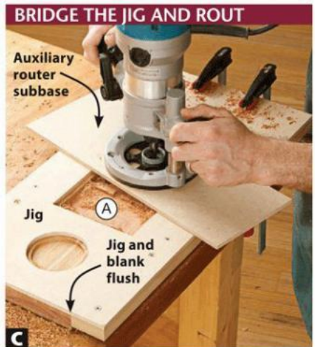
The auxiliary base spans the jig, keeping the router from tipping into the recesses as it works. Rout slowly to avoid tear-out.
