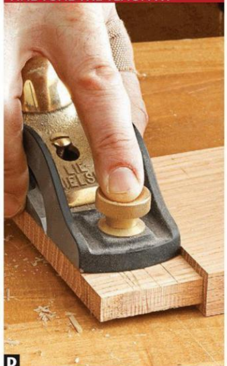
D To fine-tune a tenon with a rabbet block plane, shave away equal amounts on both faces. Check the fit after every two passes.
