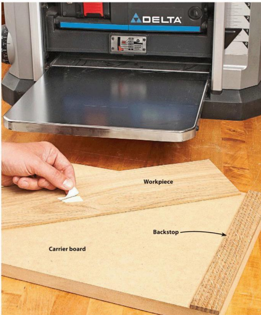
The backstop prevents slipping, while the planer's rollers hold the workpiece against the carrier board. All that's needed is a small piece of tape to prevent side-to-side motion.
