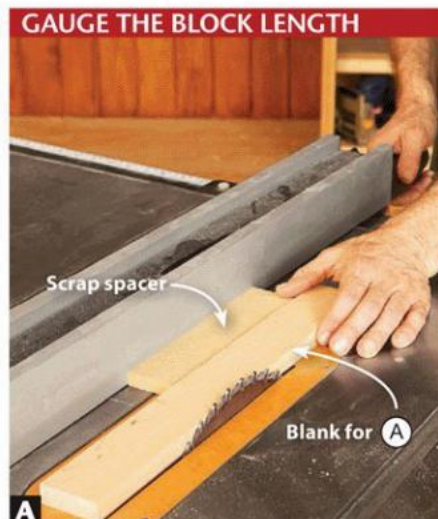
A Cut perfectly square blocks (A) without measuring by using the blank as a gauge when setting the rip fence and spacer.
