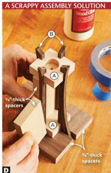
D Spacers below the lower block (A) set it at the proper height. Spacers between the legs (B) position the upper block. Clamp with tape.
