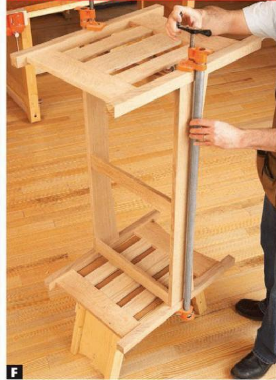
F Elevating the bottom side assembly provides clamp clearance. After clamping, rest all four legs on a level surface and check for square.
