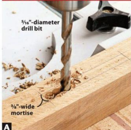
A Overlapping holes drilled with a brad-point drill bit should leave evenly spaced scallops and rounded corners.
