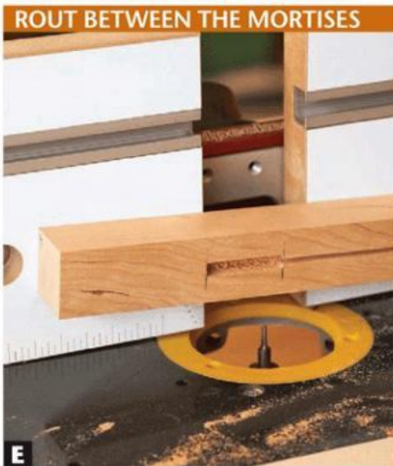
E Begin the groove by dropping the mortise over the straight bit. Stop when the bit reaches the opposite mortise.
