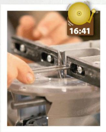
After removing the guide bushing and installing the router's edge guide accessory, Jeff sets the bit's cutting depth for the \frac{1}{4} " back rabbet.
