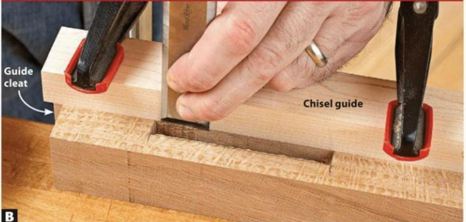
B Glue a guide cleat to your chisel guide so the guide edge aligns with the marked mortise edge. The guide holds the chisel 90° to the workpiece and prevents cutting outside the layout lines.
