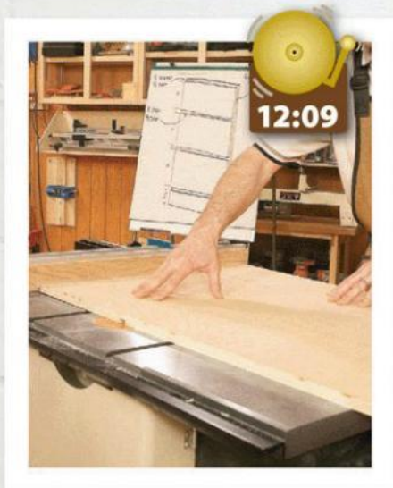
After resetting the rip fence, Kevin cuts his first dado, second cut overall.
