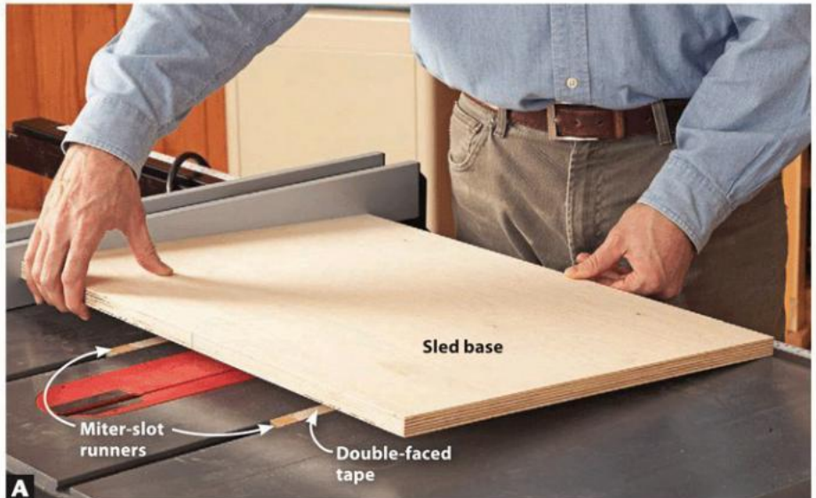
A Attach double-faced tape to the miter-slot runners and align them with the front edge of the saw table. Press one edge of the sled base against the rip fence as you tilt the sled down against the table and press it against the miter-slot runners.
