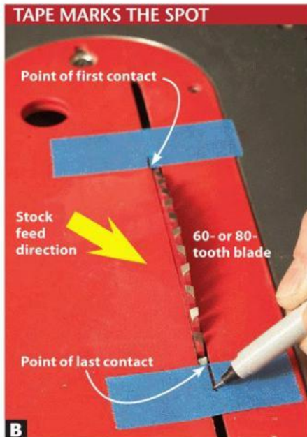
B Mark on the tape where the stock will first contact the front tooth of the blade and where it will last contact the rear tooth.
