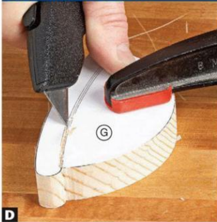
D Carve a \frac{1}{16} "-deep V-groove by carefully cutting along the pattern lines. Deepen the groove with successive cuts if needed.
