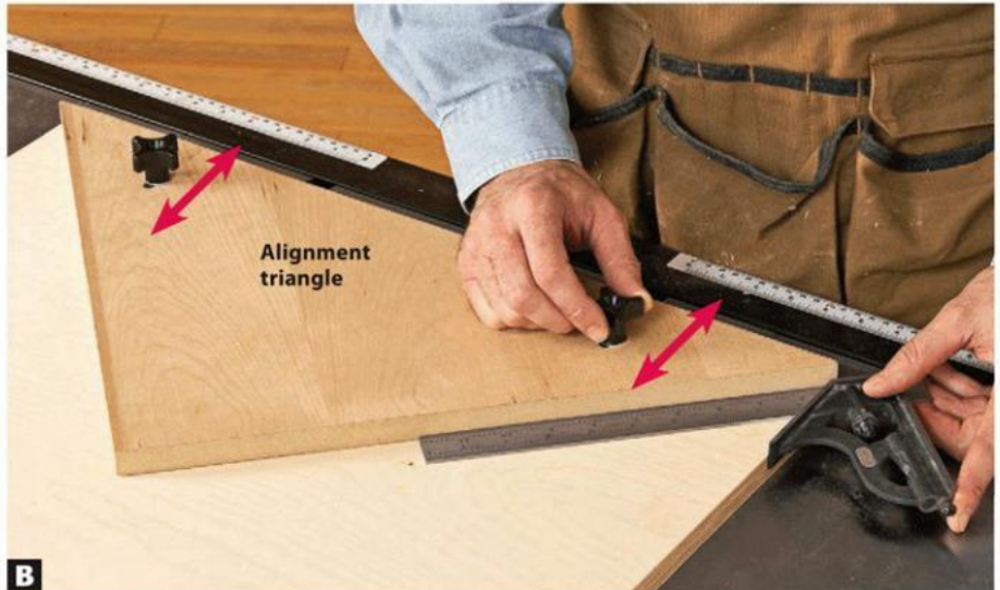
B Press your combination square against the edge of the sled base and move the alignment triangle up or down until the edge rests tight against the square. Do the same on the other side. Then secure the alignment triangle in place by tightening the knobs.
