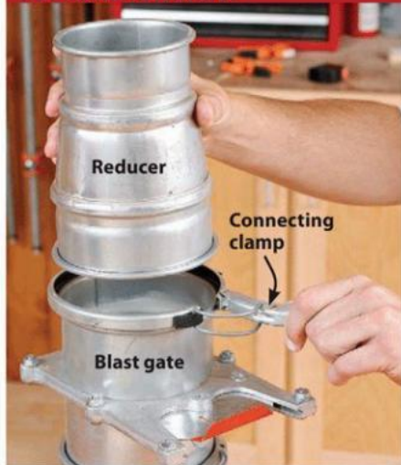
This reducer connects to corrugated hose or narrower duct. Connecting clamps let you reconfigure this type of metal duct.
