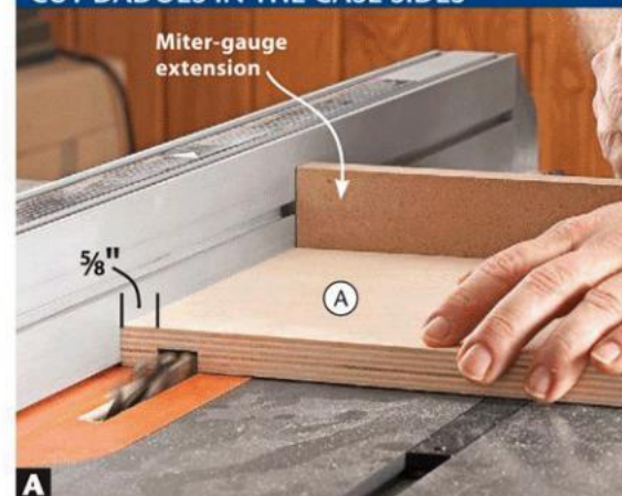
A To prevent tear-out, back up dados cut in the sides (A) with a miter-gauge extension.
