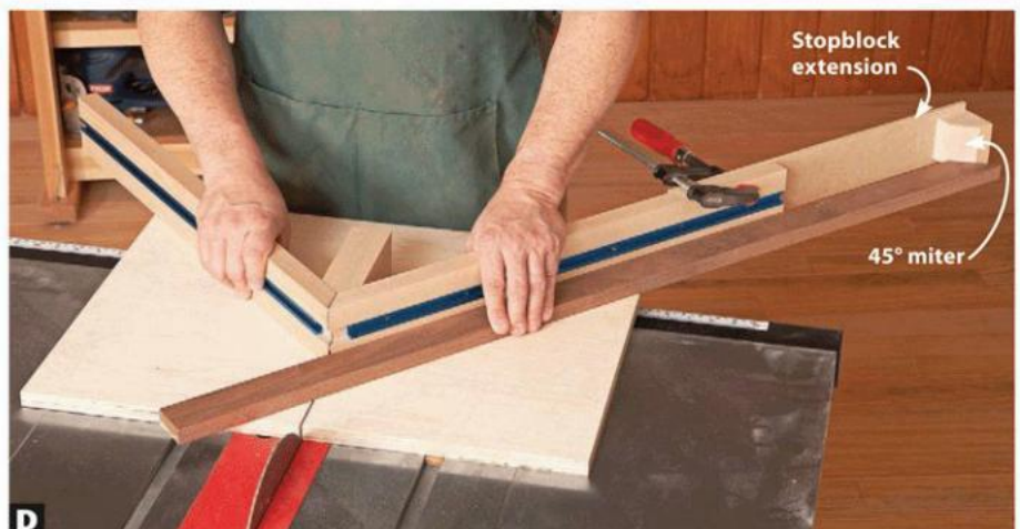
For workpieces longer than your miter fences, cut them to identical lengths using a stopblock extension. Make the stopblock 2" thick so that the mitered end of your workpiece can touch the mitered end of the stopblock.
