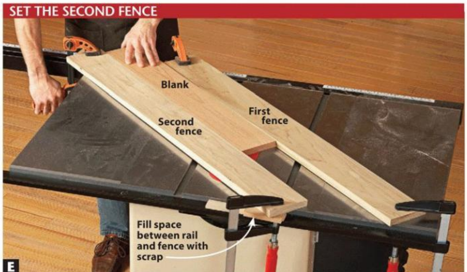
E Place a molding blank against the first fence to position the second fence. The blank must slide between the fences without binding.
