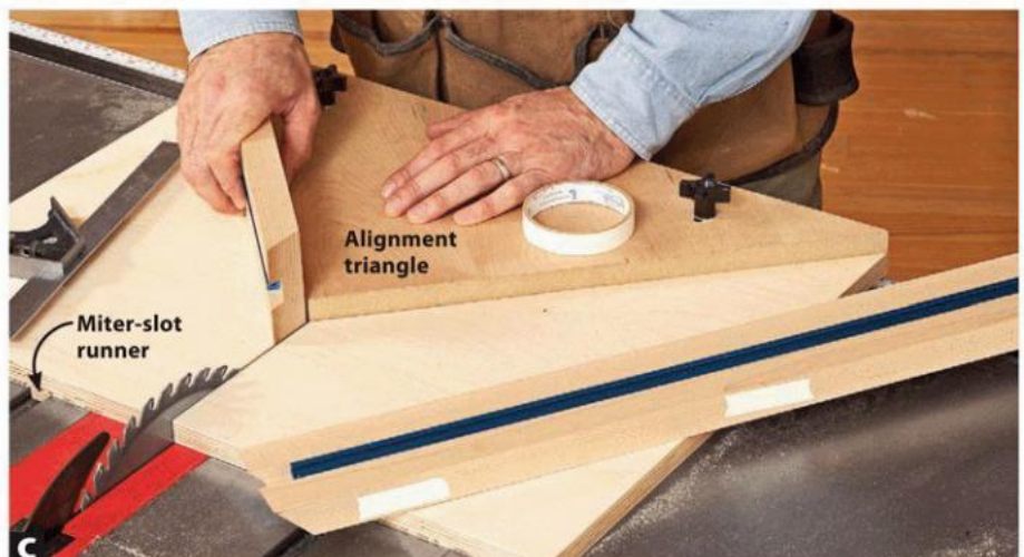
Double-faced tape holds the miter fences in position while you check their alignment by cutting test pieces to make a frame. The tip of the fence overlaps slightly less than half of the saw kerf in the sled base, with the T-track recessed 1" from the end.
