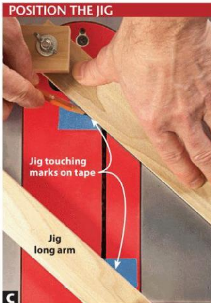
C Align the jig so the inside edges of the long arms touch the marks on the tape. Mark one long inside edge of the jig onto the saw table.
