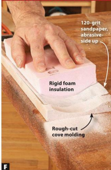
F Place sandpaper in the cove and rub a block of foam insulation across it to make a sanding block that perfectly matches the profile.
