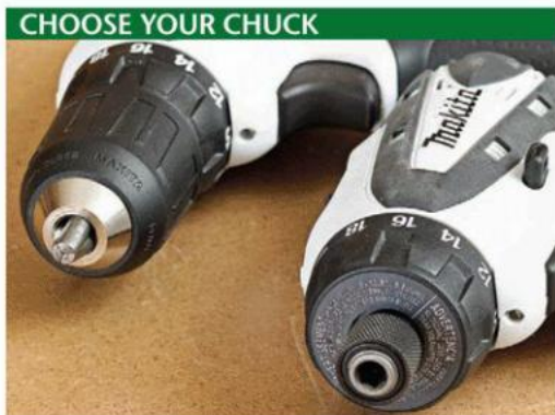
Drivers with a 3/8" three-jaw chuck (left) work with hex- and round-shank bits. Models with a hex chuck (right) accept only bits with 1/4" hex shanks.
