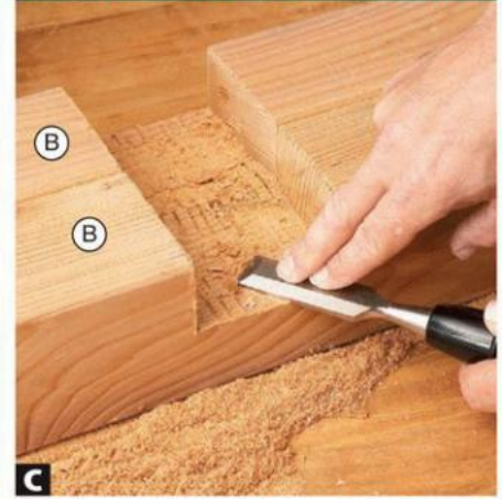
C After breaking off most of the waste between kerfs, press the flat face of a chisel against the dado bottom and shave it flat.
