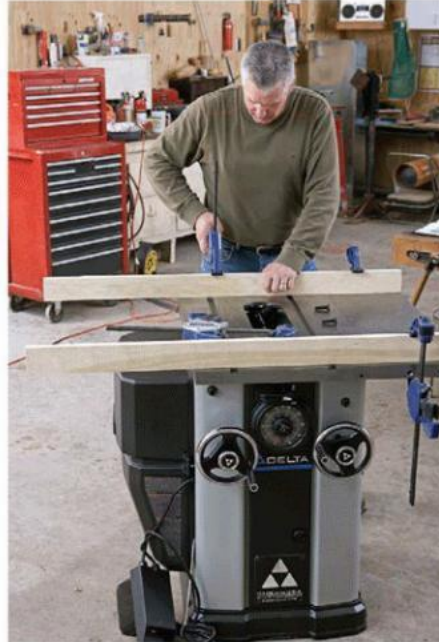
2. Holding the wing loosely aligned front to back with the table edges, clamp the boards tightly to the main tabletop.
