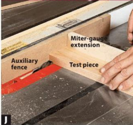
J House a \frac{1}{16} "-wide dado blade in an auxiliary fence and raise the blade \frac{3}{16} " above the table. Cut rabbets on each face of a test piece.
