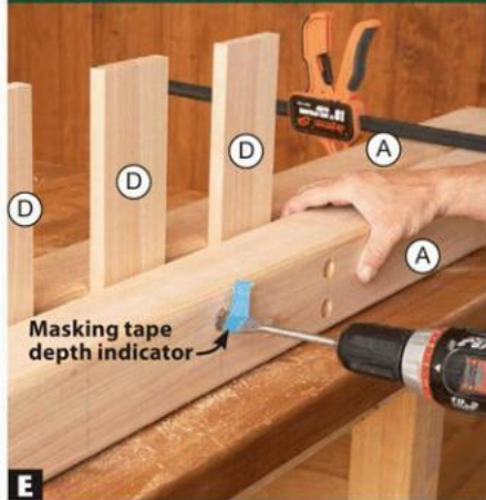
E Attach a depth indicator \frac{3}{8} " from the cutting edge of a \frac{3}{4} " spade bit and counterbore the inside seat slat (A) for the lag-screw heads.
