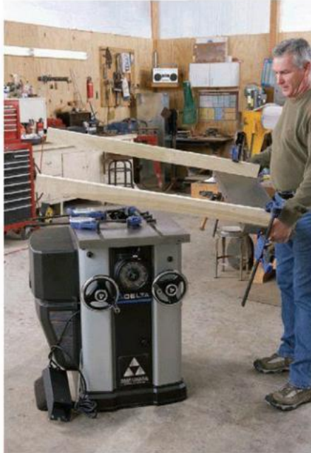
1. Clamp two straight boards about 3' long to one of the cast-iron extension wings. Extend the boards over the main tabletop.
