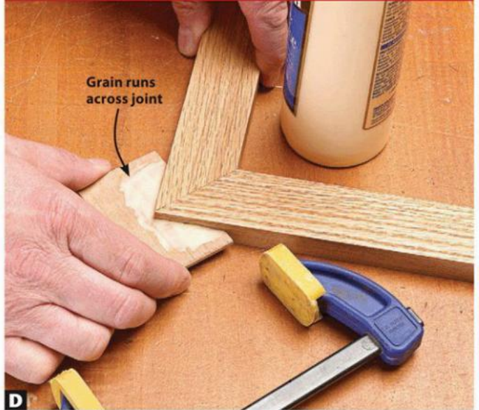
D Apply glue to both sides of the spline, and slide it into the slot. Apply the clamp pads to the top and bottom faces of the mitered corner.
