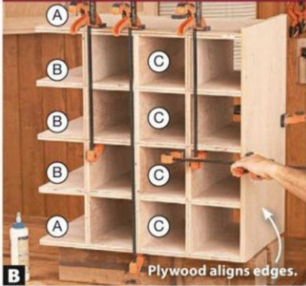
B Temporarily clamp a piece of plywood to the cabinet to align the shelves (B) and top and bottom (A) and to keep the assembly square.
