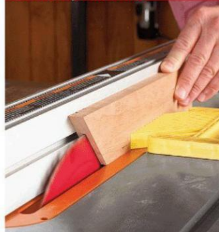
E Precisely center the slots on the mitered joint sides to ensure that both faces will be flush when you assemble the joint.
