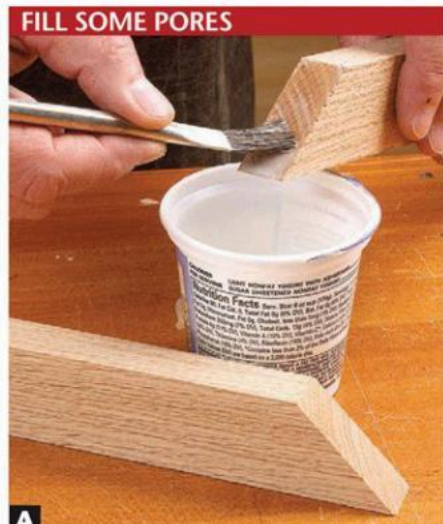
A Woodworking glue diluted with water seals the open pores in end grain. This increases gluing area and strengthens the joint.
