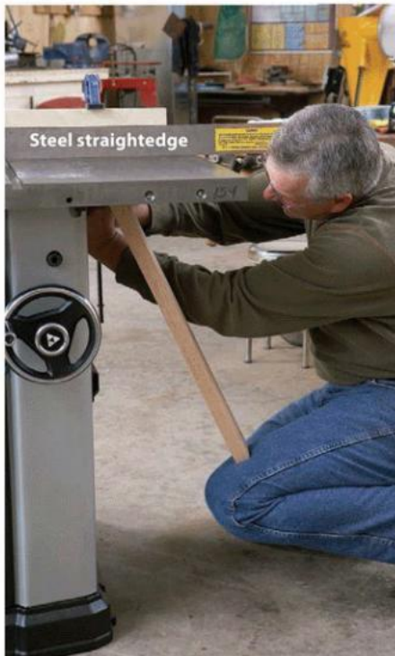
4. Insert the mounting bolts and hand-tighten them. If you need to raise the wing slightly, use a scrap board on your leg for leverage.
