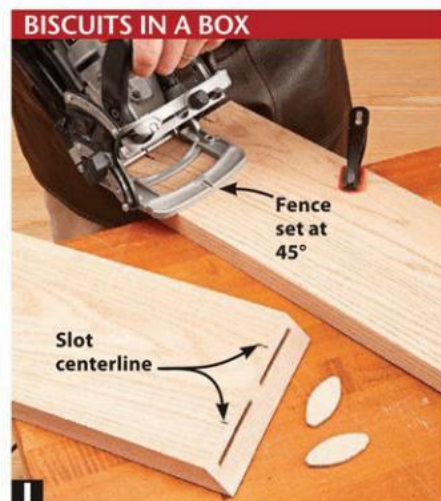
J The cutter plunges the slots straight into the face of the miter cut, allowing easy assembly and gluing of the biscuit joints.
