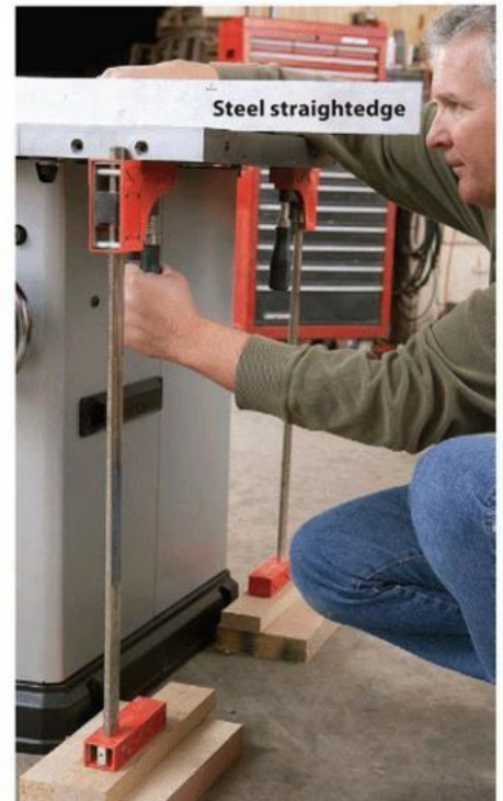
6. To remove sagging, changing a clamp to spreader mode lets you microadjust the wing height. Parallel-jaw clamps work great for this.
