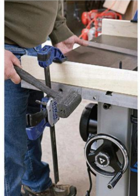
3. Now perfect the edge alignment by tapping the wing laterally with a rubber mallet until the mounting holes align.
