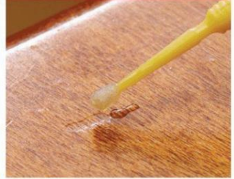
LEVEL OFF THE DIP WITH FINISH
