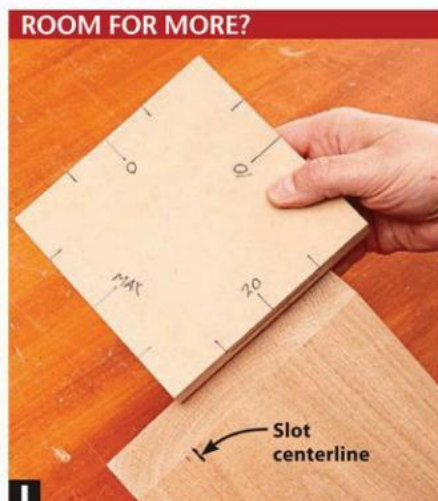
I A wider joint may have room for more than one biscuit. Space the slots evenly across the face of the joint.
