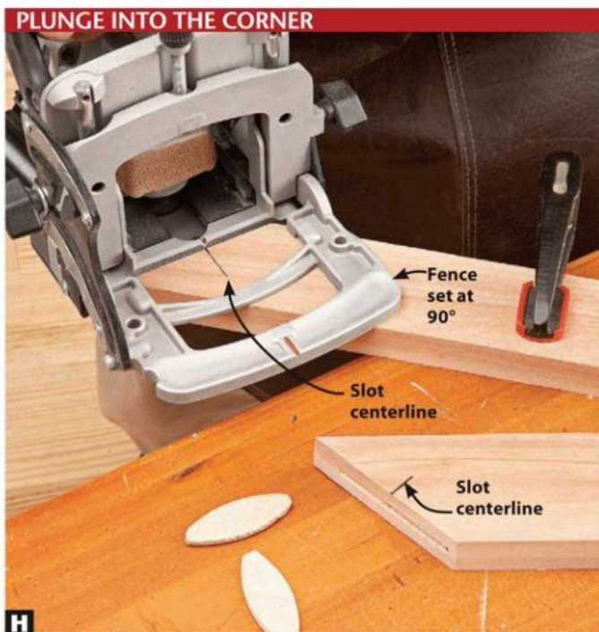
H Align the biscuit joiner on the biscuit location marked on the part. Cut the slots for both sides of the joint from the same face.
