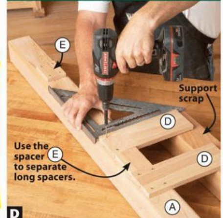
D Drill and drive one screw to secure a long spacer (D). Then hold it against a square while you drill and drive the other screws.
