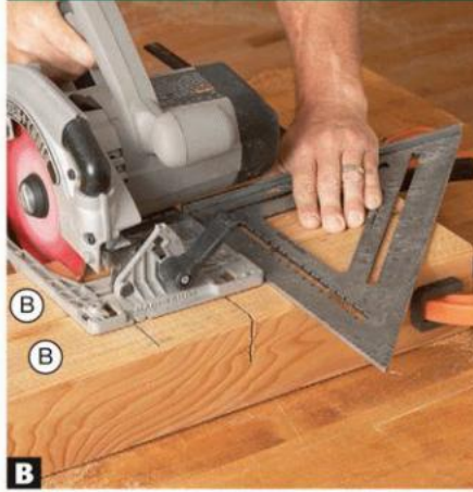
B Using a square to guide your circular saw, cut the second kerf where marked in Photo A to establish the width of your dados.
