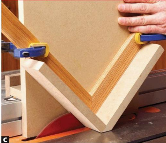
C Clamp the frame to the jig for accuracy and safety when you cut a spline slot. For splines, rip thin strips of stock to snugly fit the slots.
