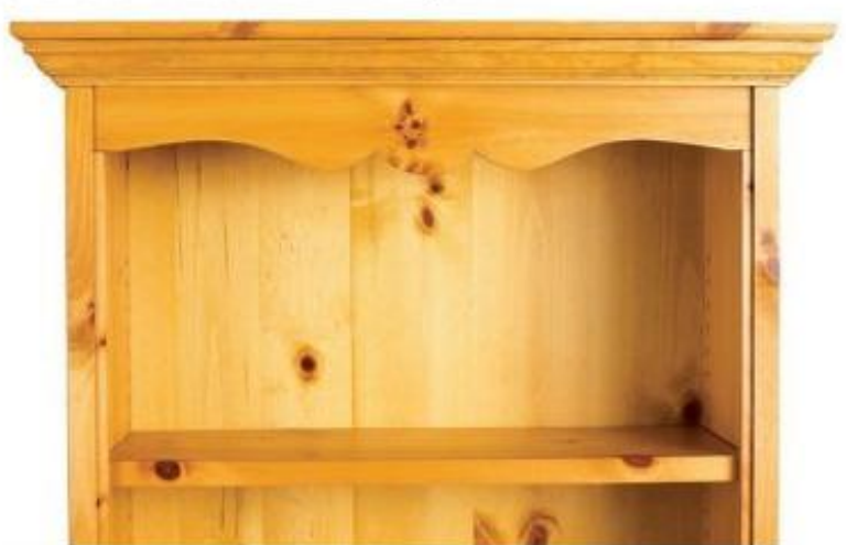
This tight cluster of knots on the top rail of a pine bookcase receives a front-and-center treatment. We used a paper cutout of the part overlaid on the uncut board to easily visualize the knots' location in the final part. 🌲
