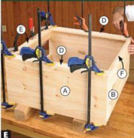
E Use the bottom rail (F) as a spacer when gluing the stiles (D) and upper rail (E) to the case. Then glue the bottom rail in place.
