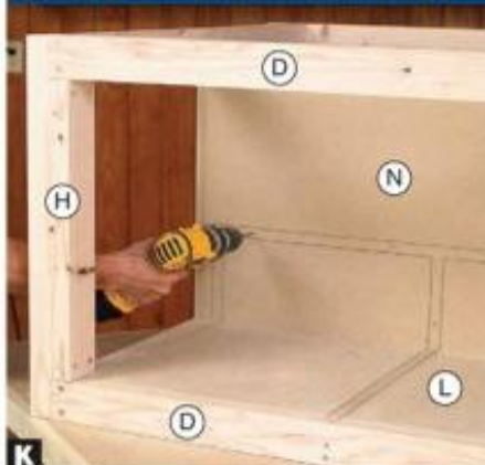
Use lines traced around the drawer carcass (O/P) to center pilot holes for attaching the carcass to the bottom (L) and back (N).
