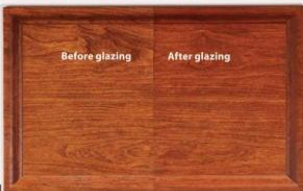
E Gel-stain glaze darkens the right side of this cherry panel without increasing the contrast caused by blotches.
