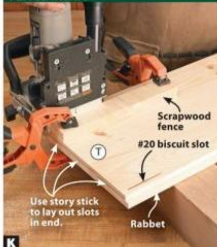
K Using the measurements in Drawing 3a, align a scrapwood fence to cut biscuit slots parallel to the front edge and the rabbet.
