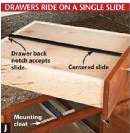
J Centered slide parts automatically center the drawer within the opening. The mounting cleat helps the slide fit this cabinet depth.
