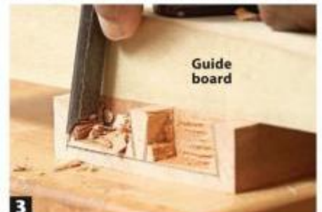
3 Pare the angled sidewalls down to the bottom of the sockets.
