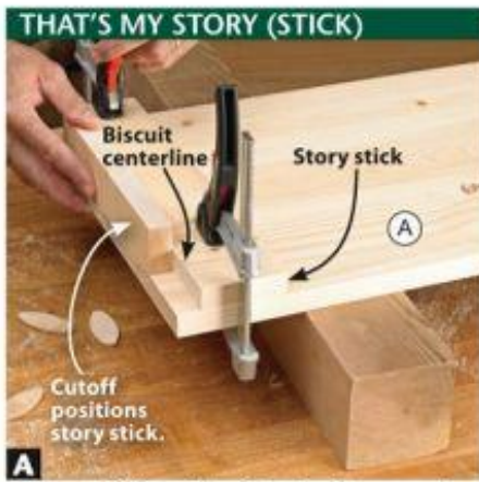
A Use a cutoff from the side or bottom panels as a story stick. Another cutoff from a panel positions the story stick.
