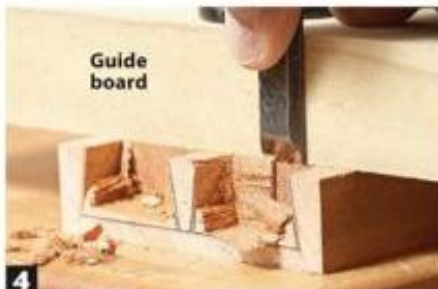
1 Remove the socket waste with a bench chisel, keeping \frac{1}{16} " from the scribed sides and back.
