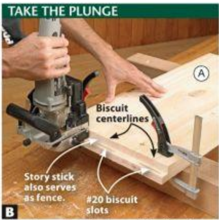
B Align the mark on the base of the biscuit joiner with the marks on the story stick and cut the biscuit slots.
