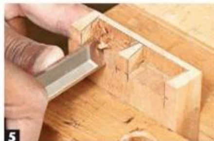
2 After making a vertical cut, counter with a horizontal cut to remove the chip.
