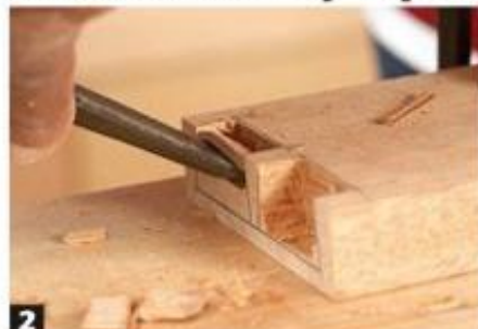
2 After making a vertical cut, counter with a horizontal cut to remove the chip.
