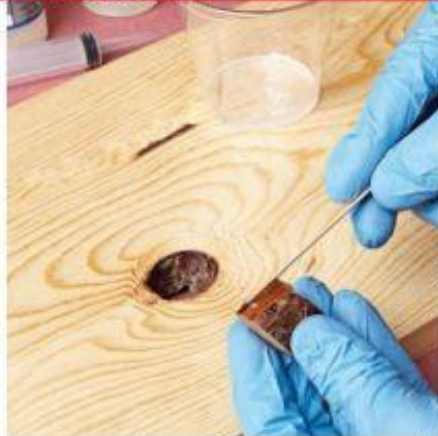
Mix up a small amount of epoxy and spread it liberally on the outside of the knot and reposition it in the board.
