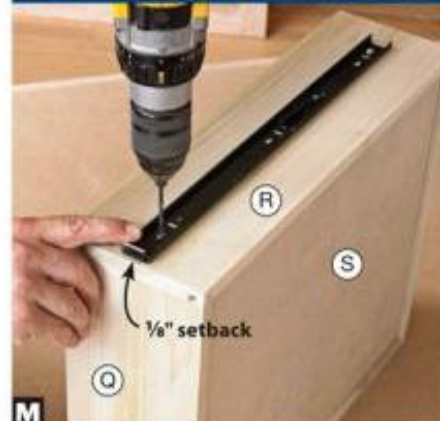
Drill pilot holes in the center of slide slots so the slides can move the drawers forward or backward within the drawer carcass (O/P).
