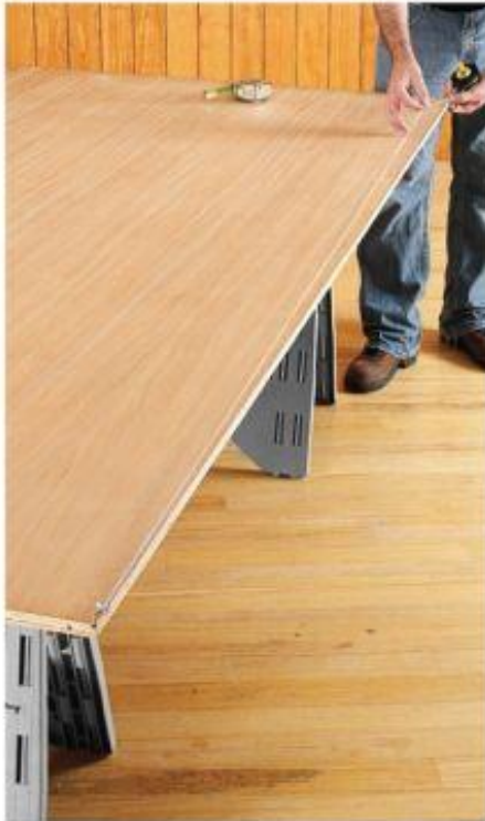
A string or a chalkline makes a ready reference for checking the straightness of a sheet of plywood.
