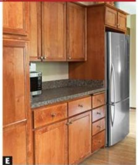
E Deep cabinets break up the line of wall cabinets, add storage, and ease access to items above the fridge.
