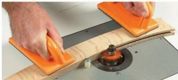
Feed the workpiece against the rotation of the bit.
