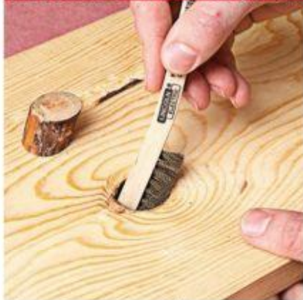
After removing the knot, clean any loose bark and debris from the knothole and the knot using a brass wire brush.
