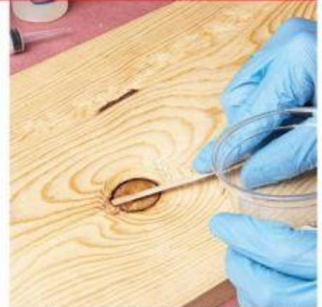
Spread additional epoxy to fill any remaining voids. After the epoxy cures fully, machine as you would any other board.
