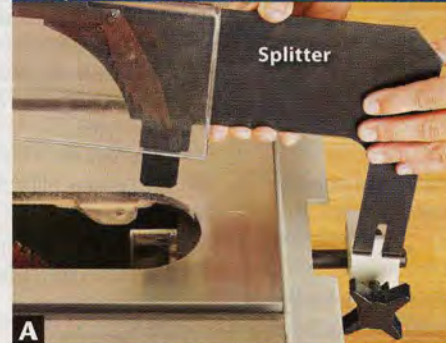
A Guards on Steel City and Craftsman saws slide into a tension clip inside the throat and over a bolt on the back. No tools required.
