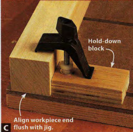
C Align workpiece end flush with jig. The hold-down block helps position the workpiece on the jig while the clamp holds it for cutting. Use the end of the jig to align workpieces consistently.
