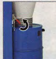
Step 1 Lift Drum Lever
