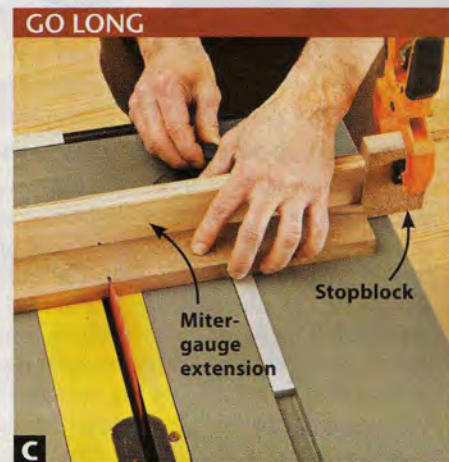
GO LONG A miter-gauge extension steadies long pieces. Clamp a stopblock to the extension to cut several pieces to identical length.
