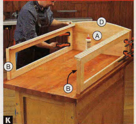
K Clamp the side assemblies to the bottom panel assembly (A/B/D) on a flat surface to avoid twisting the case.
