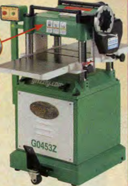
Spiral Cutterhead w/Solid Carbide Inserts Helps Reduce Tear-Out
