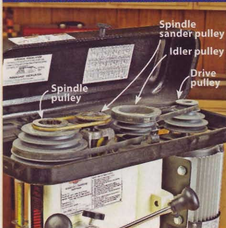
Three-pulley systems (left) provide more speed selection and slipped less under torque than stepped two-pulley systems (center) in our tests. For continuous variable speed, Ryobi's shiv pulleys (right) open and close as you change the speed setting. At top speed, as shown, the drive pulley closes down to run the belt near its outer perimeter, while the spindle pulley opens its widest. For the slowest speed, the drive pulley opens up and the spindle pulley closes down. The variable-speed presses in our test also exhibited little, if any, slippage under torque.
