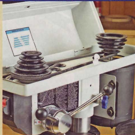
Three-pulley systems (left) provide more speed selection and slipped less under torque than stepped two-pulley systems (center) in our tests. For continuous variable speed, Ryobi's shiv pulleys (right) open and close as you change the speed setting. At top speed, as shown, the drive pulley closes down to run the belt near its outer perimeter, while the spindle pulley opens its widest. For the slowest speed, the drive pulley opens up and the spindle pulley closes down. The variable-speed presses in our test also exhibited little, if any, slippage under torque.
