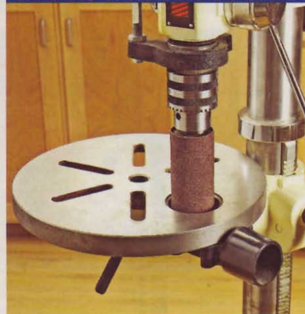
When using Shop Fox's drill press as an oscillating spindle sander, attach your shop vacuum hose to the 2¼" dust port.
