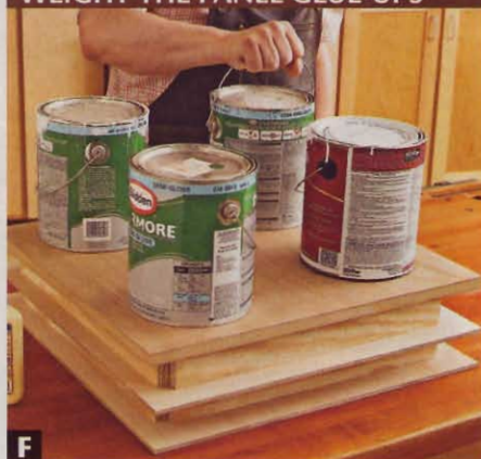
WEIGHT THE PANEL GLUE-UPS
