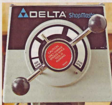
Change speeds on the Ryobi (top) by swinging the lever; the digital readout shows the speed. Adjust Delta's DP350 (bottom) by turning the dial. With no markings, though, you have to guess the speed.
