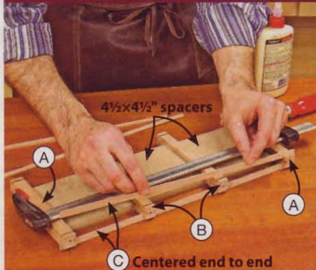
B Place spacers between the posts (A, B), align the post ends, and clamp them together. Glue the bars (C) in place, centered.
