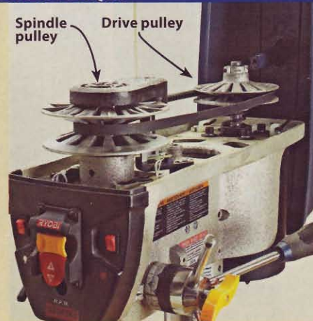
Three-pulley systems (left) provide more speed selection and slipped less under torque than stepped two-pulley systems (center) in our tests. For continuous variable speed, Ryobi's shiv pulleys (right) open and close as you change the speed setting. At top speed, as shown, the drive pulley closes down to run the belt near its outer perimeter, while the spindle pulley opens its widest. For the slowest speed, the drive pulley opens up and the spindle pulley closes down. The variable-speed presses in our test also exhibited little, if any, slippage under torque.
