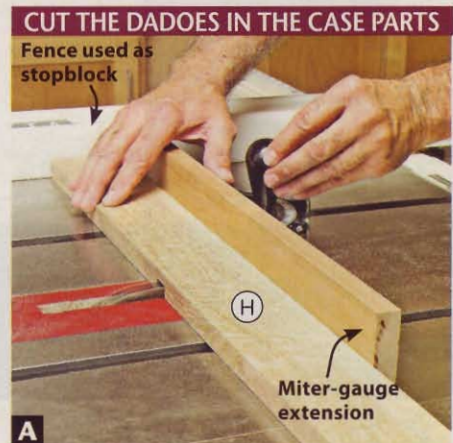
A Use your tablesaw fence as a stopblock to ensure identical dado locations in the sides (A), dividers (B), bottom (F), and cleats (H).
