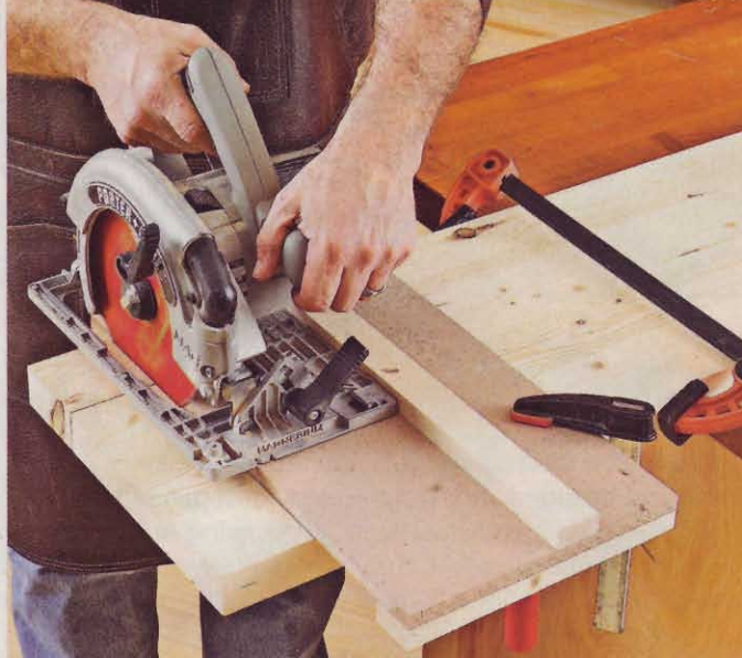
Align the saw edge of the jig with the rabbet layout line, clamp the jig in place, and cut a saw kerf to define the rabbet shoulders.
