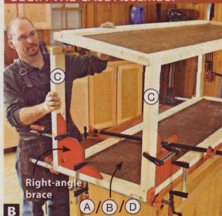
B With the stretchers (C) attached to the first side (A/B/D), apply glue to the stretcher rabbets, and position the second side.
