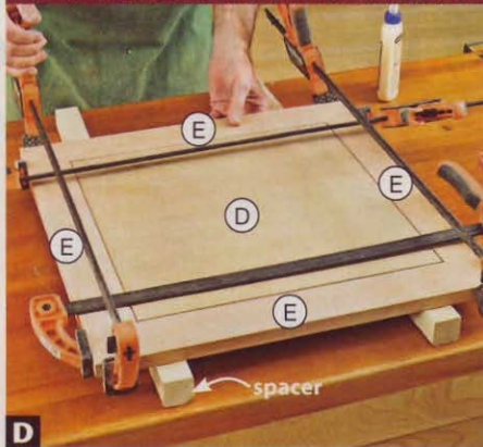
D Using spacers for clamp clearance, glue, biscuit, and clamp the tall-table top trim (E) to the top panel (D) with the top faces flush.
