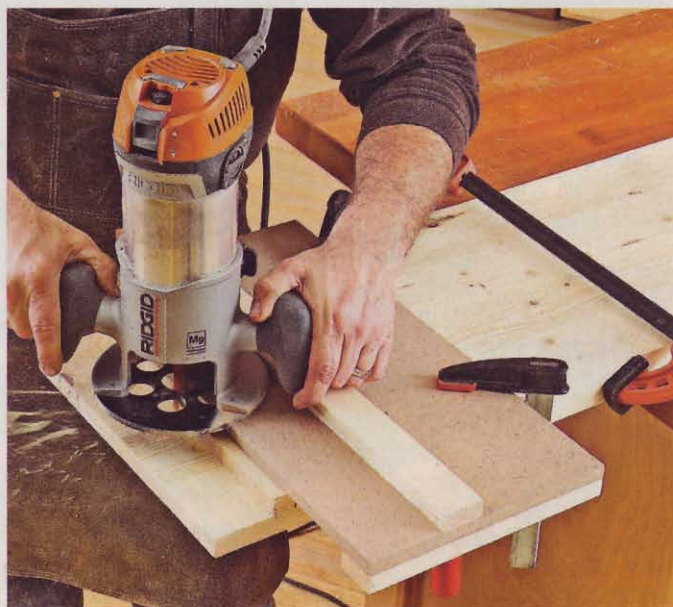
To clean out the rabbets, start with the router edge of the jig \frac{3}{8} " from the stile ends, and make repeat router cuts to the saw kerf.
