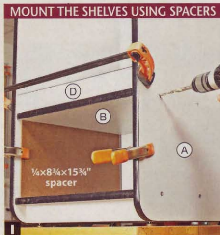
I Position and clamp a large shelf (B/D) in bin 4 on 8 \frac{3}{4} "-wide hardboard spacers. Drill the mounting holes, and drive the screws.
