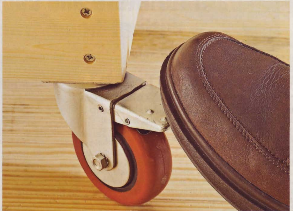
Casters that lock both the wheel and the swivel action prevent tools and cabinets from moving until you want them to.
