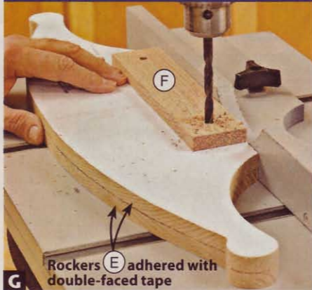
G Rockers (E) adhered with double-faced tape. Using your drill-press fence for support and the holes in the rocker bracket (F) as guides, drill \frac{5}{16} " holes through the rockers (E).
