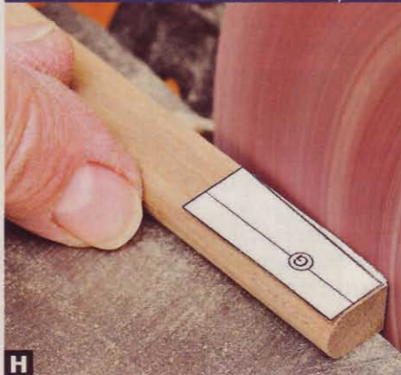
H Taper the end of the blank for the wedges (G) to the angled wedge pattern line using a 120-grit disc sander.
