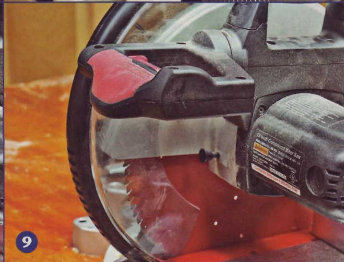
6 The dust-collection chute blocks Hitachi's laser as you lower the saw for a cut, so you might have to line up your cut at full height.
