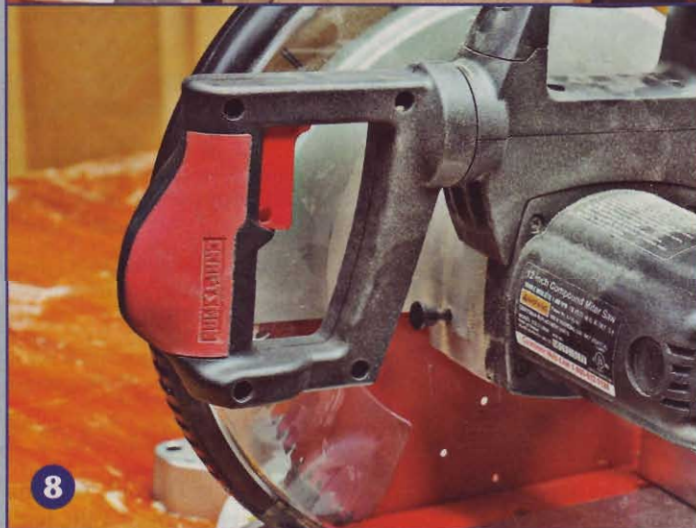
6 The dust-collection chute blocks Hitachi's laser as you lower the saw for a cut, so you might have to line up your cut at full height.
