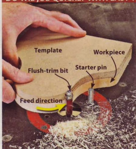
Using a flush-trim bit on a router table allows you to better see the larger workpiece because the smaller template rides on top.
