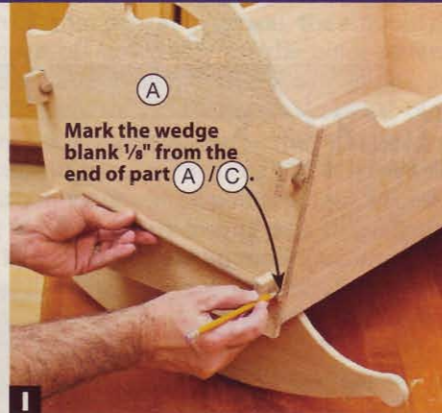
I With the tapered end of the wedge blank tight in an angled mortise, mark the blank \frac{1}{8} " from the end of the end (A/C).
