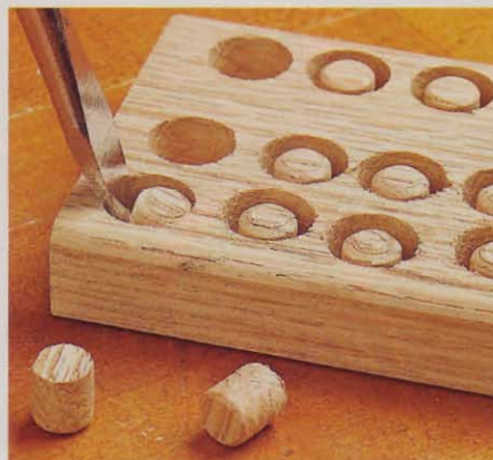
To free plugs cut into scrap, insert a screwdriver into a plug hole at the end grain and pry gently. Cut extras to improve your chances of matching workpiece surfaces.
