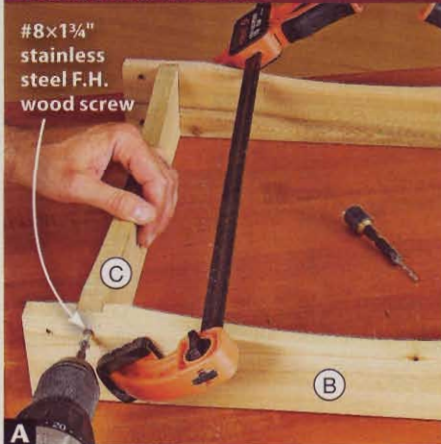
A Glue and clamp the side rails (C) into the end rail (B) dadoes. Check for square, drill pilot holes, and drive the screws.
