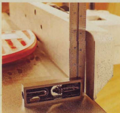
A misaligned jointer fence means out-of-square stock. Check the fence regularly to ensure it's square to the bed.
