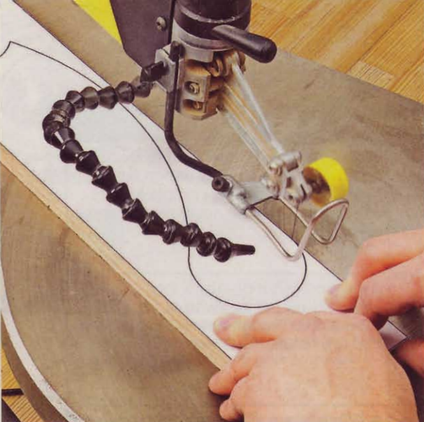
Make your own super-sized part patterns using CAD drawings saved as PDF files that can be printed at a local copy shop.
