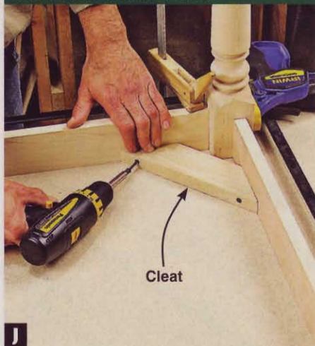
J These cleats not only hold the assembly square but also provide contact points from which to secure the tabletop.
