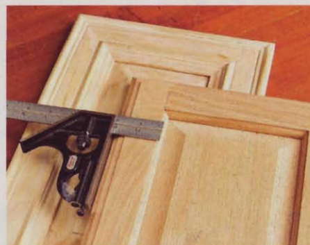
These unfinished door frames measure 2" (top) and 2 3/4" wide.
