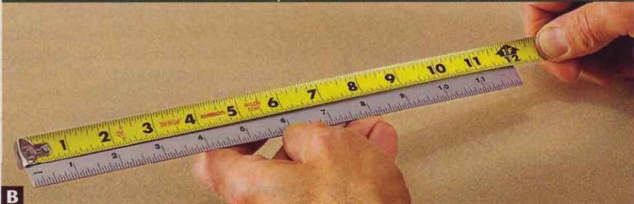
B Rely on an accurate steel rule to check your measuring tape at the 12" mark. This tape proved to be \frac{1}{32} " longer than the rule at that mark.
