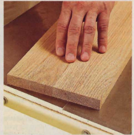
Two boards may appear to have the same thickness, but running fingertips over the surface will turn up planing inconsistencies.
