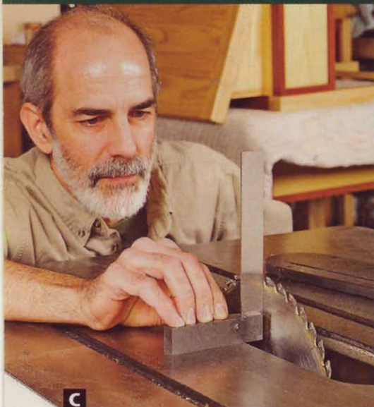
C Check the blade's squareness from the side with the narrowest throat opening. Place the square against the blade's body, not its teeth.
