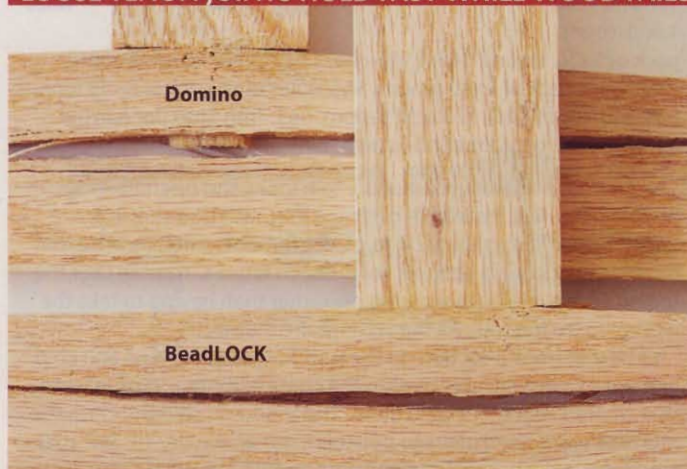
Both the BeadLOCK and Domino glue joints held fast in the pull-apart test. Note how the stiles broke apart at the bottom of the mortises.
