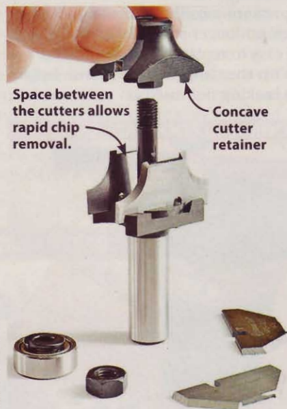
Concave or convex retainers support the edges of the interchangeable cutters in Amana's Nova bits.
