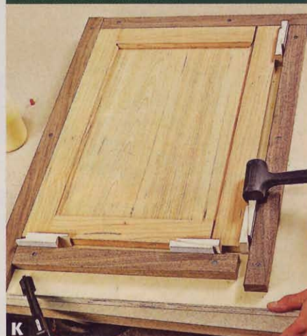
K Apply a film finish to the jig's base or place waxed paper underneath your workpiece so it doesn't become glued to the jig.
