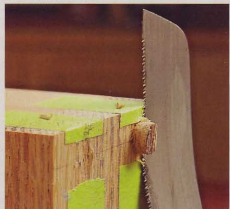
Exposed plugs can be sawn flush or shaved flush with a chisel. Masking tape reduces the likelihood of marring surrounding wood with the saw's teeth.
