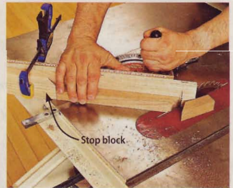
This angled stop block, clamped to a miter-gauge extension, ensures that all mitered frame parts are cut to identical lengths.
