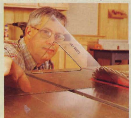
A plastic drafting triangle from an office supply store provides an accurate, inexpensive way to measure blade angles.
