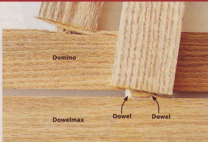
In the shear test, Domino's sample broke along the stile's grain. The Dowelmax sample failed when wood between the dowels gave way.
