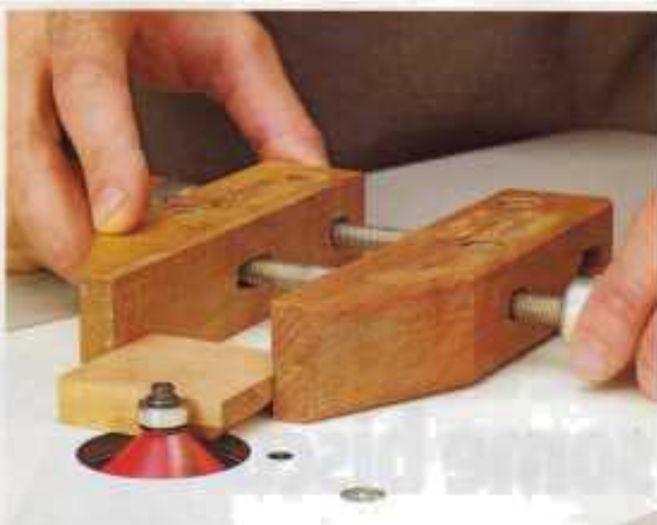
A wooden handscrew clamp serves as a safe extension of your hands, gripping the small part firmly while sitting flat on the table surface as you rout its edges.
