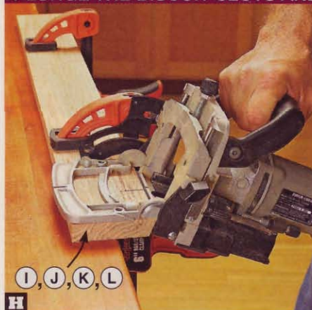
H With the stiles (I, J, K, L) clamped to your workbench, plunge #20 biscuit slots into the beveled edges at the marked centerlines.
