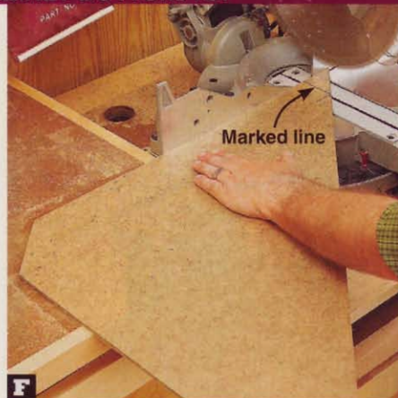
F Positioning each side of the template tight against the fence of your miter saw, cut the corners along the marked lines.
