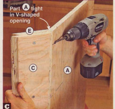
With the beveled edge of the bottom-case left side (A) tight in the V-shaped opening in the back (C/E), drive the pocket screws.
