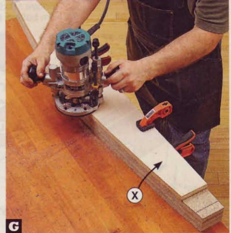
G Clamp the crest (X) to the form between the marked lines and flush at the bottom edge. Then flush-trim its rough-cut edge.
