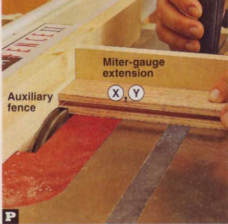
P Using an auxiliary fence attached to your rip fence, cut a 1/4" tenon 3/8" long on each end of the bottom and top rails (X, Y).
