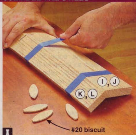
I Glue and biscuit the bottom- and top-case corner stiles (I, J) and front stiles (K, L) together, drawing the joints tight with tape.
