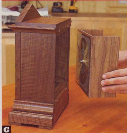
G With the clock face correctly oriented, slide the clock-face sides/backer assembly (C/D) into the case, tight against the stops (E).
