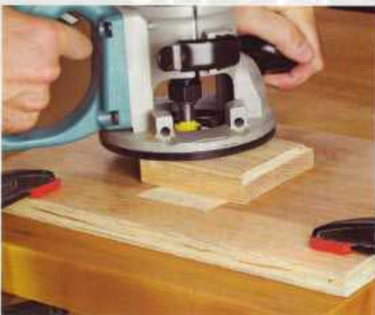
For handheld routing of small parts, clamp a scrap to your workbench and apply cloth-backed double-faced tape to the top. Press the small part onto the tape for a secure hold during machining.
