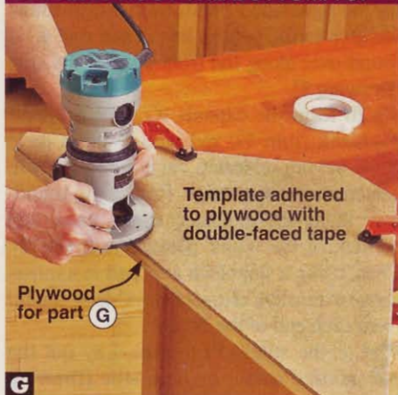
G Keeping the bearing of the flush-trim bit tight against the hardboard template, pattern-route the plywood bottom/top (G) to shape.
