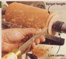
turned our spigot to a 21/4" diameter.) Now use a skew chisel to undercut the spigot, matching the angle of the chuck jaws.
