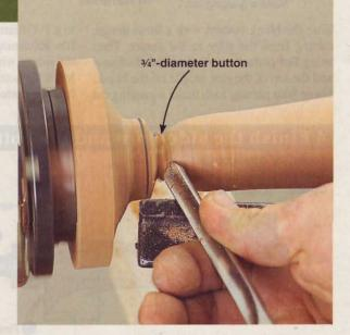
Using a parting tool, make a gauging cut to a 11/4" diameter at the top of the side profile. Checking your progress with **Template 1**, use a bowl gouge to finish-turn the profile. Then using **Template 3** as a guide, mark the
