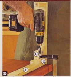
Then glue and clamp each base side/support assembly (G/E) to the base front (F). Drill pilot holes, and drive the screws.
