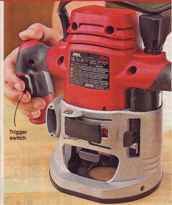
The power switch should be within easy reach without letting go of the router. Porter-Cable's 890-series fixed-base router has a dual-position switch that works well both when handheld and inverted in a router table. Skil's trigger switch keeps power control literally at your fingertips for handheld use, but is more difficult to activate and lock when table-mounted.
