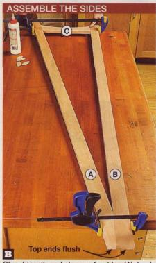
Glue, biscuit, and clamp a front leg (A), back leg (B), and side rail (C) together to form each side, keeping the leg top ends flush.
