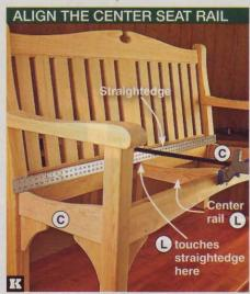
Align the center rail (L) with a straightedge resting on the top edges of the end rails (C). Then clamp the center rail in place.
