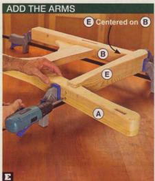
Glue and clamp the arms in place. Then using the holes in the rear legs as guides, drill pilot holes into the arms, and drive the screws.
