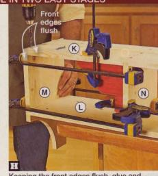
Keeping the front edges flush, glue and clamp the sides (M) to the case (K/L/N). Drill mounting holes, and drive the screws.
