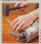
Give the wrench a light whack. Make sure you're turning the nut in the right direction. Be careful not to damage the bit or the plunge rods in the process.
