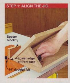
for box corner splines that pass the length of the miter, as shown on *page 37*.
