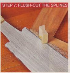
Then apply glue to the sides of the butterfly splines and insert them through the openings. Once the glue dries, flush-cut the splines to the frame surface, as shown in Step 7, and sand flush.
