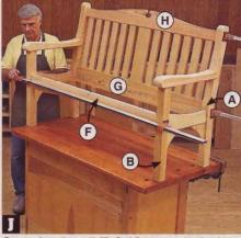
Capturing the rail (F, G, H) tenons in the leg (A, B) mortises, glue and clamp the end assemblies to the front rail and back assembly.
