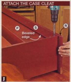
With the case cleat (S) tight against the shelf (R) in the orientation shown, drill pilot holes into the case and drive the screws.
