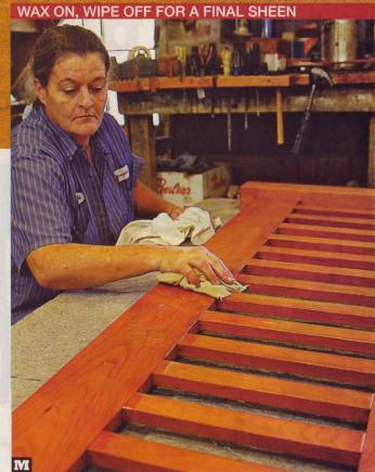
After three coats of an oil-varnish blend and a light burnishing with 0000 steel wool, the finished piece is given a light coat of wax. The light wax topcoat makes the wood shine like stone.
