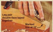
works well.) Check with a square that the edges are 90° to the faces. This will ensure a tight and flush joint between the front and back legs at the top.
