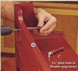
pegs in the holes. To strengthen the peg attachments, drill pilot holes and drive screws into the pegs, as explained in the **Shop Tip**, *above*.
