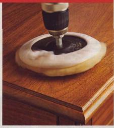
When the wax coat turns dull, buff it with a pad installed in a portable drill. Woodworker's Supply (800/645-9292) carries a wool pad (item 958-735) for \$10.99 and a backing disc (958-728) for \$21.49.
