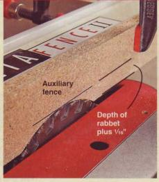
auxiliary fence covers all but about 1/16" of the blade, and lock the fence in place. Now turn on the saw and slowly raise it to the marked line, as shown above. (The extrawidth cut in the auxiliary fence provides for plenty of side-to-side adjustment.) Turn off
