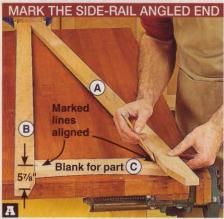
With the front leg (A) resting on the side-rail blank (C), draw a line along the leg back edge to mark the angle on the rail blank.
