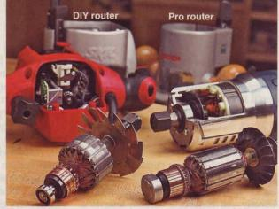
The quality of the internal workings separates pro-level routers from DIY models. Larger bearings and beefier motor components help the pro model run cooler and last longer.
