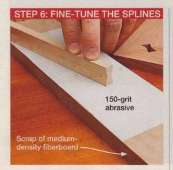
If the spline is too long, sand equal amounts from both sides using adhesivebacked 150-grit sandpaper on a flat surface, as shown in Step 6. Custom fit keys to each corner and cut them about 1" thicker than needed. Mark which spline goes in each corner and its orientation.
