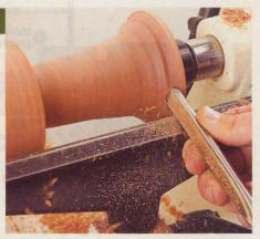
back the tail center away and finish the bottom profile. To reduce the chance of a tool catch when starting a gouge cut at the rim of a project, see the **Turning Tip** on page 82.
