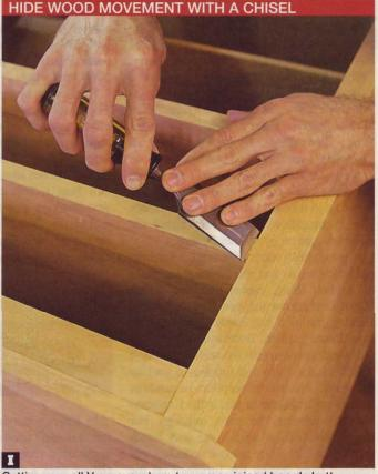
Cutting a small V-groove where two cross-joined boards butt together helps conceal future wood movement and adds a handtooled touch. Here, a sharp chisel and light touch do the trick.
