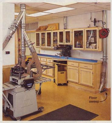
Each of the stationary tools feeds dust into the collection system, including the radial-arm saw with a wall-mounted chute. The system's floor sweep is shown to the right.
