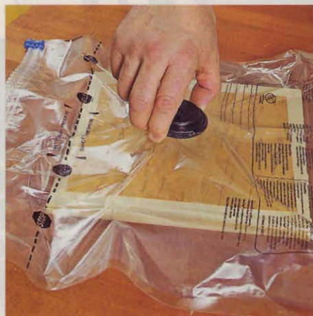
Lifting on the Space Bag's one-way valve shows how much hold-down pressure the bag lost overnight.
