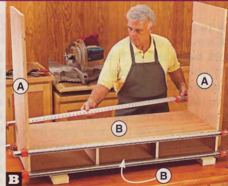
B Spread glue in the side (A) rabbets and dados, and clamp the sides to the top and center panel (B) with the front edges flush.
