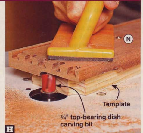
H Follow the template with a top-bearing dish carving bit raised 1" above the table. Make extra passes to remove waste at the corners.
