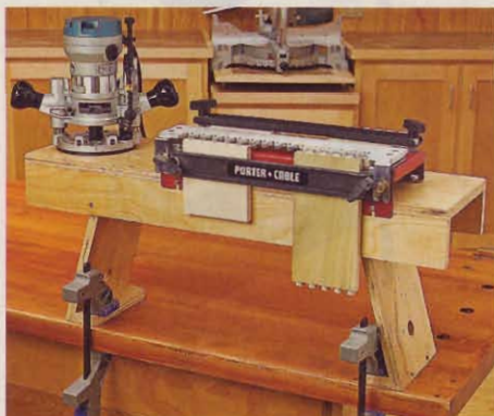
This 12\frac{1}{4} "-high stand makes routing easier by letting you work without bending over.
