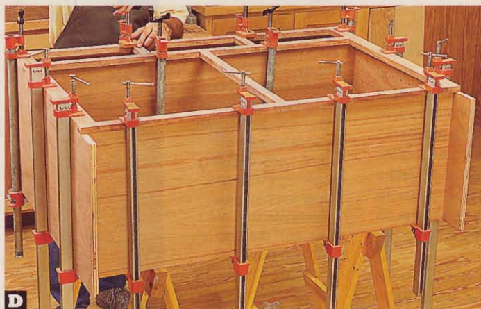
D Spread glue on the front edges of the case parts and clamp the assembled face frame in place, keeping the outside edges flush.
