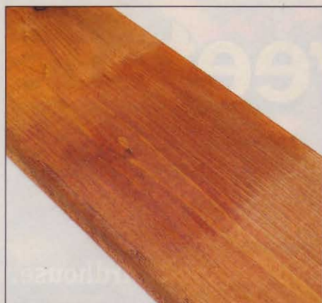
Shades of difference can appear when sun-heated surfaces cause semitransparent stains to dry too quickly.
