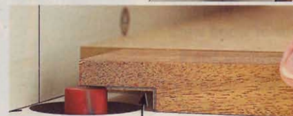
After rabbet-cutting with a dado blade, rout away the final \frac{1}{16} ".
