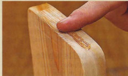
Press an effective clear adhesive sealant into end grain. Here we use an elastomeric.
