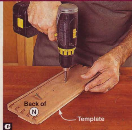
G Secure the front (N) to the template by driving 1 1/4"-long wood screws through the previously drilled pull holes.
