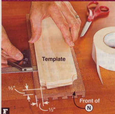
F Adhere the template to the front face of the drawer front (N) with double-faced tape, centering the template on the front.
