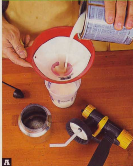
A Spray-gun nozzles clog quickly unless you strain out bits of debris and dried finish. Use a fine-mesh cotton filter for thin-body materials, such as lacquers, and a medium filter for most thick-body paints.
