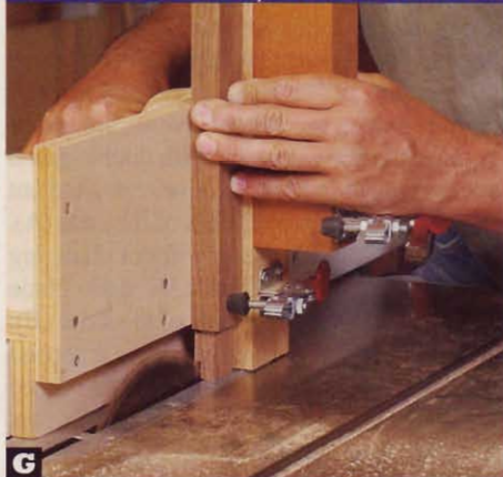
G Only if the jig fits snugly over the tablesaw fence and rides smoothly along it will it cut clean, well-proportioned tenon cheeks.
