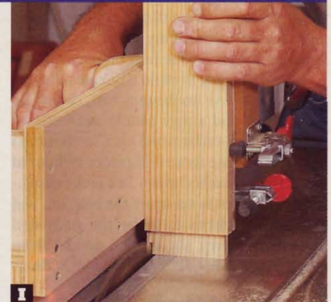
I On wider stock, Zane nixes the spacer and relies on the outer clamp to secure the workpiece when cutting cheeks.
