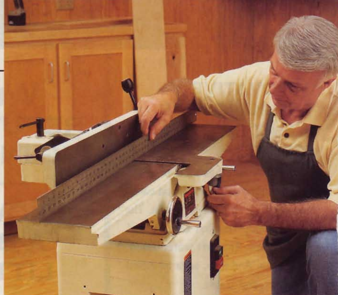
Check for parallel alignment by raising the tables to full height and laying a straightedge across them. Light showing beneath indicates a need for adjustment.
