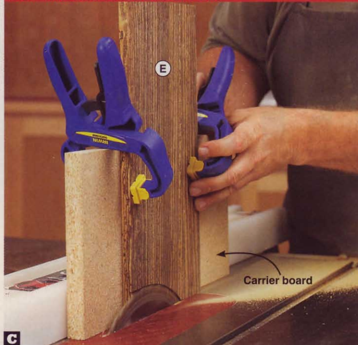
C To steady the lid (E) and keep your fingers away from the blade when cutting the end rabbets, clamp the part to a carrier board.
