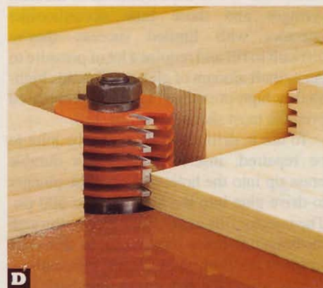
D For end-grain cuts, mount an auxiliary face on your miter gauge. Note that the abetting head cutter is now set for cutting thin stock.
