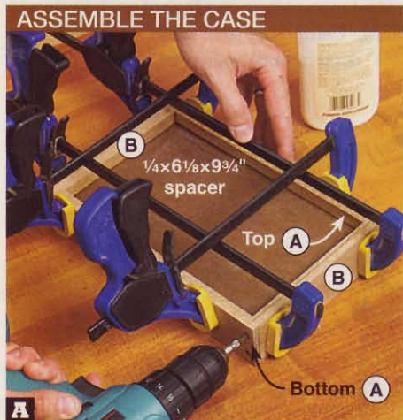
With the case top/bottom (A), sides (B), and 1/4" spacer clamped together, drill pilot holes and drive the screws through the bottom (A).
