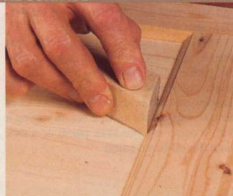
Foam sanding pads and sandpaper-wrapped blocks reach into corners.
