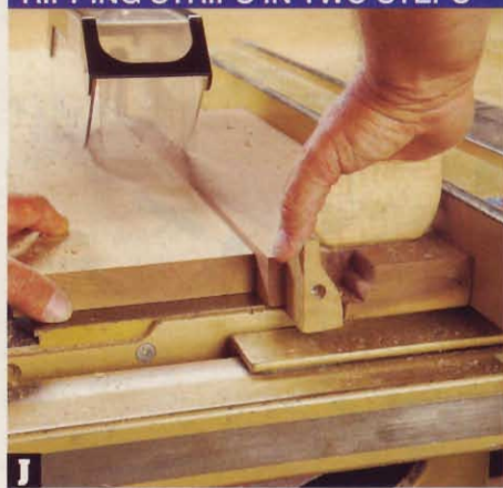
J First use the base of the thin-strip ripper as a fence by sliding the workpiece along its edge after setting up the desired strip width.
