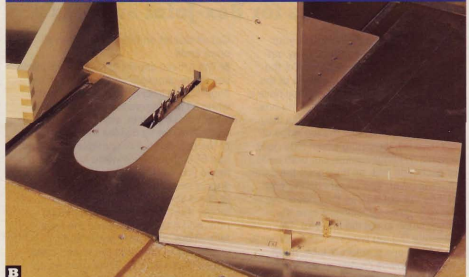
B Zane makes several easy-to-add front faces for different size box-joint fingers. These attach with machine screws, washers, and knobs.
