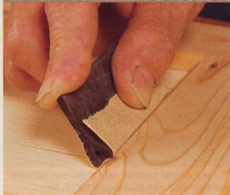
Sanding profile blocks conform to routed contours and reach into tight spaces.
