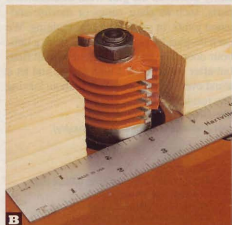
B The ball-bearing guide of an adjustable bit must be flush with the router fence.
