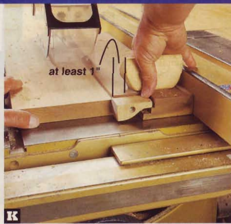
K As the cut proceeds, drop down the toggle to serve as a ledge for supporting the workpiece and safely completing the cut.
