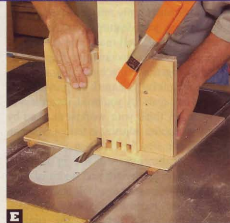
E Use the notched first workpiece, as shown, to establish the location of the beginning (open) notch to be cut in the mating workpiece.
