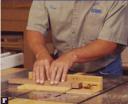
F Raise the blade to the establish the needed tenon depth. Then, using the jig, cut shoulders on the workpiece faces and edges.
