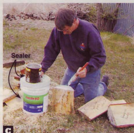
C Apply sealer to the blank ends with an inexpensive 3" brush. When processing large quantities of stock at the same time, speed the task by using a paint roller.
