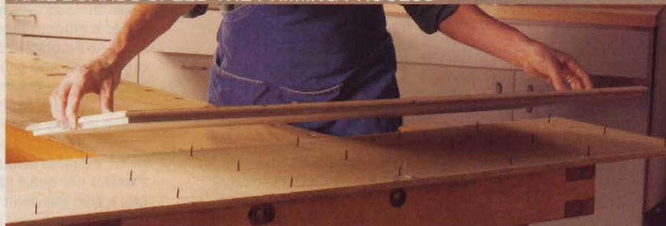
A nail board supports the freshly primed door of the chimney cupboard, allowing both sides and all four edges to be finished at once. With their fine points, drywall nails provide even support with only imperceptible marring.
