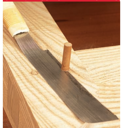
STEP 9: FLUSH-SAW THE DOWELS
