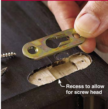
An extra recess beyond the one for the fastener allows a screw to slide into position on the narrow part of the keyhole.
