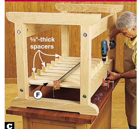
C Separate the slats (F) with \frac{5}{8} "-thick spacers. Then using the slat holes as guides, drill pilot holes into the cleats (D) and drive the screws.
