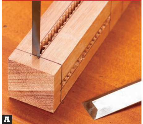
To avoid splitting, clean up the ends of the leg (A) mortises using a ¼" chisel. Then pare the sides using a chisel at least ¾" wide.
