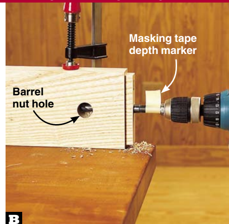
B Mark the \frac{3}{4} " hole depth on the drill bit with masking tape. Aiming for the center of the barrel nut hole, extend the hole to full depth.
