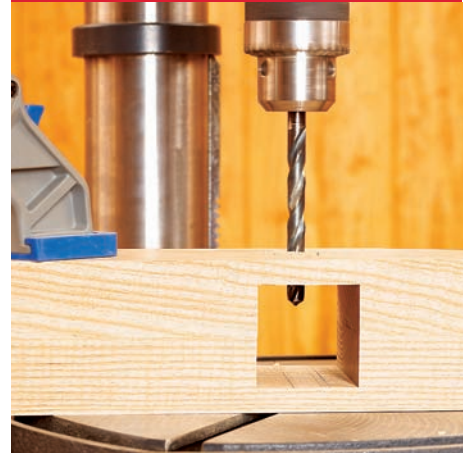
STEP 6: START THE DOWEL HOLES
