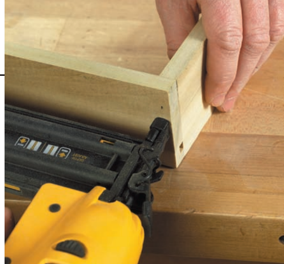
A lightweight brad nailer offers a convenient way to hold furniture joints while glue dries, as in the drawer construction shown here.
