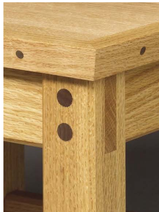
Miller dowels reinforce a mortise-and-tenon joint, and secure the edge trim on this table.
