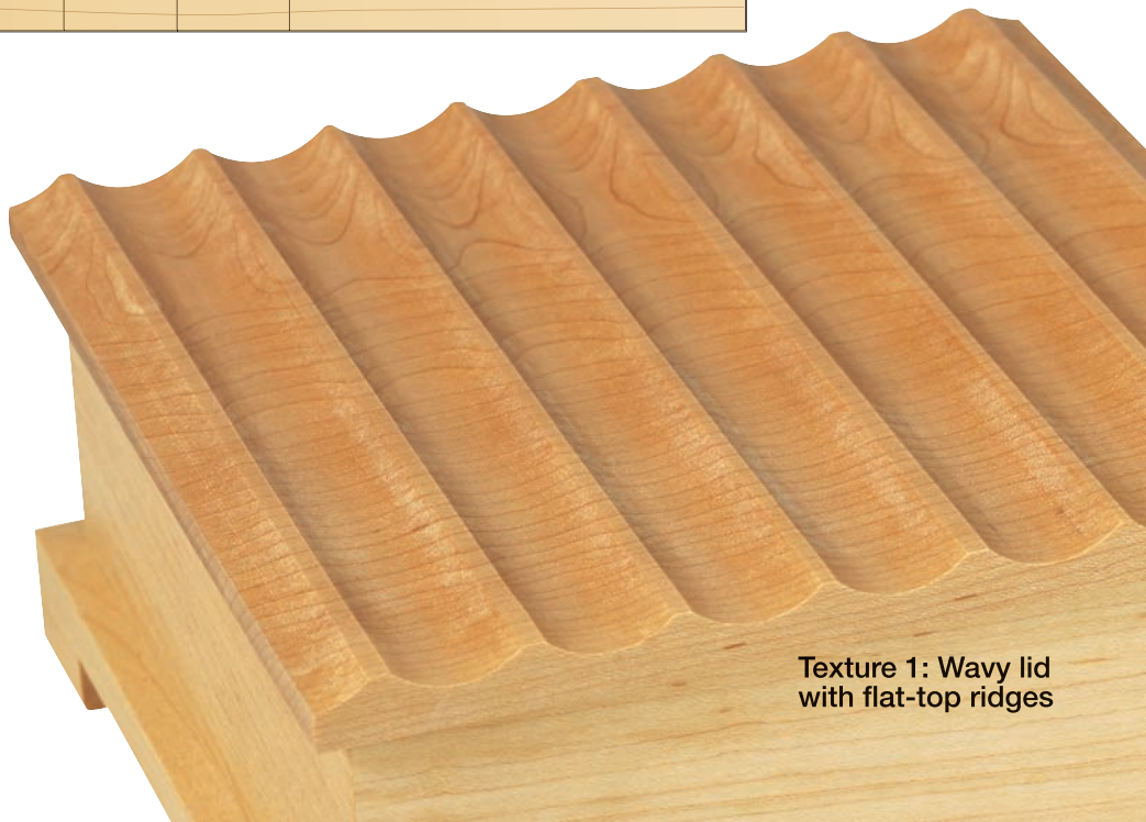
A Center the tip of the round-nose bit beneath each evenly spaced mark indicating the center of a groove. This maple workpiece includes a 1/8" layer of cherry for contrast.
