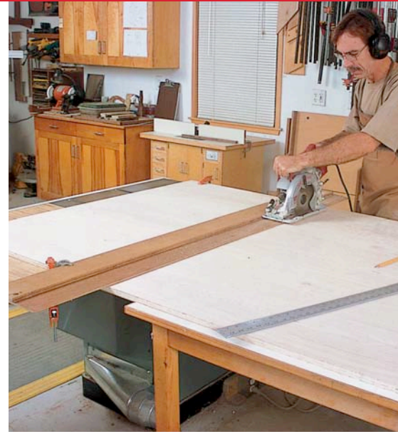
Pulling the table away from the saw transforms Paul's outfeed table into a plywood crosscutting station.
