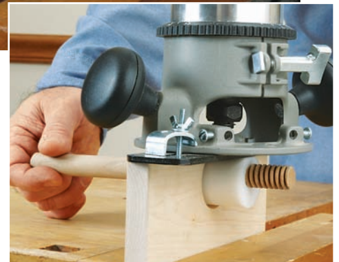
You can cut threads manually with a traditional threadbox shown above or add a Beall jig to your router for a power assist, as shown at right.
