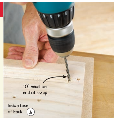
A Clamp the back (A) and side (B) together using a squaring brace to keep the parts square. Then drill the pilot holes in the side.
