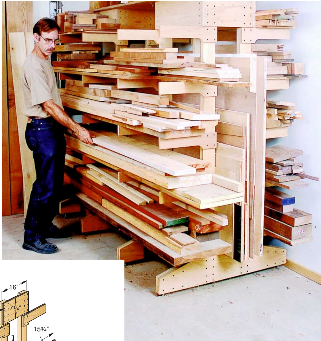
Paul's easy-to-make rack keeps boards and panels out of the way, but always at arm's reach. When not in use, disassemble and stack it out of the way.
