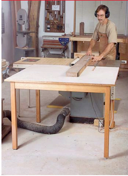
Having a big outfeed table at the far end of your saw is the best way to keep control over long boards or sheet goods during the cut.
