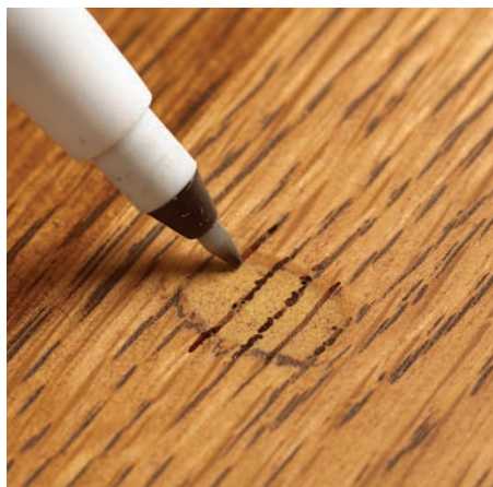
A graining pen helps you reproduce grain lines that mimic wood. A fine-bristle brush and dark pigments produce a similar look.
