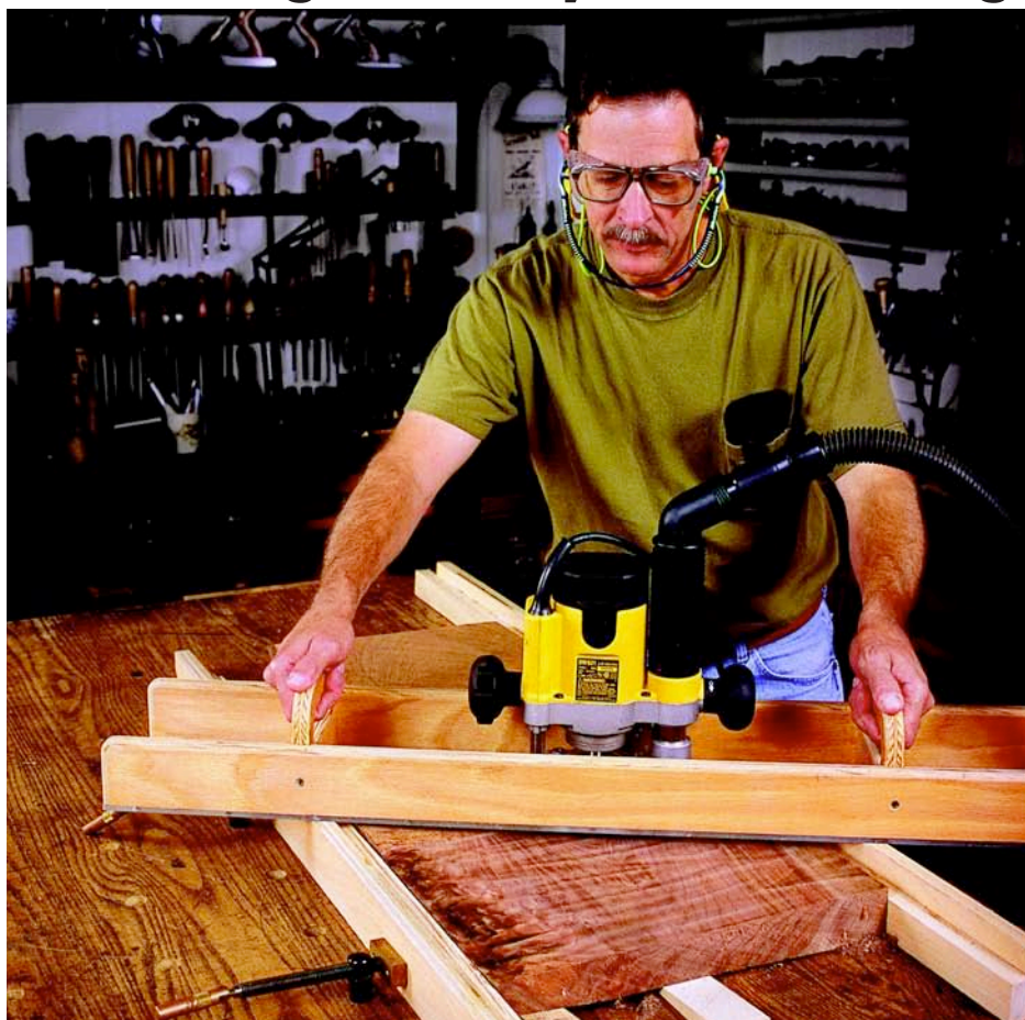
Craig Bentzley's super-simple planing jig cuts through all types of tough stock without tear-out. And while most jointers max out at 6 or 8"-wide, this jig can flatten boards up to 17".
