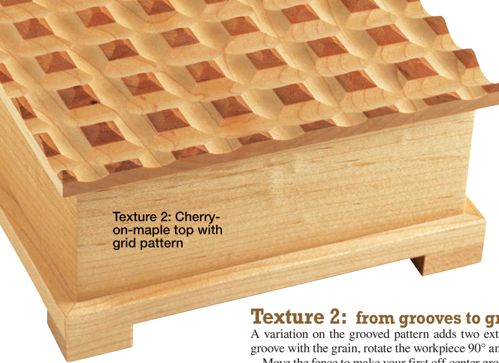
C Making the grid pattern is as simple as rotating the workpiece three times for each off-center pass.
