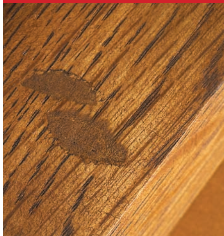
The porous texture of some wood putties makes them soak up more stain than the surrounding wood.
