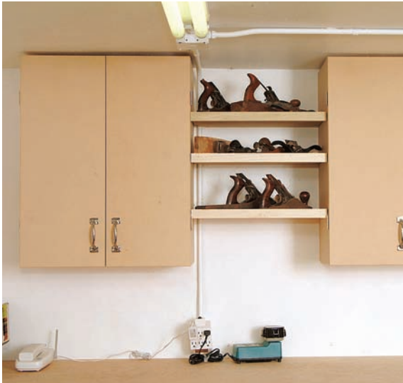
Two wall cabinets were mounted 18" above the countertop beside the mitersaw work station. The 18" space between the cabinets allows them to support adjustable shelving for added storage.
