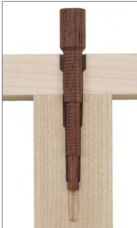
Steps formed by the drill bit are slightly longer than the ribbed steps on the dowel.
