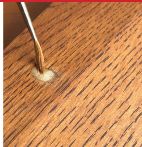
To avoid excess stain both in and around the patch, cover the putty with a light coat of shellac before attempting a color match.
