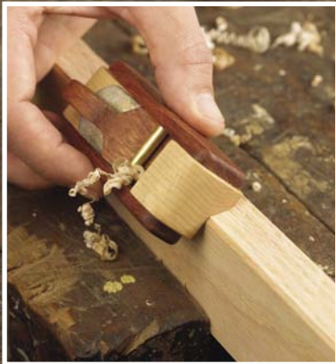
To chamfer an edge, simply ride the angled portion of the plane sole on one surface of the workpiece.
