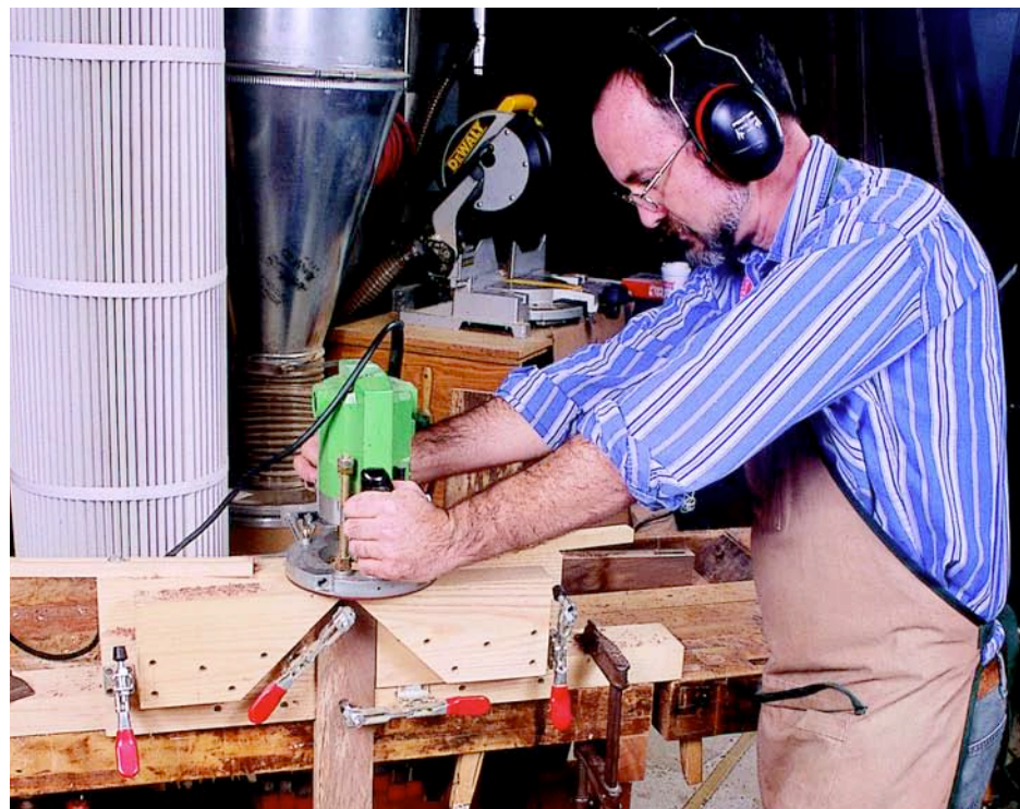
Craftsman Ken Burton saves time milling mortises using his customized scrapwood jig. The long base allows him to clamp the jig firmly to the workbench.
