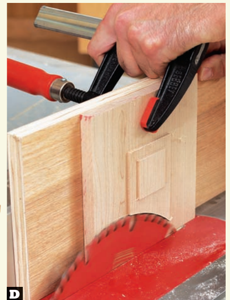
D To solve tear-out problems, cut passes against the grain before cutting the two with the grain. Use the clamp as a handle.
