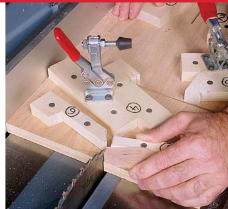
Kept at a safe distance, fingers and a scrap backer work well to secure a part for sawing.
