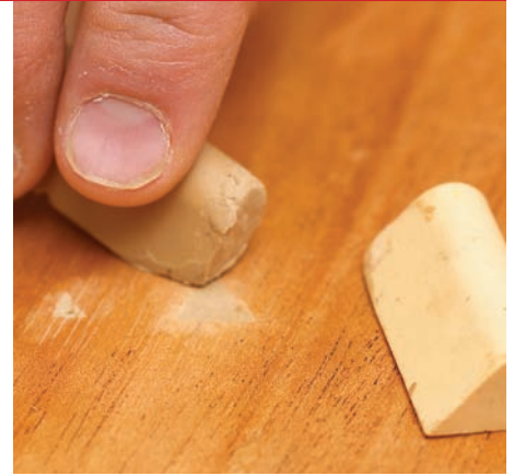
Colored putty sticks can be rubbed into minor dings for a quick fix. Some types can be blended to create custom colors.
