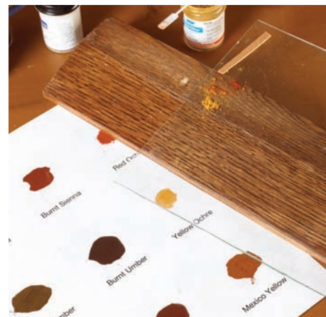
Pigment samples sealed in place with clear shipping tape make it easier to estimate the colors needed to match surrounding wood.
