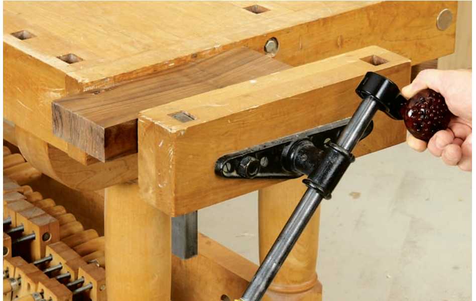
Twirling a steering wheel spinner opens and closes your bench vise quickly when it doesn't have a quick-release mechanism.
