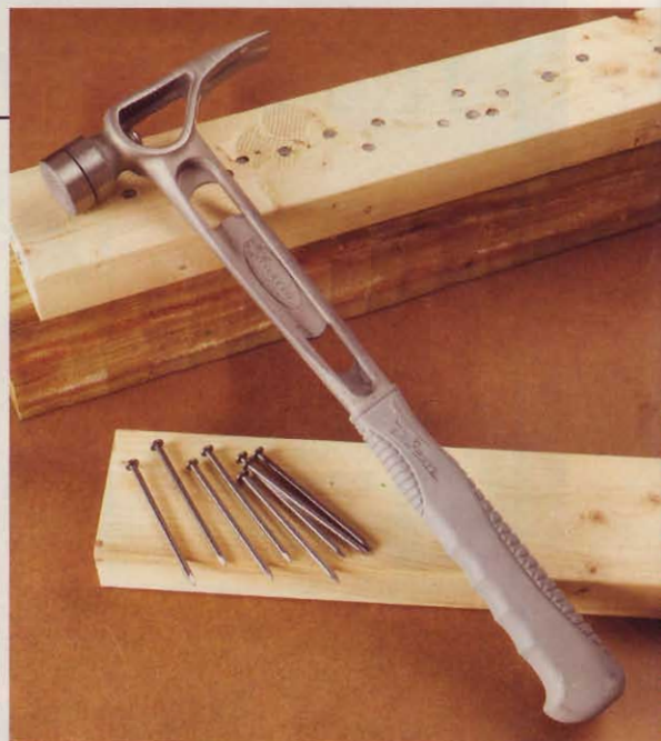
This titanium hammer, with its interchangeable smooth or milled face, cost a bundle, but may be worth it for the professional framer.
