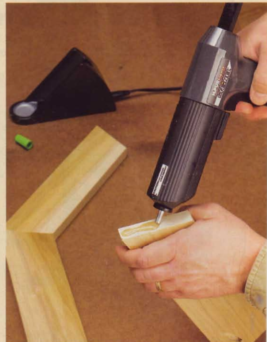
Titebond's HiPURformer system uses glue cartridges in a heated gun, and the three formulations of glues have different open times (30, 60, and 75 seconds).
