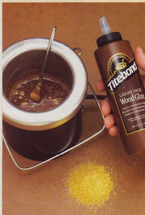
Traditional hide glue comes in dry crystals that you mix with water and heat in a pot. Titebond's premixed Liquid Hide glue proved far stronger and easier to use in our tests.
