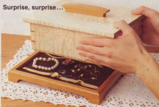
Walnut and curly maple with a maple golden amber aniline dye applied.
