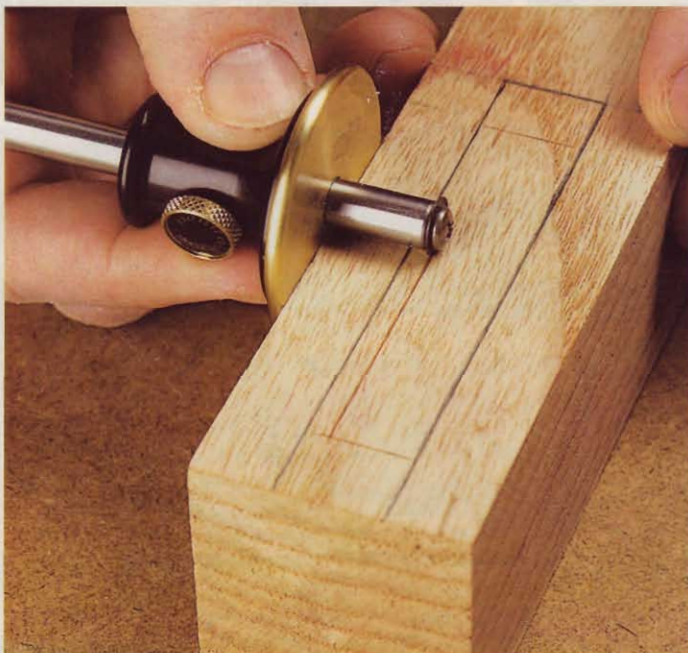
Use a marking gauge to strike a fine line parallel to the workpiece edge. Here we're marking the mortise location for a rail after drawing the rail end location.
