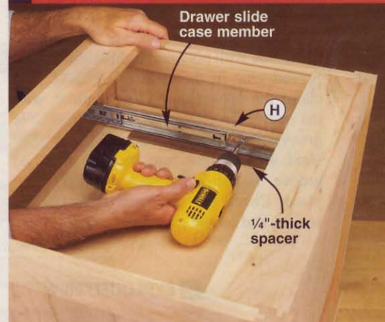
Place the slide case member on a 1/4"-thick spacer. Align the front edge of the slide with the front edge of the cleat (H). Drill holes, and drive the screws.
