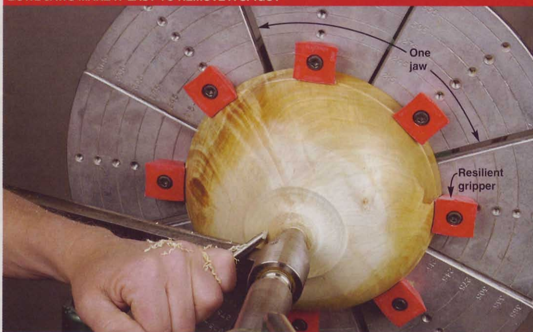
Although each manufacturer has a different name for this chuck accessory, adjustable bowl jaws all work the same. Resilient grippers hold the bowl rim to the chuck jaws. Sets cost from $50 to $140.
