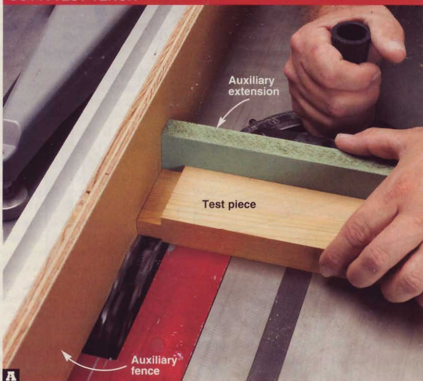
Keeping the end of your test piece tight against the auxiliary fence, crosscut both faces to form a ⅜" tenon ¾" long.
