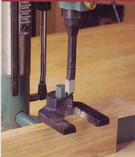
GOOD: Bridgewood's stock hold-down requires a hex wrench to secure it. And its 1 1/8"-high fence provides average support.
