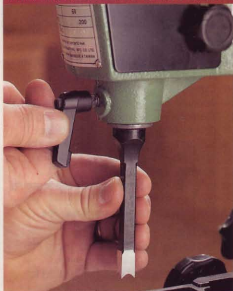
General International's handy ratcheting lock secures the chisel. The rest of the mortisers require a wrench or screwdriver.
