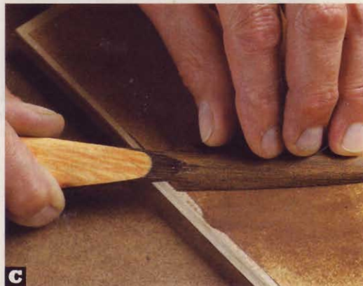
C Adhere 100-grit sandpaper to a piece of plywood, and chamfer both blade edges.
