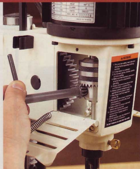
Jet's long chuck key and wide-open access to the drill chuck (left) make it easy to secure bits. By contrast, Bridgewood's chuck (right) can only be operated from the right or front of the machine, and the handle of the chuck key hits the cover knob.
