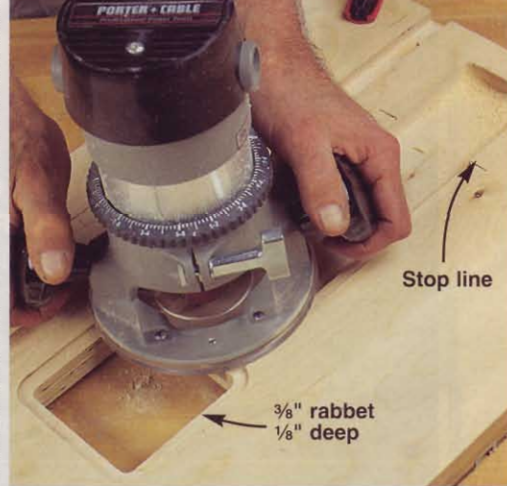
Rout a ⅜" rabbet ⅛" deep along the edges of the 3½×3½" cutout and the edges of the 2½"-wide channel, stopping 3" from its end.
