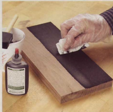
To re-create the look of ebony, brush on black aniline dye. Flood the surface, and then wipe away the excess to reveal the grain. Apply multiple coats if necessary.
