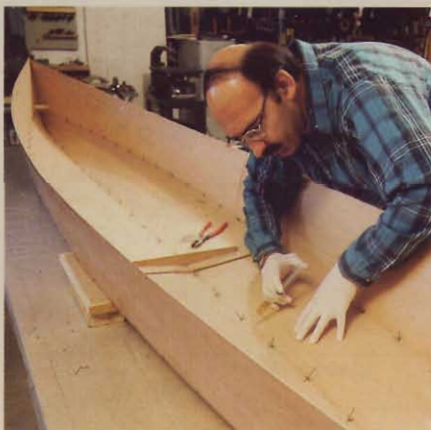
Waterproof epoxy works well above and below water. Boatbuilders use it because of its durability and gap-filling quality.
