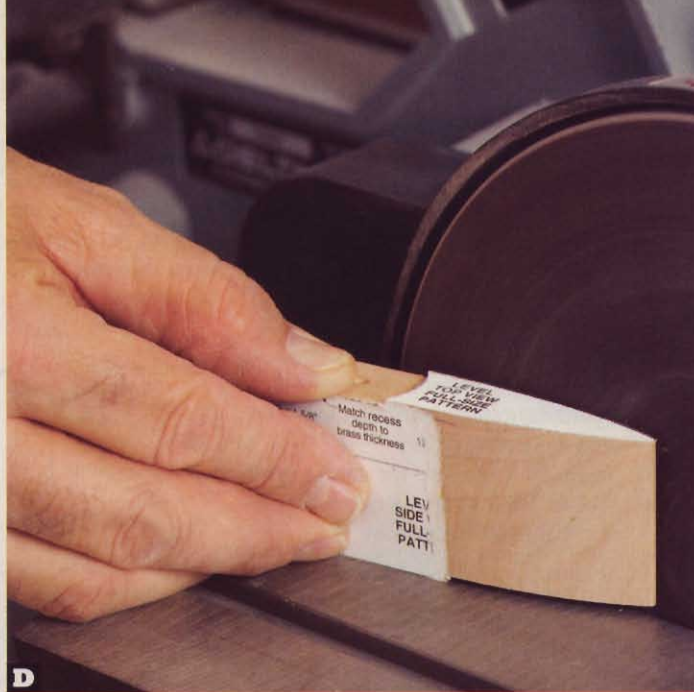
SAND THE LEVEL'S TAPERED ENDS
