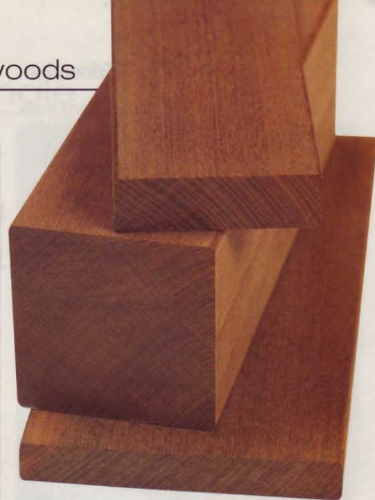
Retailers commonly stock 1x4, 1x6, and 4x4 ipé stock. Some also carry 2x2 and 2x4 stock for deck railings.
