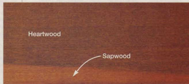
Ipé sapwood carries a white to tan color and proves less resistant to decay than the darker heartwood.
