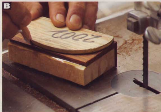
Templates guide freehand cutting at the bandsaw to give the head rough shape. Russ then sands the head to its final profile.
