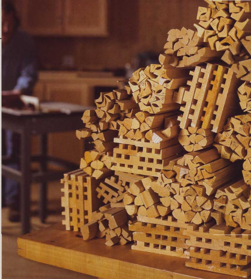
These bundles of 4'-long workpieces represent a mere fraction of the oak and MDF we machined to learn what separates premium- and low-cost router bits.
