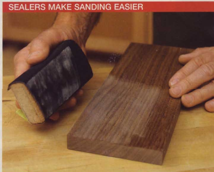
We brushed lacquer-based sanding sealer onto this walnut sample board and let it dry. Light sanding produced a powdery residue that didn't clog the 320-grit sandpaper.
