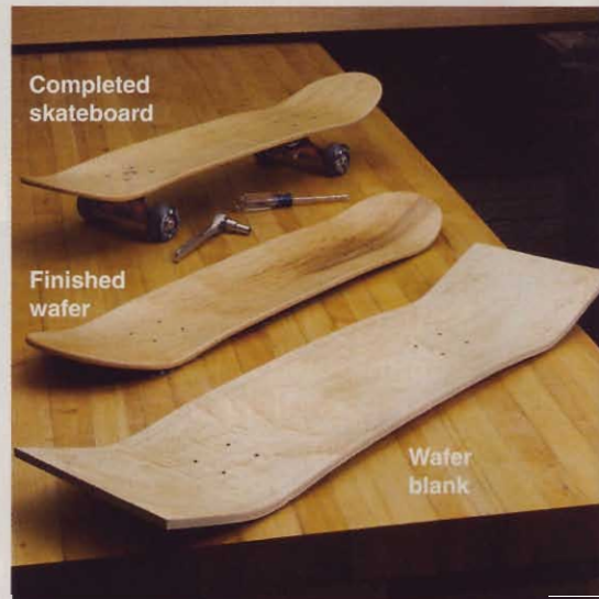
To make a skateboard from the kit, cut the wafer blank to size. Next, sand to the cutline and round over the edges with rasps, files, and sandpaper. Apply finish (center). Then add the wheels to the trucks, and secure them to the wafer using the factory-drilled holes and fasteners.
