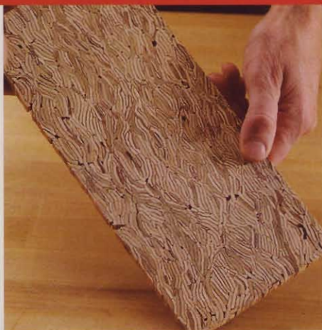
Crosscut Parallam to expose a pattern unlike anything else in woodworking. The voids you see here are holes that require filling.
