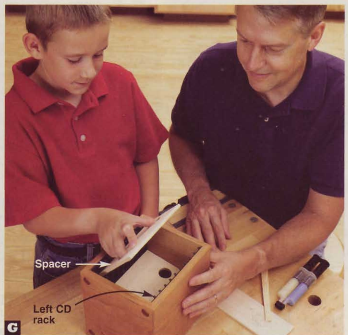
G Insert two spacers in the case, one at the back and the other at the front, to wedge the epoxied CD racks against the sides.
