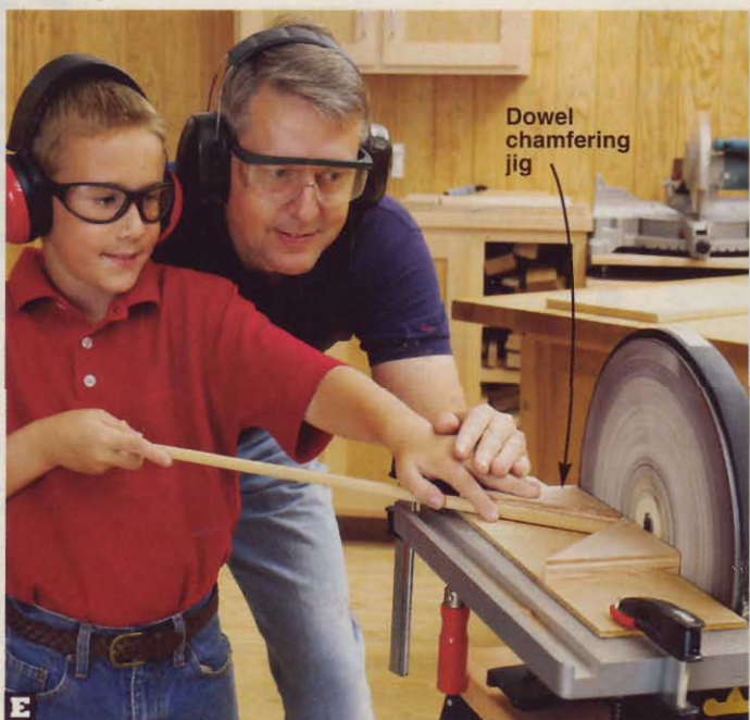
E Holding the dowel flat on the jig's base and tight against its angled stop, rotate the dowel 360° to sand a 1/16" chamfer on its end.
