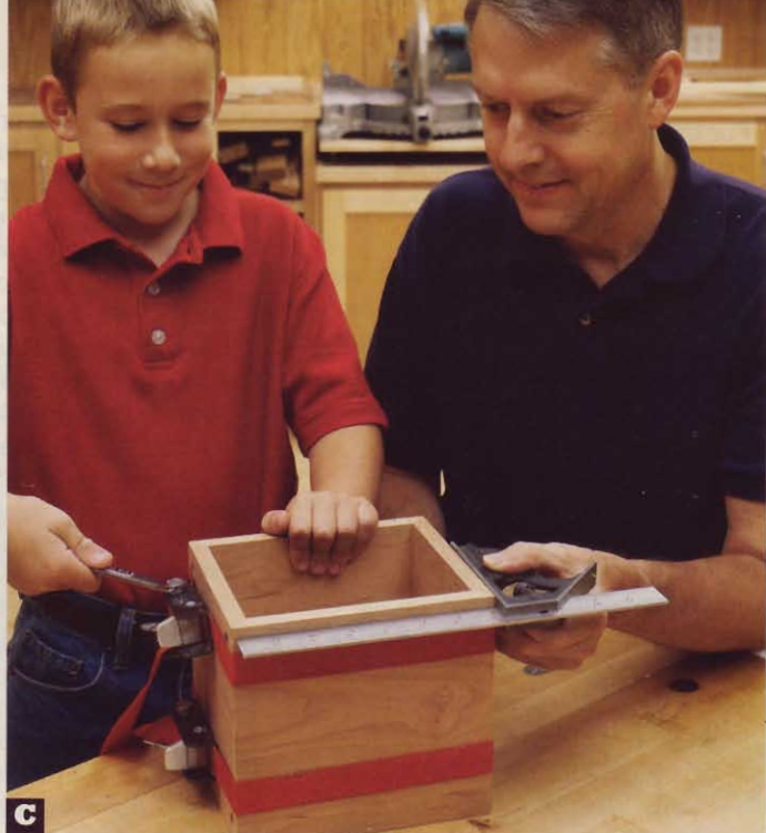
C While checking for square and verifying tight mitered corners, tighten two band clamps around the case to secure it.
