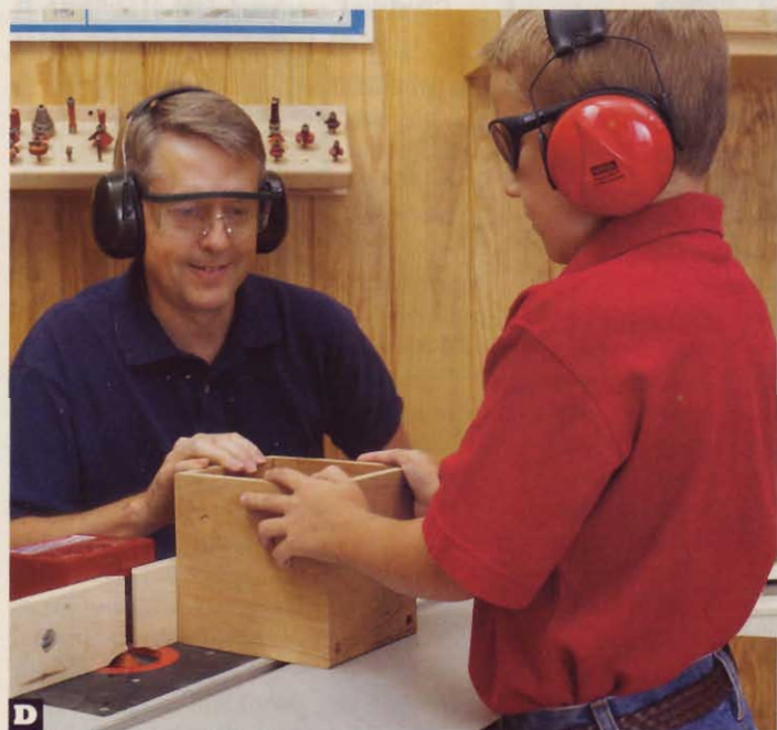
D Keeping the case assembly tight against the fence, move the assembly at a steady rate across the bit to chamfer the case edges.
