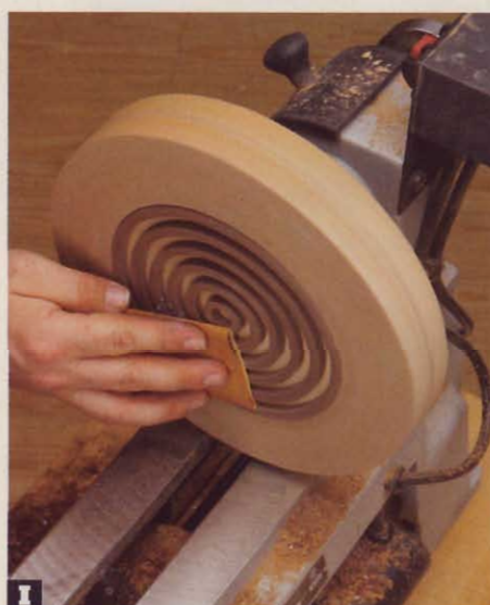
Tool: Parting tool Tool Rest: Center Speed: 800–1,200 rpm
