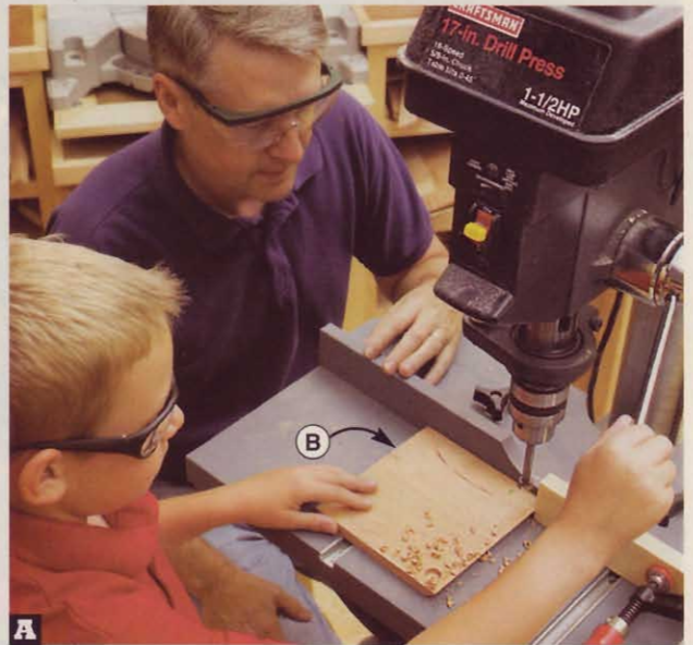
With the case bottom (B) held tight against the drill-press fence and stopblock, drill a ½" hole ¼" deep in each corner of the part.
