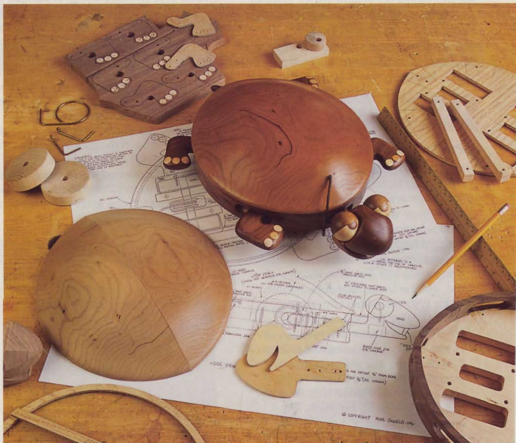
Mike Jagielo's projects all develop in the same way. After figuring out what he wants to build, he makes a full-size drawing, then templates, roughed-out pieces, and finally the finished product.
