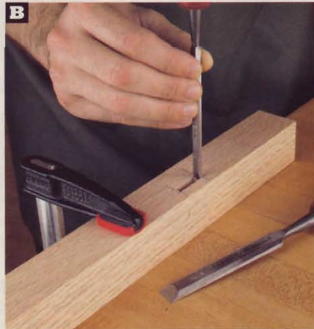
Using chisels held perpendicular to the leg's surfaces, square the mortises' ends and clean up their sides.
