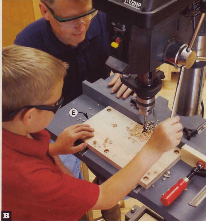
B With the stopblock positioned 5/8" from the bit's center, drill a hole in the base (E), rotate the part 180°, and drill another hole.
