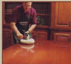
Refinishing - complete stripping and refinishing using an eco-friendly, water-based system
