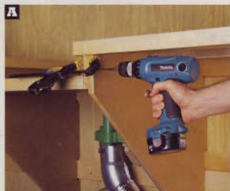
A Seat the platform supports against the underside of the tables, and secure the assembly with screws only. This allows you to move the platform should you ever switch saws.
