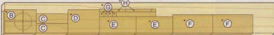
\frac{3}{4} \times 5\frac{1}{2} \times 48 " Cherry (2 bd. ft.) *Plane or resaw to the thicknesses listed in the Materials List.
