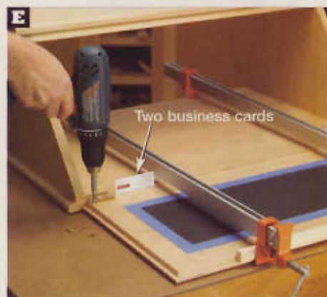
Inserting business card spacers, center the drop leaf on the desk case, and clamp it in place. Drill pilot holes into the drop leaf, and drive the hinge screws.
