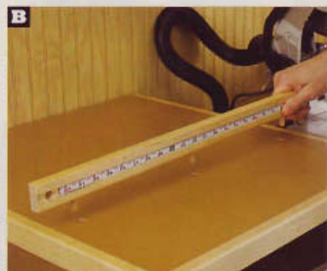
B Removable fences allow the tables to do double-duty as work surfaces. Slightly bevel the holes in the table using a countersink to make the dowels easier to slip into place.
