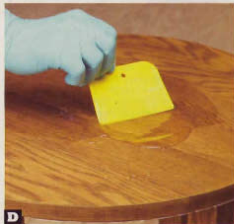
D Pour the epoxy mixture onto the surface, and spread it with your plastic spreader. After applying your first thin coat, wait 30 minutes, and then use this same tool to scrape off the excess. Pour the second coat up to ¼" thick, and again use the spreader to assist the self-leveling process.
