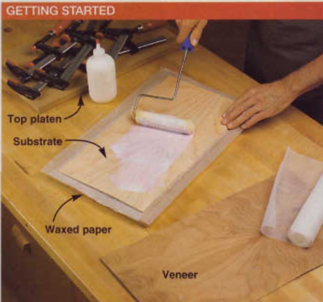
Place waxed paper on the bottom platen, and then the plywood substrate. Squeeze glue onto the substrate, using a foam roller to spread it evenly.
