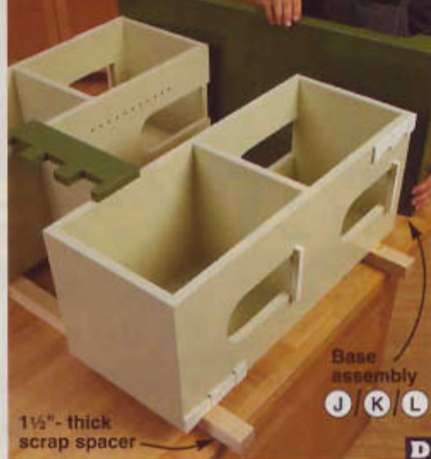
With the case assembly supported on 1 1/2"-thick spacers, center the base assembly (J/K/L) side-to-side on the case assembly's bottom, and fasten with screws.
