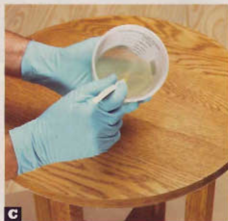
C Use a measuring spoon or small cup to measure out the resin and hardener into your mixing container, and then stir it steadily for two minutes with a stick. Scrape it off the sides as necessary, but don't mix vigorously enough to introduce air bubbles.
