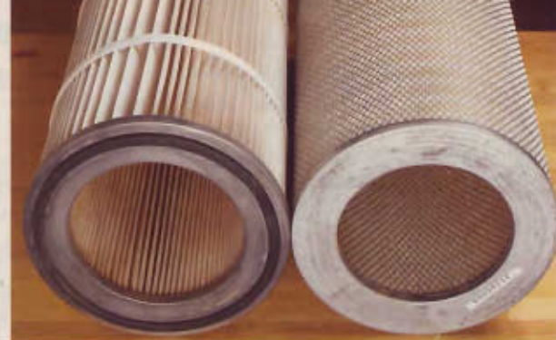
Pleated cartridge filters pack more filter surface area into a small package. Oneida's (left) cleans easily by blasting it with compressed air; Penn State's filter has five times the surface area, but its closely spaced pleats take more time to clean.
