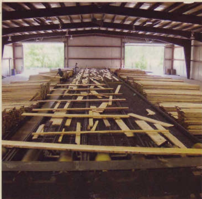
After leaving the grading and crosscutting station, the freshly milled boards fall back into human hands in the load-out area. As the boards travel down this long conveyor, workers inspect each one by hand, and then sort the boards according to grade and length. Finally, the boards get stacked to await drying.
