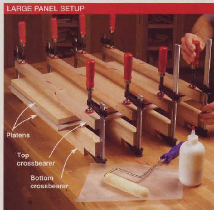
Space crossbearers 3" from each end and no more than 6" apart along the panel's length. To avoid confusion, mark "UP" on the edges of the top crossbearers opposite their tapers.
