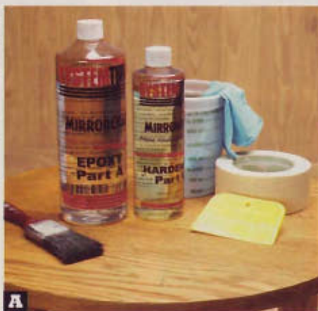
A Along with a two-part epoxy product, you need a mixing container; gloves; masking tape for the underside of the surface; a leveling tool, such as the plastic spreader shown here; and an inexpensive brush that you'll throw away after coating the edges.
