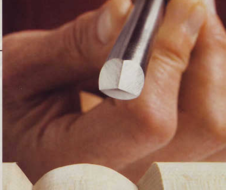
Three bevels and three sharp edges on the end of a 1/2" round shaft make a versatile tool you'll want to take for a spin.
