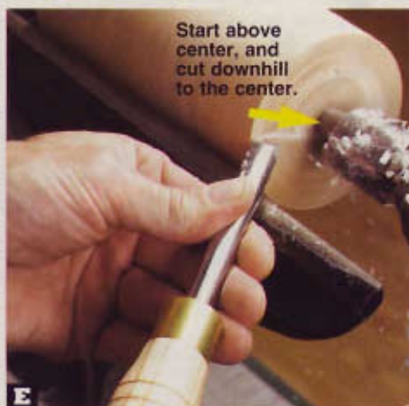
E To dress end grain, position the tool with one bevel up and tilted slightly toward the work surface. Engage the workpiece, advancing the tool from edge to center, using the whole cutting edge on flat surfaces and the middle of the cutting edge on convex surfaces.
