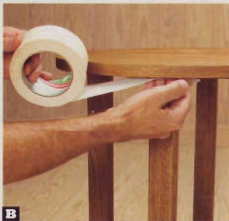
B Apply masking tape flush with the edge of the surface to be coated. We placed short strips all the way around the table, each one protruding slightly, and then trimmed them with scissors. After you pour the epoxy, allow it to set up, and then peel away the tape. Any epoxy "stalactites" will come with it.
