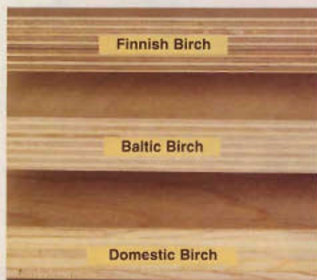
Finnish or Baltic birch \frac{3}{4} " plywood has 13 plies, compared to seven (five core plies plus face and back veneers) in domestic birch.
