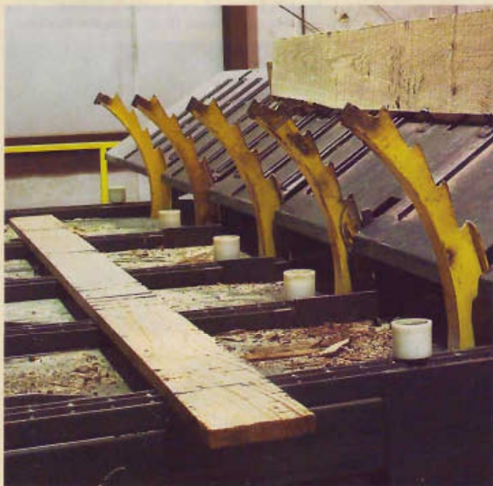
The lumber grader looks down on this sloped platform, where he examines the appearance of one face of each board, then flips it and looks at the opposite face. At the same time, he checks the board's width, and sends the board to be automatically crosscut to final length and stamped with a grade mark.
