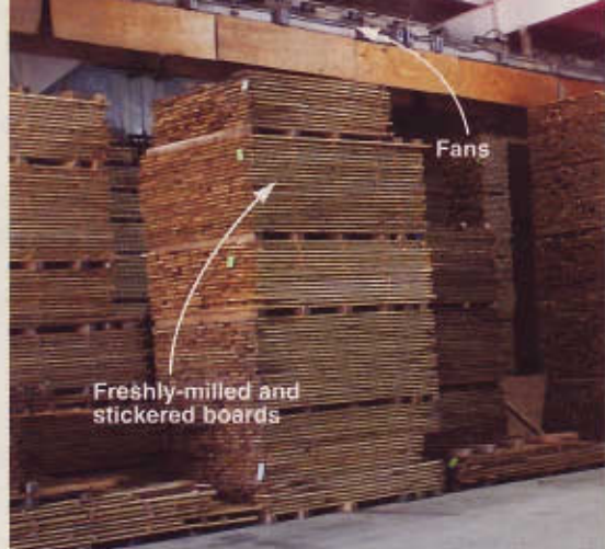
Large fans near the roof of the predryer circulate air through the 91 stickered boards. Baffles positioned between the stacks direct the airflow to ensure even drying.
