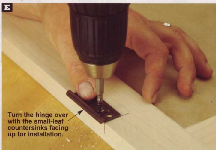
Turn each hinge over so its barrel and the countersunk holes in the small leaf face up. Fasten the hinge to the door stile using the screws supplied with the hinge.
