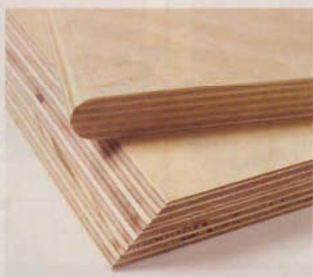
Good quality wood, fine glue lines, and void-free plies combine to make Baltic and Finnish birch plywood quite machinable.
