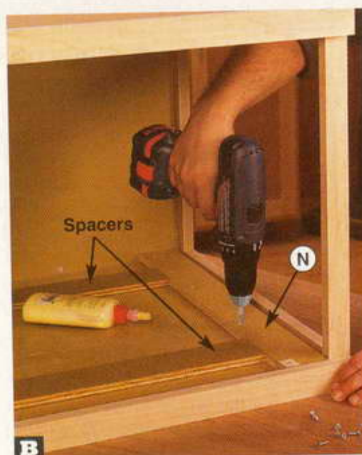
B With their ends against the cabinet's bottom, use a pair of 18"-long spacers to position the top cleats. Then glue and screw the cleats in place.
