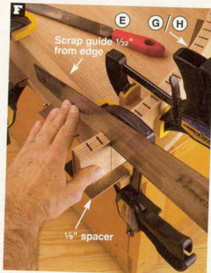
Clamp a \frac{3}{4} \times 3\frac{1}{2} \times 18 " scrap to the tabletop half, \frac{1}{32} " back from its straight edge and tight against the apron. Using the scrap as a saw guide, trim the apron's end.
