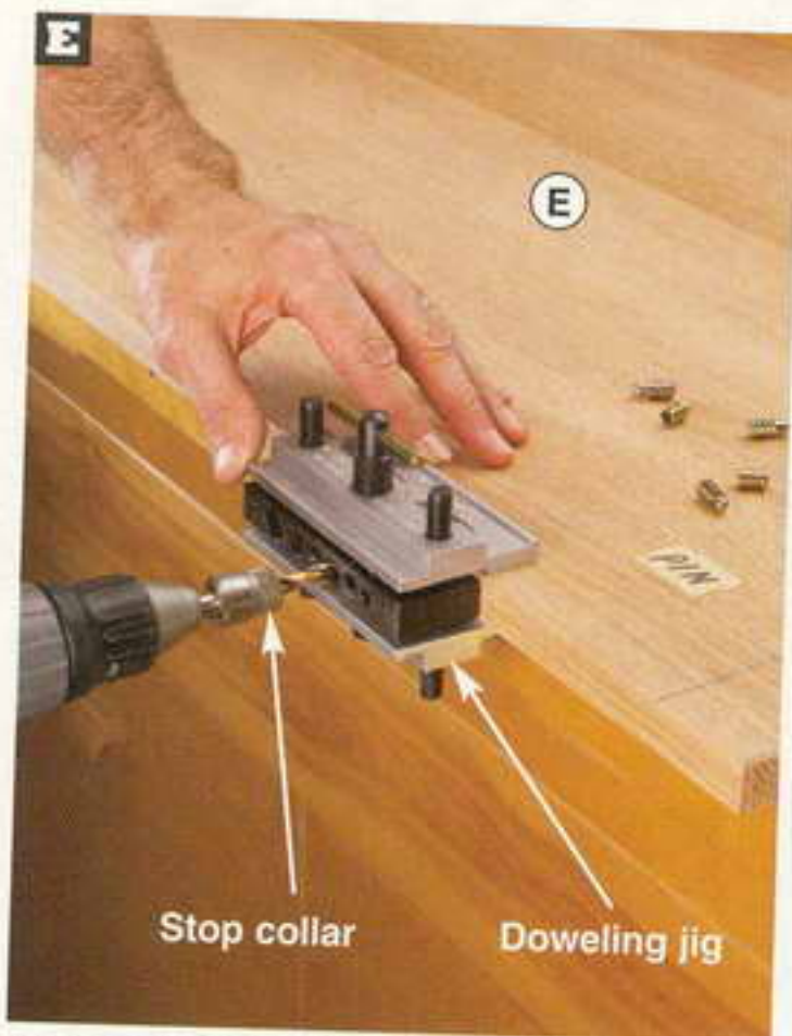
Align a doweling jig's \frac{5}{16} " guide hole with the marked line for a pin or sleeve. Adjust the jig to center the guide hole on the part's edge, and drill the hole.
