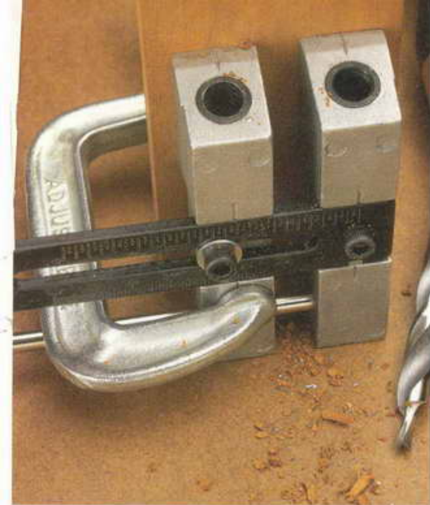
The guides on Rockler's 21296 didn't hold up well in our test. Even after boring more than 50 pocket holes, we still found steel shavings among the wood chips.
