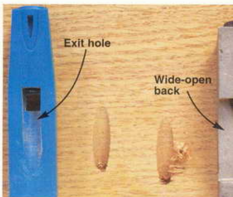
The close-fitting bit-exit hole of the Kreg Mini (left) prevents tear-out in cross-grain cuts better than the wide-open back of the Task Pro Center 06200 (right).
