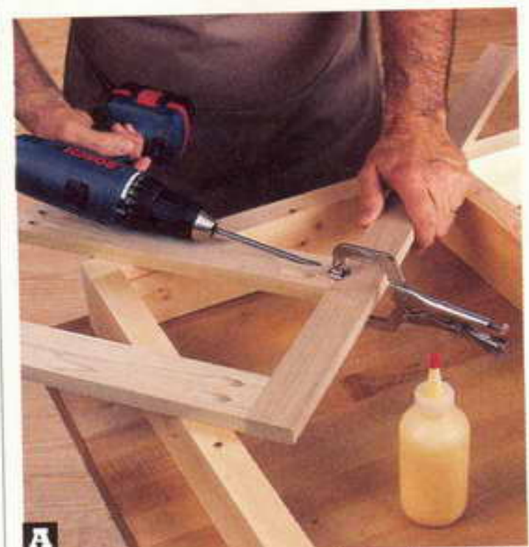
A A clamp, such as this specialized version, keeps the joint members flush while you drive the pocket-hole screws. Use 1 1/4" pocket-hole screws for 3/4" stock.
