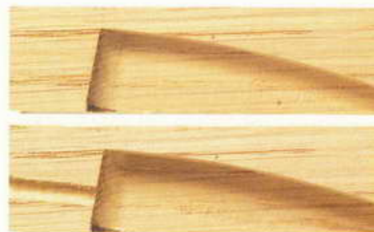
Porter-Cable's 552 swings a straight router bit up into the workpiece to create an arch-shaped pocket (top). Then, a drill bit plunges into the end to create the screw pilot hole (bottom).
