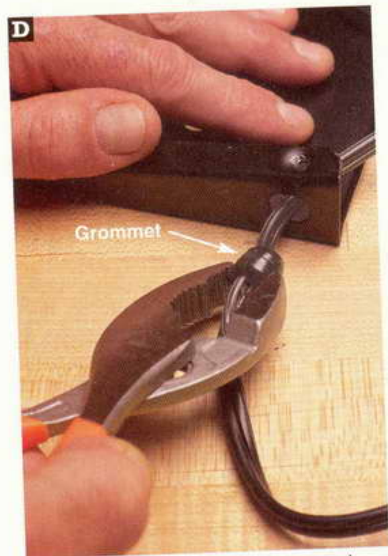
Grasp and squeeze the cord grommet with pliers to release the cord from the housing. Pull the cord out of the housing, and remove the grommet.
