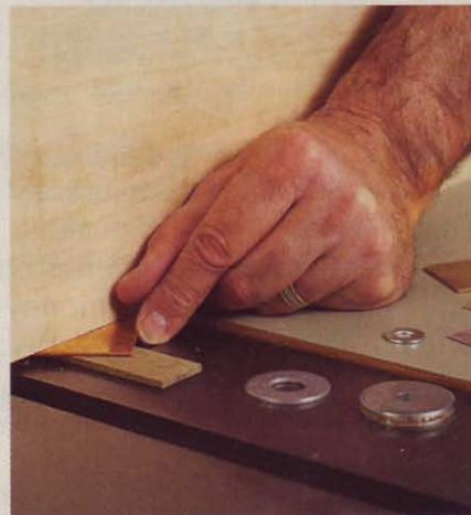
Find the right combination of shims to fill the gaps between the tool's table and straightedges at the locations over the mounting holes in the tool's base.
