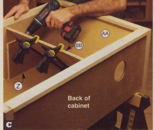
C Position the right baffle (BB) on the supports (Z). Clamp it to the left baffle (AA), and screw it to the supports.
