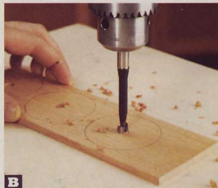
B Using a 3/8" Forstner bit, drill a 1/8"-deep counterbore in the center of each foot (C) on the workpiece.
