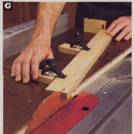
The width and adjustability of the taper jig allow you to handle a wide range of angle cuts. Here, with the jig flipped end-for-end, we're shaping a simple leg.
