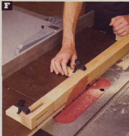
Hold the taper jig tightly against the table-saw rip fence as you cut. Before starting each pass, make certain that your left hand is well away from the line.
