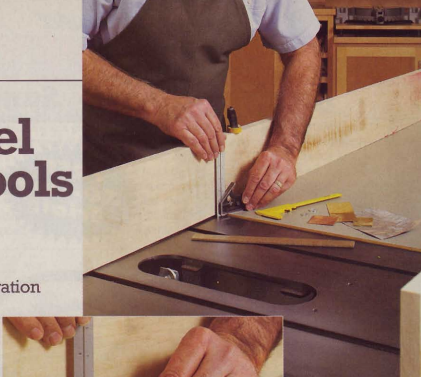
Use an adjustable square or calipers to measure the tables' offset and gaps under the straightedges.
