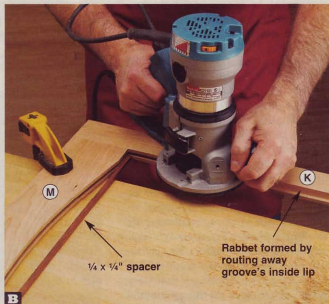
B When routing away the groove's inside lip, cut a 1/4 \times 1/4 inch spacer to friction-fit between the stiles (K). The bit's pilot bearing contacts the spacer, stopping the bit before it cuts into the upper rail (M).
