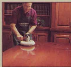
Refinishing - complete stripping and refinishing using an eco-friendly, water-based system
