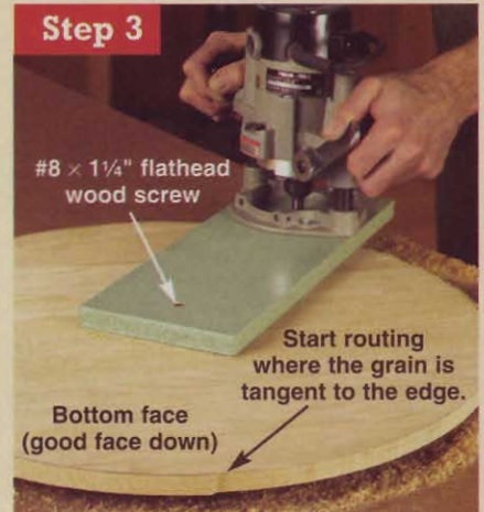
Step 3 Screw the trammel to the center of the bottom face of the top with a #8x \frac{1}{4} " flathead wood screw. Plunge the bit into the top's edge, and rout. Raise the bit before switching off the router. Start routing where the grain is tangent to the edge. Bottom face (good face down)
