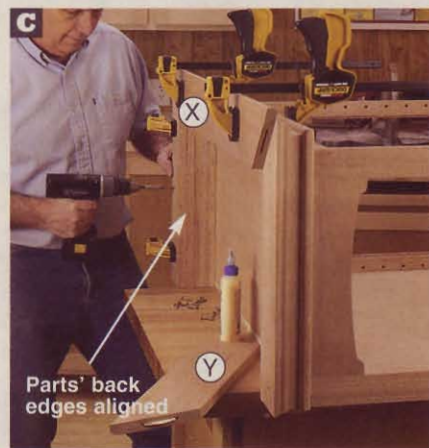
Align the back edges of the crown's parts as you assemble it. Offset each part's screw locations to avoid striking the screws below.
