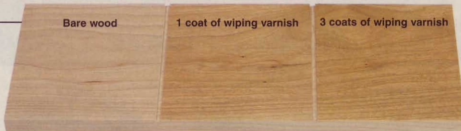
Applying the first coat of wipe-on finish brings wood to life, but don't be disappointed when it dries and goes flat. Adding another coat or two builds sheen and color.
