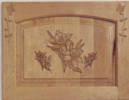
Laser engravings—both small and shallow, and large and deep—adorn this raised-panel door.
