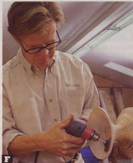
F Final sanding removes any ridges left by tools, and prepares the bowl for finishing.
