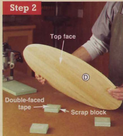
Step 2 To provide clearance for the router bit, stick three scrap blocks to your workbench with double-faced tape, then stick the top (D) to the blocks with more double-faced tape, top face down.
