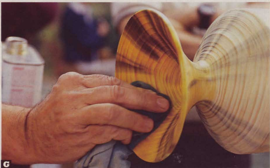
G Oil finish brings the almost-complete bowl to life, highlighting the contrast between dark and light, and adding an amber glow.
