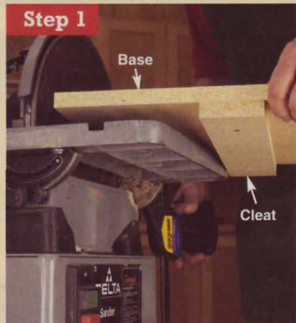
Step 1 Position the jig on your disc sander's table with the cleat contacting the table's right-hand corner, but about 2" away from its left-hand corner. With a single clamp, secure the jig's base to the table.
