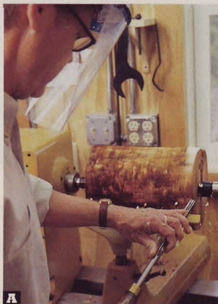
A With the lathe's speed at about 500 rpm and the tool rest about 2" below center-line, Macy trues the blank using a gouge.
