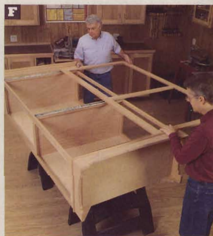
Using a helper, align the door's and cabinet's slides, and slide the door in place.
