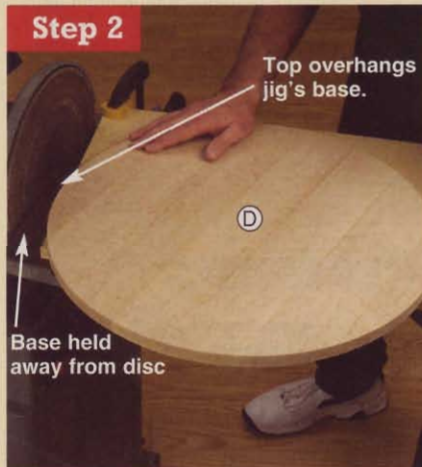
Step 2 Fasten the oversize bandsawn top (D) to the jig's base with a #8x1 1/4" flathead wood screw. The top overhangs the edge of the base that faces the sanding disc by about 1/4".
