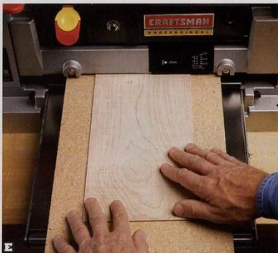
C To handle a significant snipe problem, run boards end to end through your planer. Place sacrificial scrap stock at the beginning and end of the line of boards.
