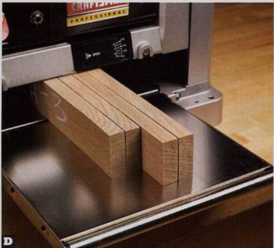
B Protect short pieces of exotic or figured wood, such as this purpleheart, by taking the time to glue strips to both edges. Rip them away after you finish planing.
