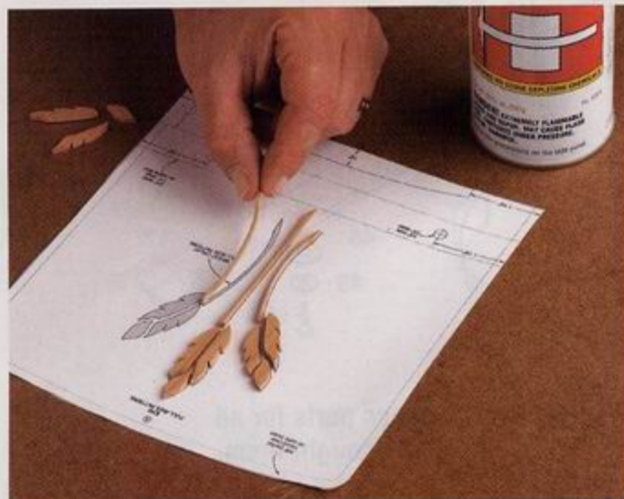
Spray the wheat onlay pattern of each end pattern with adhesive. Align and press the onlay pieces to the pattern.
