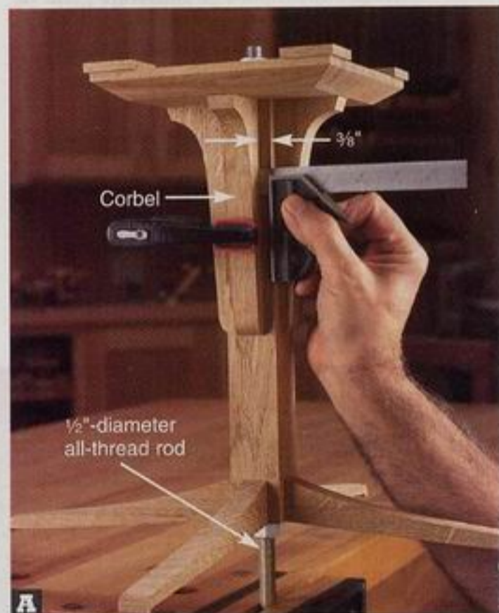
A Use an adjustable square to center the corbels on the post. Check for an equal \frac{3}{8} " measurement from the face of the corbel to the edge of the post.
