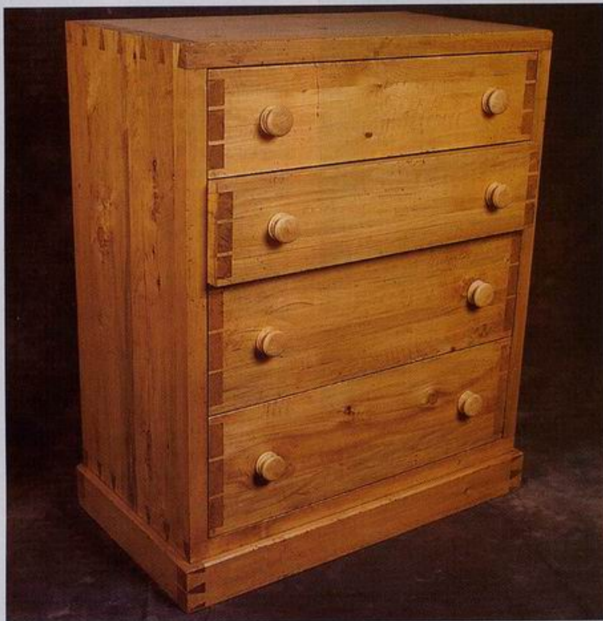
There's no need to guess what holds this four-drawer chest together. The massive dovetails lend a hand-tooled look that harken back the days of limited resources.
