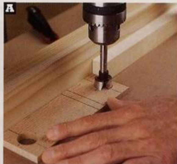
Guided by the drill-press fence and a stopblock, bore 1" holes in the blanks for parts H and I, and J and K.
