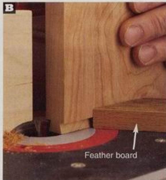
Use a feather board when forming dovetail tenons; its pressure ensures a smooth, straight cut for a snug joint.
