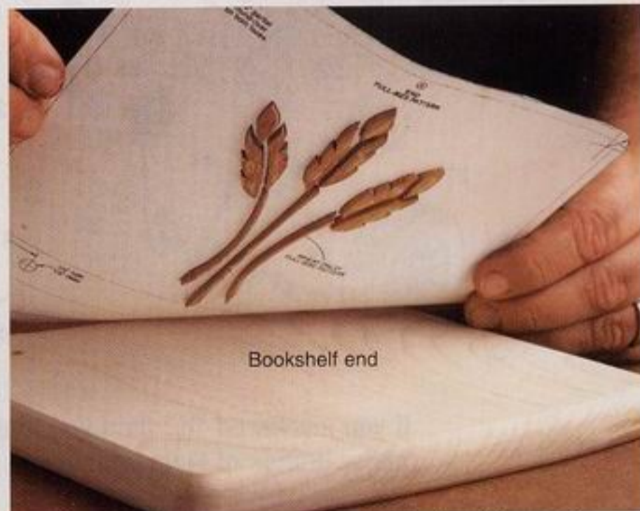
Align the end pattern with the bookshelf end, and press the glue-coated onlays in place.
