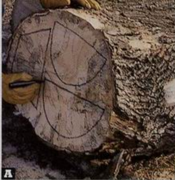
A After you find a spalted log, plan how best to use it. In Photo A, we marked three bowl blanks, being certain to avoid the unstable pith. After sawing into the end of the log to free those pieces, we cut them closer to finished shape, as shown in Photo B.
