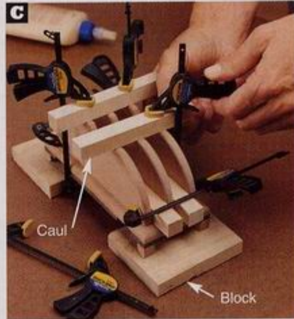
Raise assembly A/B/C/F on blocks for clamp clearance. Use scrapwood cauls to apply firm, even pressure to the dividers.
