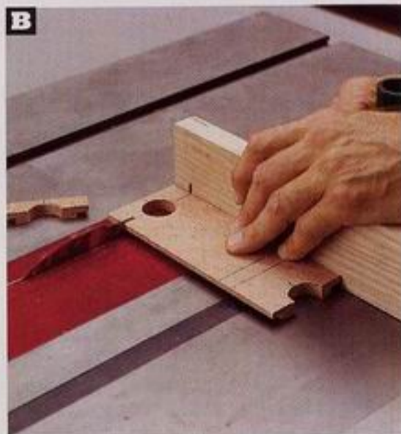
Form the semicircles by cutting through the 1" holes at the ends of the blanks for parts H and I, and J and K.
