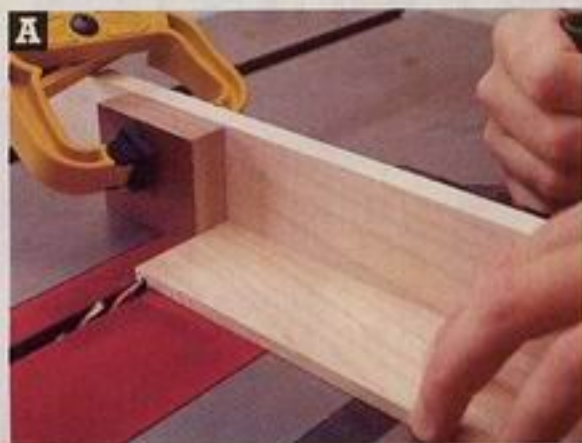
A A notched miter-gauge extension eliminates chip-out, and simplifies setting the stopblock to make identical cuts.
