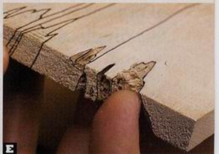
E Even though the board is usable, this very soft spot should be cut away to avoid milling and finishing problems.
