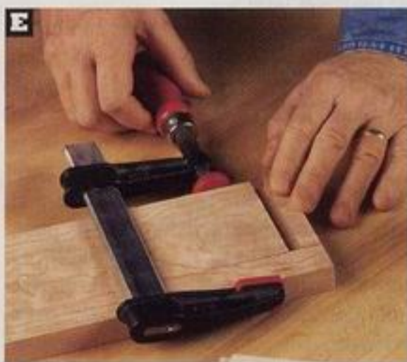
Keep the faces aligned perfectly when you reassemble the pieces. You'll avoid lots of scraping and sanding.
