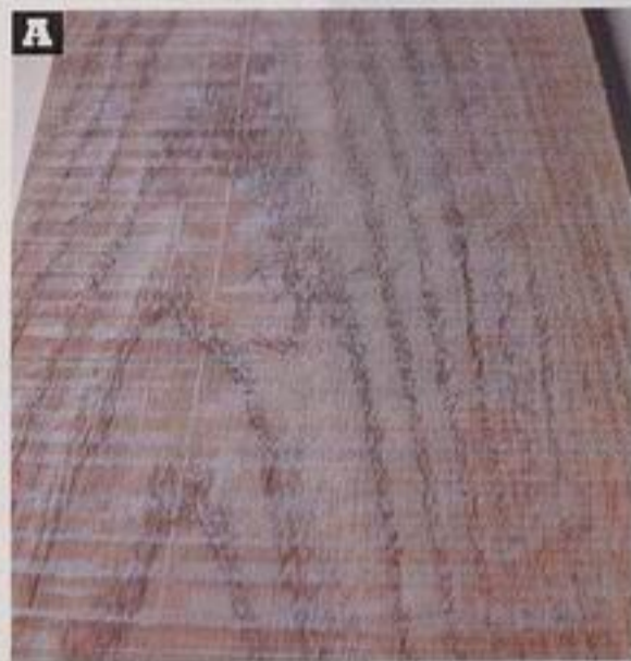
Blue chalk on these planed but unsanded boards shows where the Ryobi AP1300 cut inconsistently, leaving deep and wide cuts (indicated by an absence of chalk) between the high points (left photo). On the other hand, the board planed by the Delta 22-580 (right photo) shows few gaps in the chalked area, meaning a consistently smooth cut.
