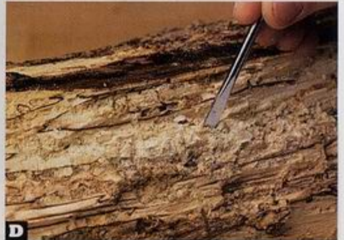
D Don't expect much from wood in this punky condition. Rather than try to save a flawed piece, search for better stock.
