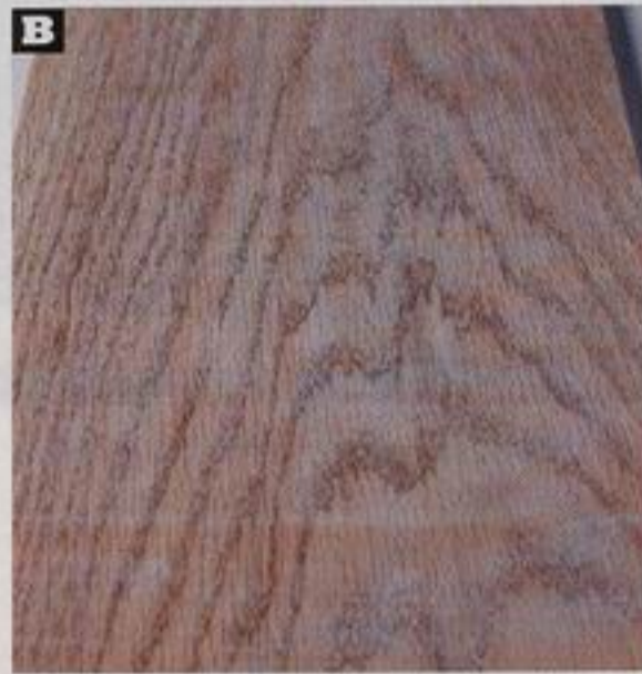
Blue chalk on these planed but unsanded boards shows where the Ryobi AP1300 cut inconsistently, leaving deep and wide cuts (indicated by an absence of chalk) between the high points (left photo). On the other hand, the board planed by the Delta 22-580 (right photo) shows few gaps in the chalked area, meaning a consistently smooth cut.
