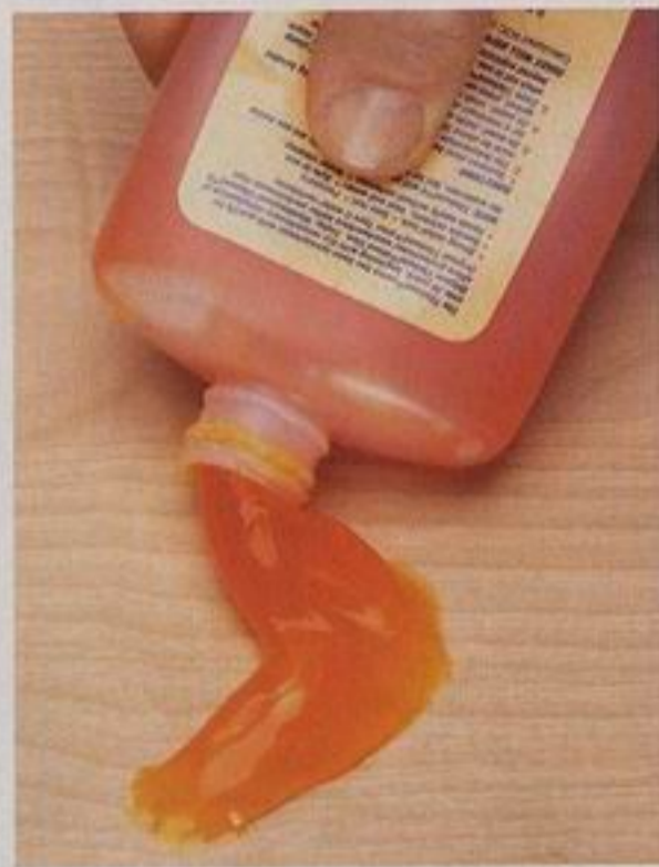
On the left is the code on a bottle of Titebond glue that was manufactured in July 2002. On the right you see the worst-case result of keeping yellow glue too long.
