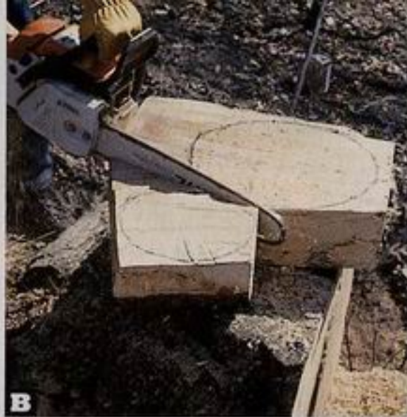
A After you find a spalted log, plan how best to use it. In Photo A, we marked three bowl blanks, being certain to avoid the unstable pith. After sawing into the end of the log to free those pieces, we cut them closer to finished shape, as shown in Photo B.
