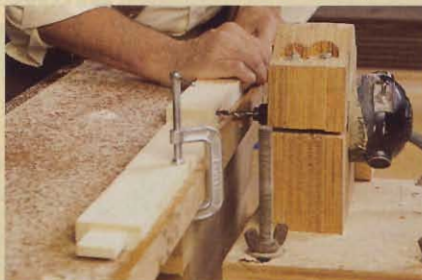
Step 1: With a horizontally mounted router, lay the workpiece on the table and ease it against a centered 1/4" straight bit. Use pencil marks and a stopblock to determine the start/stop locations of the mortise.
