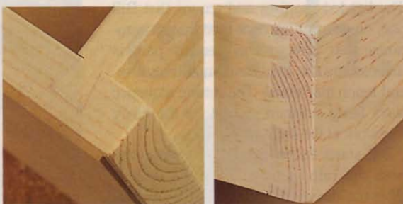
Two types of joints can be found in Bill's drawer-front construction: vertical sliding dovetails, left, and the more common half-blind dovetails, right.
