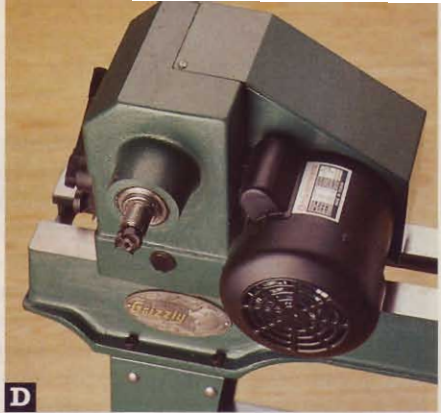
With the headstock in standard position, left, the distance to the lathe bed restricts turning diameter. Rotating the headstock outboard, right, allows you to turn larger pieces attached to a faceplate. (Grizzly model G1067Z shown.)
