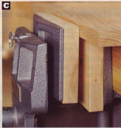
C Why have a pop-up dog when the entire jaw rises? You could clamp small panels with the Wilton 78A because of the wide, workpiece-friendly wooden surface.
