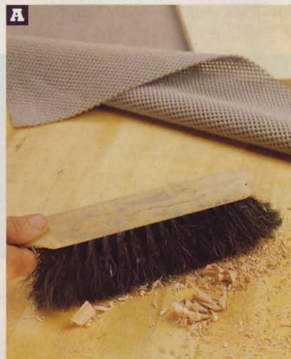
It's much easier to prevent dents and gouges in soft pine, rather than trying to fix them later. Before you start a project, take a minute to clean up your working surfaces. Then place a soft pad on the workbench to protect the wood.
