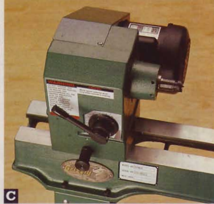
With the headstock in standard position, left, the distance to the lathe bed restricts turning diameter. Rotating the headstock outboard, right, allows you to turn larger pieces attached to a faceplate. (Grizzly model G1067Z shown.)
