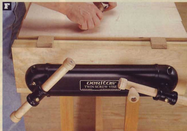
A twin-screw vise, such as this Veritas model, distributes pressure more evenly across its jaws than a single-screw vise.
