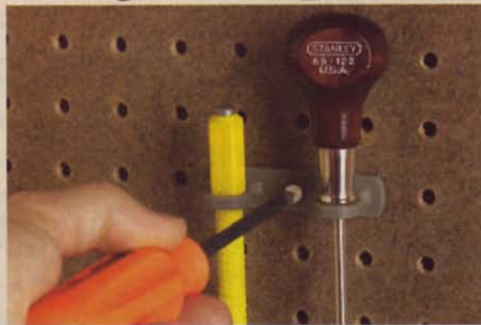
Locking hooks have a dual-purpose pin that you push in to lock the hook in place and unscrew to remove it.
