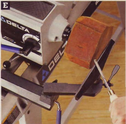
Included with some of the tested models, a simple extension positions the tool rest for outboard turning. (Delta 46-715 shown.)
