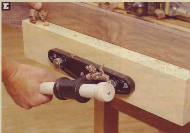
The wide jaws you make for a wooden-jaw vise provide excellent grip on long workpieces.
