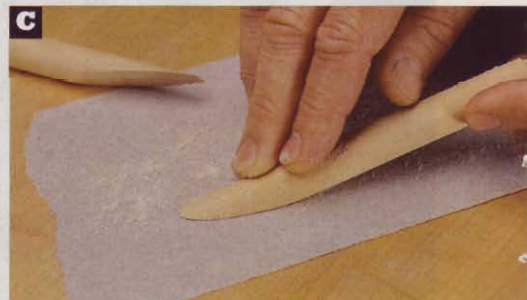
C Place self-adhesive sandpaper on a flat surface, such as your workbench, and carefully smooth the scarf joint.
