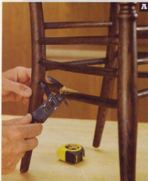
A Fixing a round stretcher rail isn't as difficult as it might look. Start by measuring the diameter and length of the piece.
