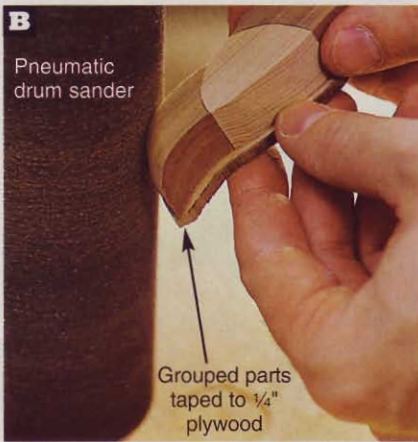
When contouring the parts, use light pressure and keep them moving to prevent burning the wood.
