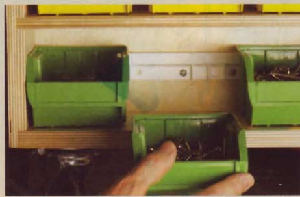
The support strip, which mounts to the cabinet back with #8x \frac{3}{8} " panhead screws, keeps the bins from sliding around when moving the cabinet.
