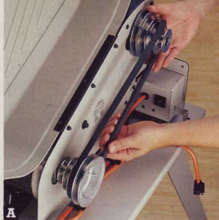
To change speeds on the Ridgid, left, and the Teknatool Nova (not shown), you stop the tool, and then move the belt on the stepped pulleys. The Craftsman, shown right, and the other tested lathes use shive pulleys. These pulleys expand and contract in diameter with just the turn of a knob or lever, increasing or decreasing the spindle speed.
