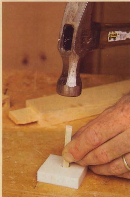
Bill rounds one end of a \frac{1}{4} \times \frac{1}{4} " square peg by tapping it into a Corian pad that has a countersunk recess machined into it. Doing this prevents the peg from splintering when he drives it.
