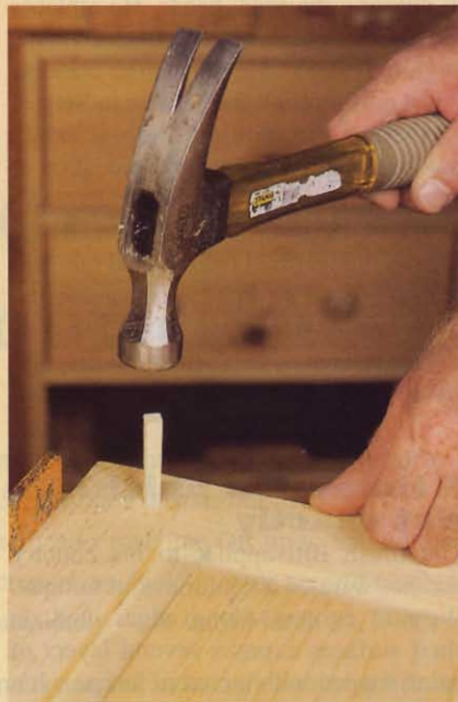
Finally, Bill drives the peg through the joint. As he does, the square corners grab the edges of the round hole, helping to anchor it in place. Excess wood is then cut and sanded off.
