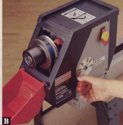
To change speeds on the Ridgid, left, and the Teknatool Nova (not shown), you stop the tool, and then move the belt on the stepped pulleys. The Craftsman, shown right, and the other tested lathes use shive pulleys. These pulleys expand and contract in diameter with just the turn of a knob or lever, increasing or decreasing the spindle speed.
