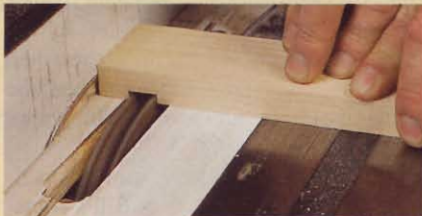
Step 2: Cut the tenon with a dado set, using both the miter gauge and fence to guide the stock.
