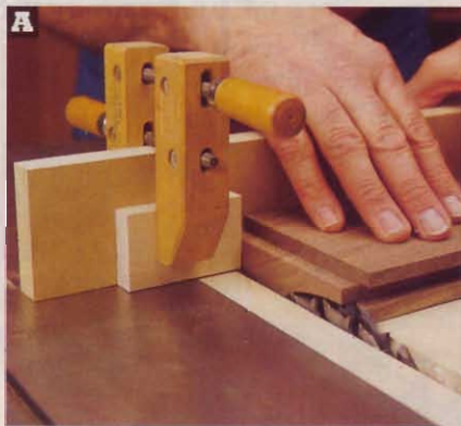
Cut the tenons on the rails and stiles using a stopblock, as shown, to ensure a consistent tenon length.
