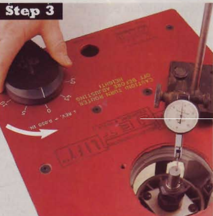
How we measured backlash: After calibrating the height of a gauge pin (in the router collet) to "0" on the fine-adjustment scale (Step 1), we raised the router at least one-half turn of the crank (Step 2). We then turned the crank back to "0" (Step 3), where the dial indicator shows the amount of backlash.
