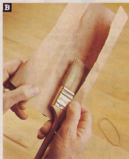
B Cut your paper long enough so you can fold it back to the ferrule without bending the bristles. Wrap it tightly, fold it, then hold it in place with a rubber band.
