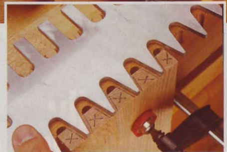
We were careful to mark the waste areas to make sure that we routed away the sockets, not the pins.
