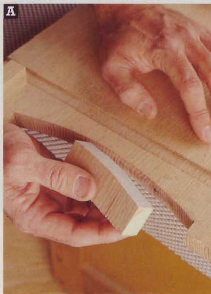
Make a custom sanding block by sticking adhesive-backed 120-grit sandpaper to a piece of the curve's waste.
