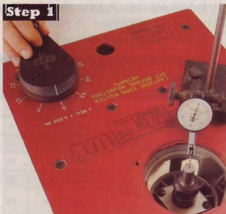
How we measured backlash: After calibrating the height of a gauge pin (in the router collet) to "0" on the fine-adjustment scale (Step 1), we raised the router at least one-half turn of the crank (Step 2). We then turned the crank back to "0" (Step 3), where the dial indicator shows the amount of backlash.
