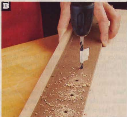
To drill uniformly spaced shelf support holes in the box long side panels, use a hole-drilling jig and a depth stop.
