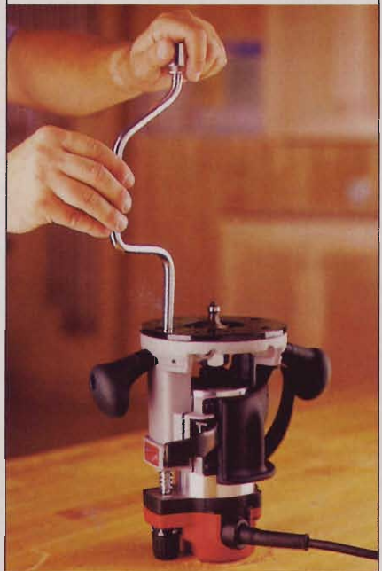
PRL's crank handle extends past the bit opening's center line and bumps the fence.
