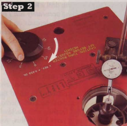
How we measured backlash: After calibrating the height of a gauge pin (in the router collet) to "0" on the fine-adjustment scale (Step 1), we raised the router at least one-half turn of the crank (Step 2). We then turned the crank back to "0" (Step 3), where the dial indicator shows the amount of backlash.
