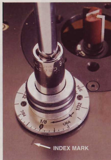
O-rings inside the Bench Dog fine-adjustment scale hold the socket shaft firmly, yet allow you to zero the scale to the index mark on the insert plate.
