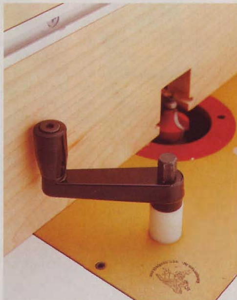
PRL's crank handle extends past the bit opening's center line and bumps the fence.
