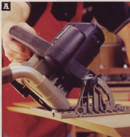
We bevel-cut thin strips of medium-density fiberboard to test each saw’s lower blade guard for hang-ups.
