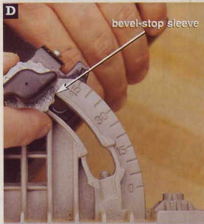
D Porter-Cable's bevel-stop sleeve rotates to open the bevel scale above 45° and below 0°. However, there are no markings to indicate whether the stop is in place or not.
