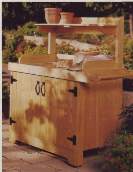
Baldcypress is weather resistant and easy to work with, making it a good choice for outdoor projects, such as this potting bench found in issue 140.
