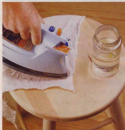
You can steam out small dents in wood with an ordinary household iron, but staining might leave a dark spot.
