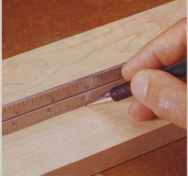
Measure by holding your rule on edge, and fit the pencil point into the incised line. This method eliminates the slight inaccuracy that can result from looking across the thickness of a rule lying flat on your workpiece.
