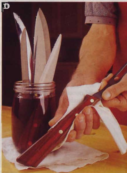
Soaking the handles lets the tung oil penetrate deeply, beautifying and protecting the wood.
