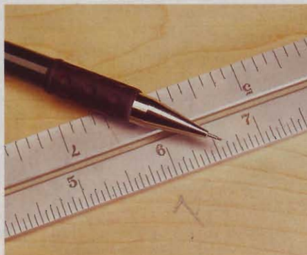
Make your mark with an arrow shape, like the one shown here. When you take the rule away, you'll still know the exact point that matched your measurement. The longer leg denotes the waste side of the cut to be made through this point.
