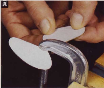
Twist each propeller blade, pushing down on the short lobe, and pulling up on the long one.
