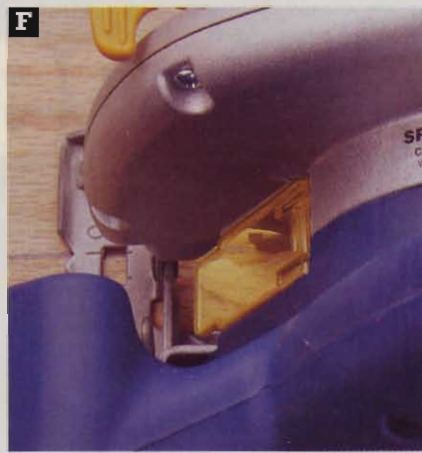
F Instead of an open space, Ryobi incorporates a dust-deflecting window for viewing the cutline. It remained surprisingly clear throughout our tests.
