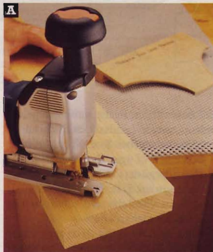
Use your jigsaw to cut the joist and girder ends to shape before smoothing the final profile with your router.
