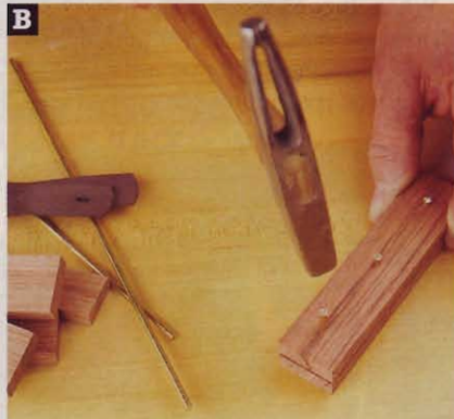
B The pins help hold the scales to the tang, and add decoration, with stainless rods arranged inside a brass tube.
