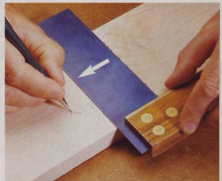
To draw a line after measuring a dimension, hold the pencil point on the tip of the arrow, then slide your square or rule until it contacts the pencil. This method ensures that your line will match the point. Now, pull the pencil along the square.
