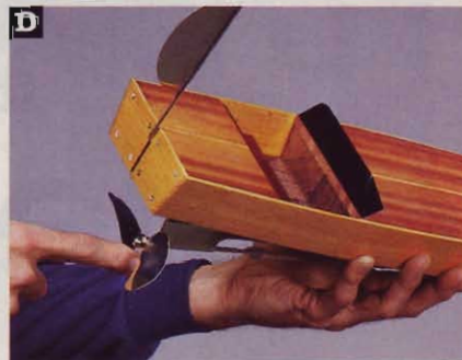
To wind the propeller, pull the rudder shaft out of the transom slot, and swing it out of the way.
