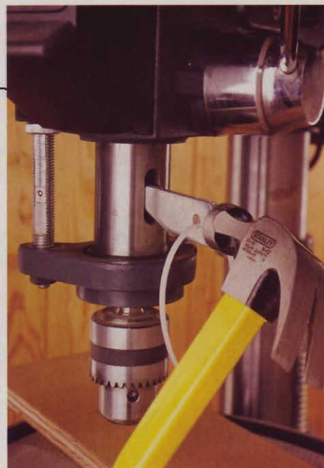
It doesn't take much force to drive the chuck out of your drill press with a wedge and a hammer.
